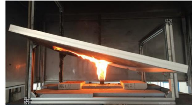
Foto: J. S. Kristensen, B. Merci, and G. Jomaas, 'Fire-induced reradiation underneath photovoltaic arrays on flat roofs', Fire and Materials, 2017.
