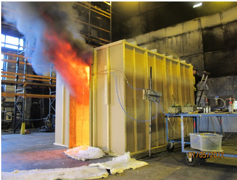
Figure 19. Photo of the room fire test 4. The heat release rate was 1.2 MW.
