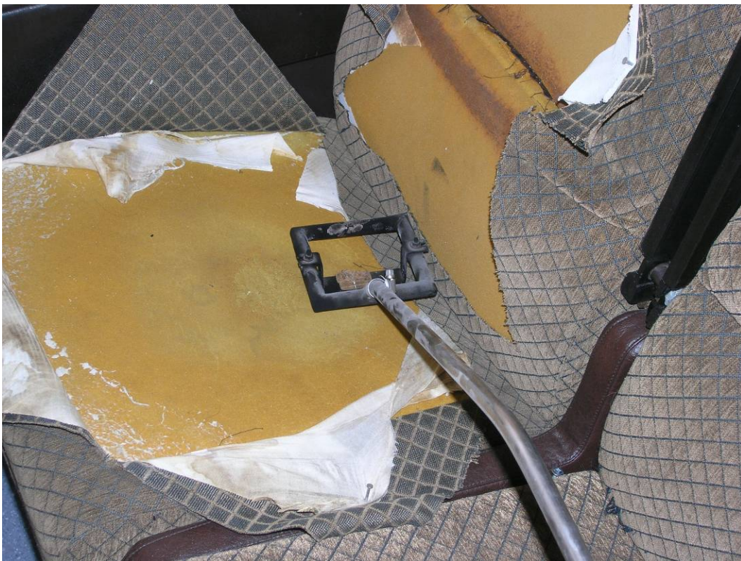
Figure 10 The square burner used for igniting the seat. Also notice the standardized vandalism of the seat [13].
