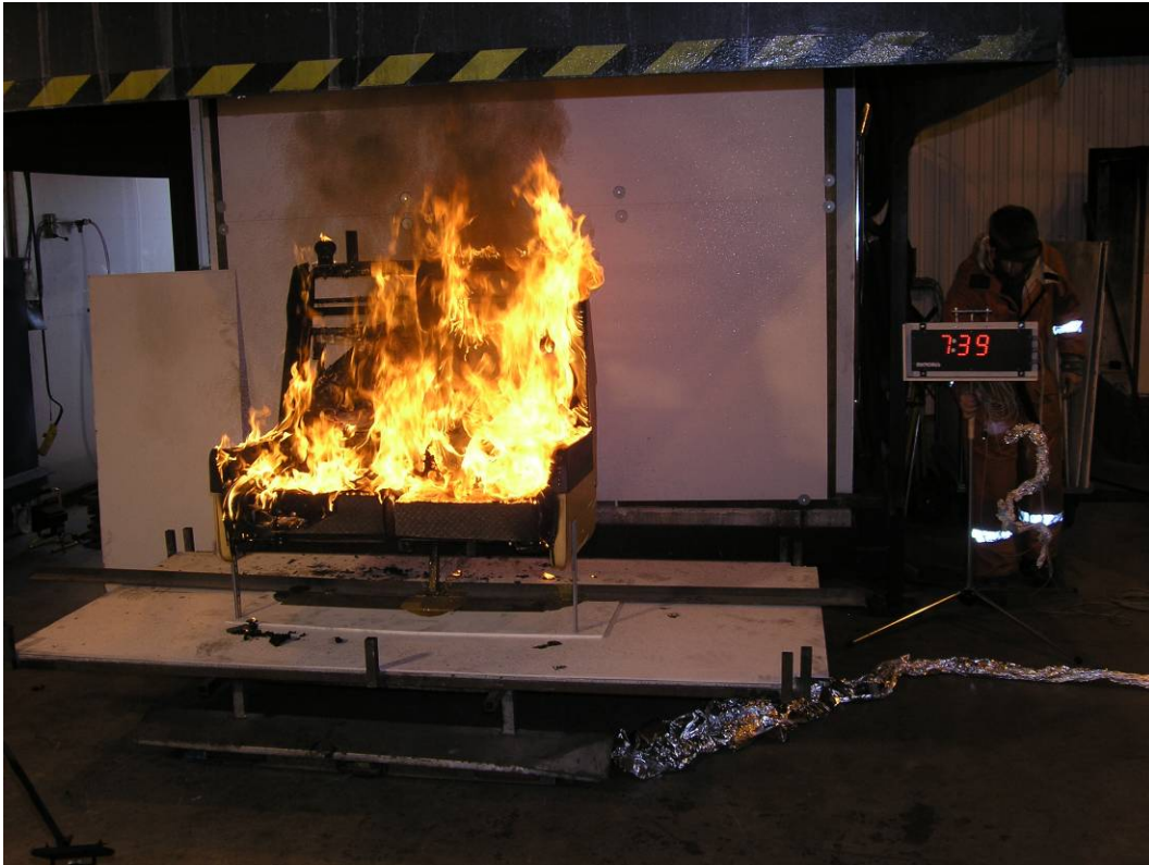
Figure 24 Free-burning seat in the furniture calorimeter, 7 min and 39 s after ignition.
