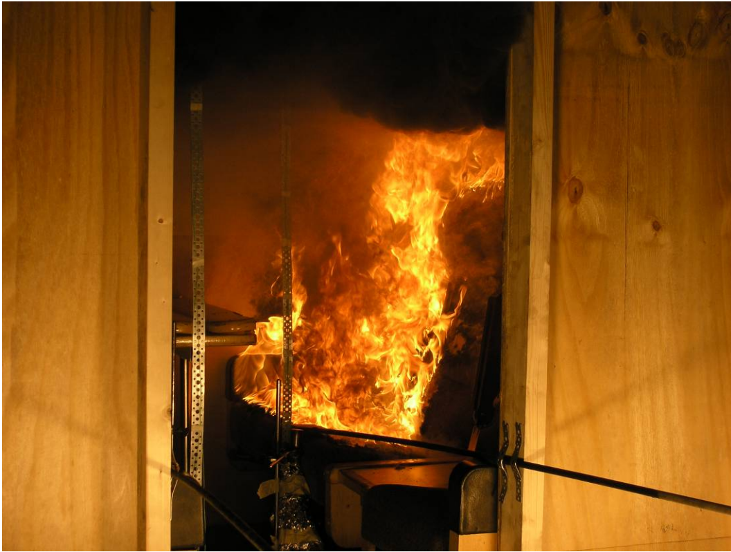
Figure 14 Fire development 132 s after ignition of the propane burner.
