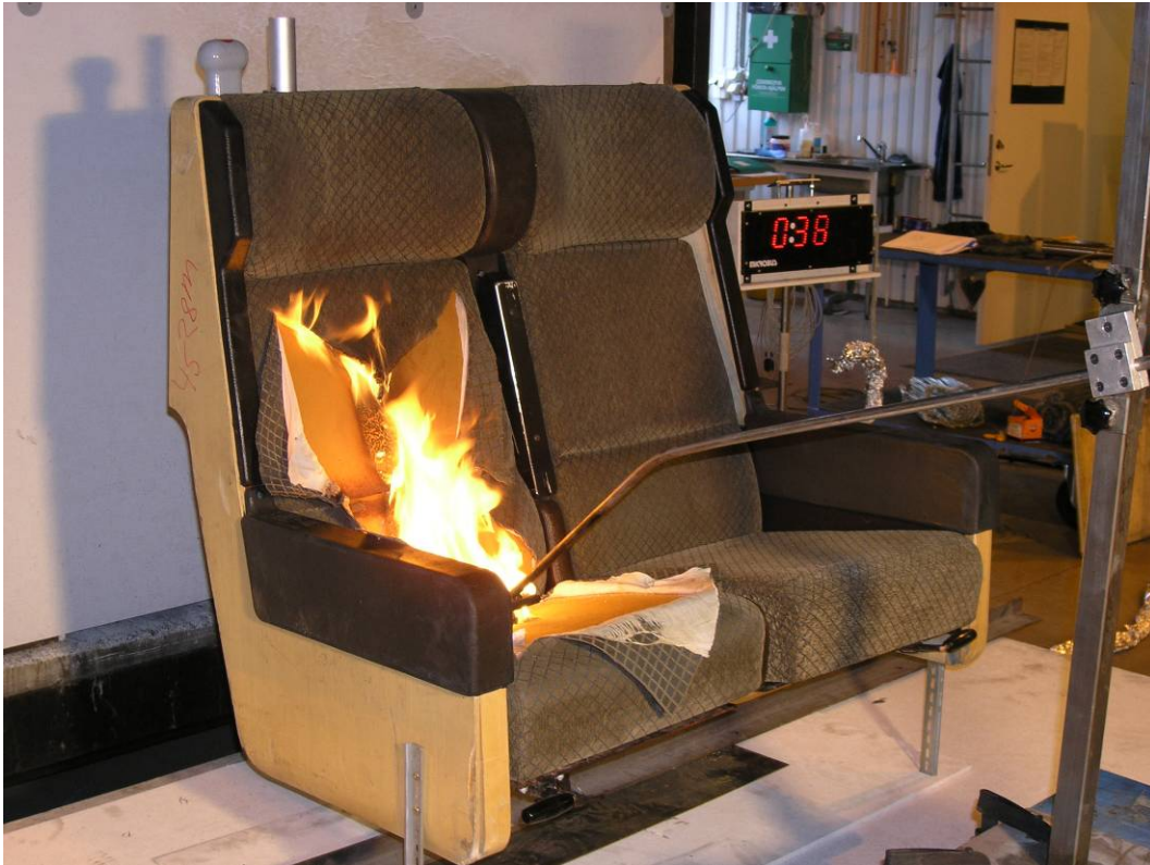
Figure 22 Free-burning seat in the furniture calorimeter 36 s after ignition with the 7 kW propane burner.
