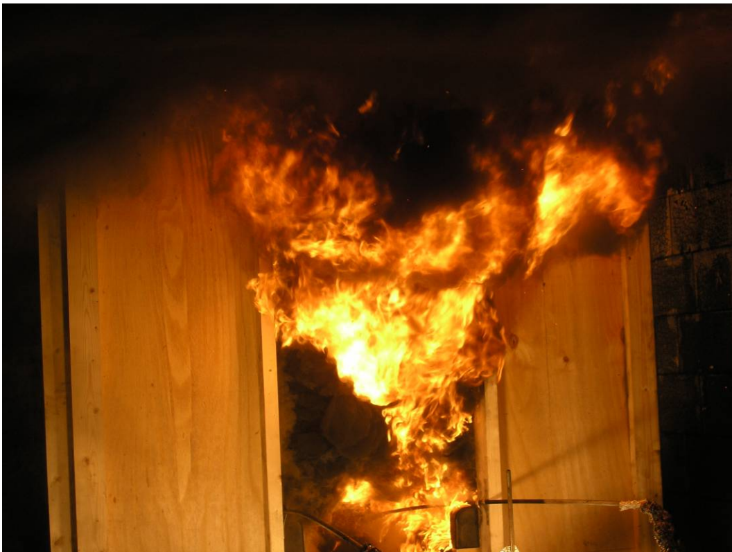
Figure 15 Fire development 208 s after ignition of the propane burner.
