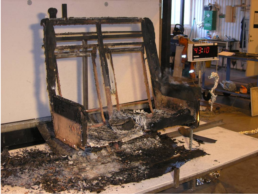
Figure 26 Combusted seat after test in the furniture calorimeter.
