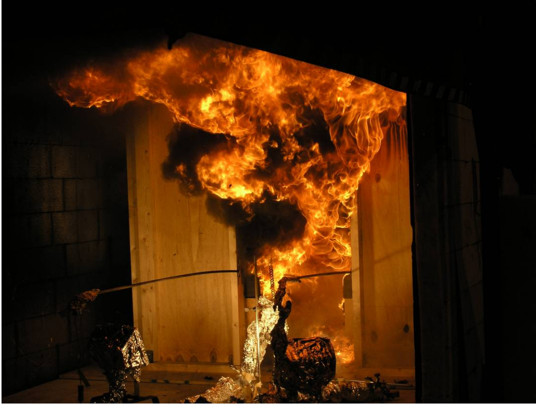
Figure 16 Fire development 218 s after ignition of the propane burner.
