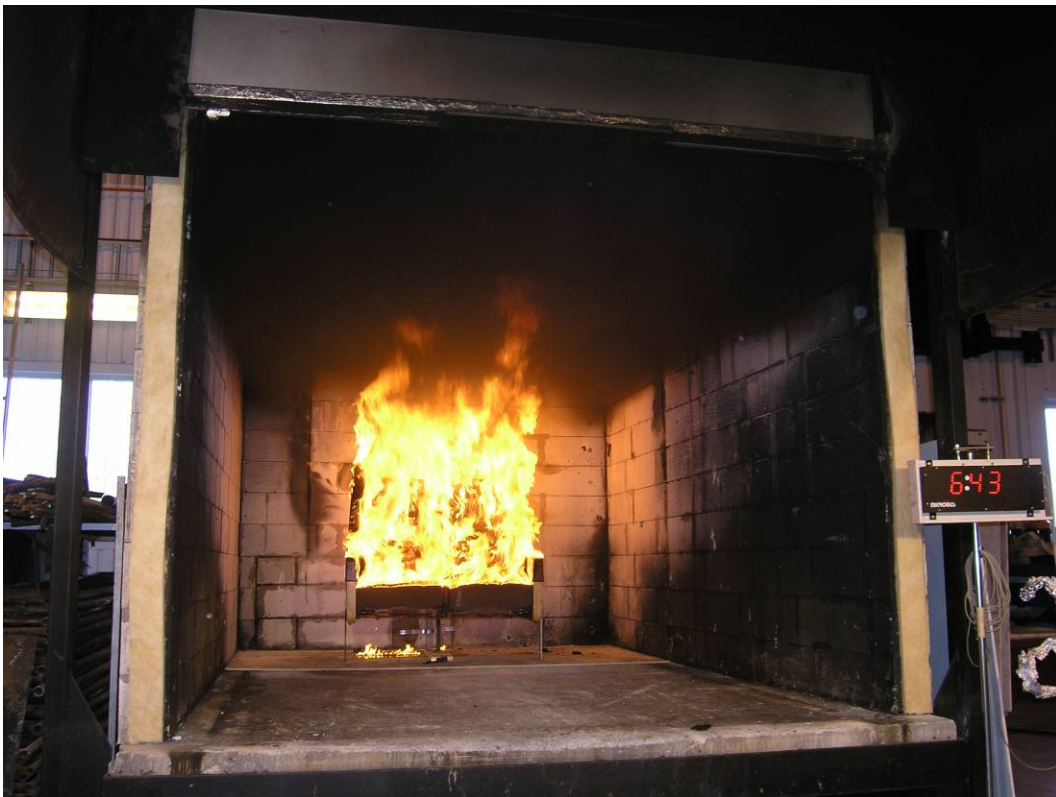
Figure 28 Burning seat in the ISO 9705 room, 6 min and 43 s after ignition.
