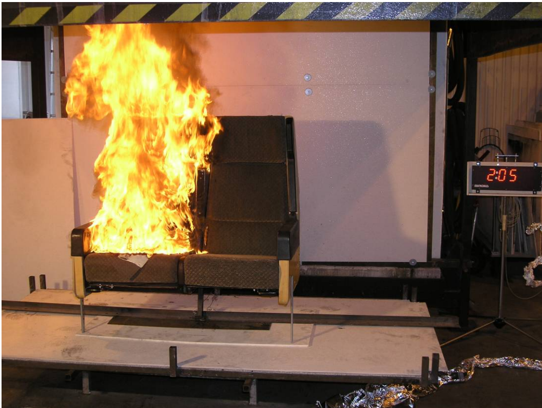
Figure 23 Free-burning seat in the furniture calorimeter, 125 s after ignition.
