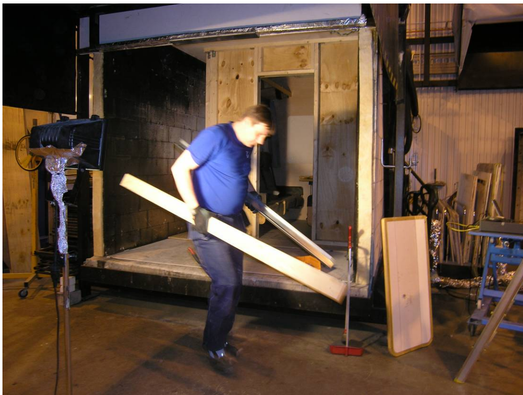
Figure 9 Photo illustrating how the train compartment was built in the inner right part of the modified ISO 9705 room.
