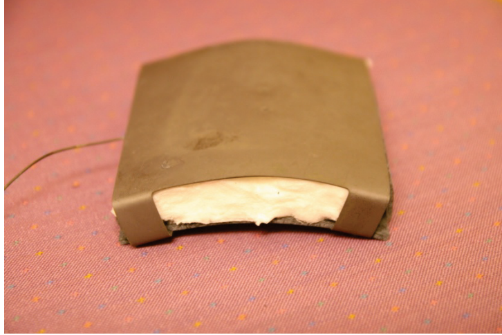
Figure A3 The specially designed plate thermometers that were embedded in the steel column flush with the surface.
