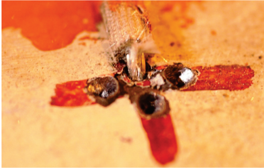
Figure A5 Quick tip with Cefir cable fixed in the steel structure.
