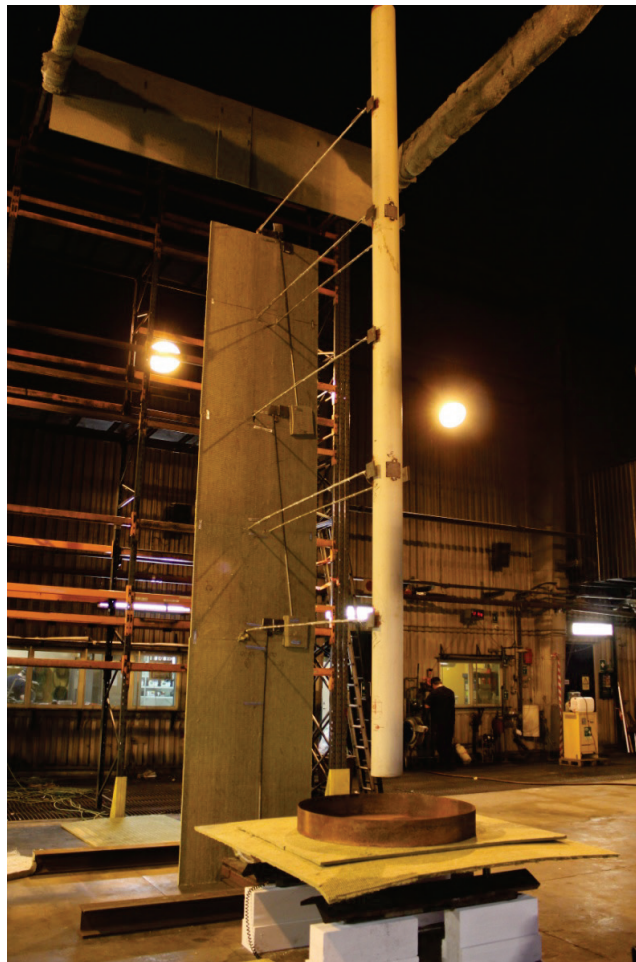
Figure 1 Experimental setup. Measurements were done at every metre along the column. Position 1 was in the left direction and position 2 was facing the mineral wool board.
