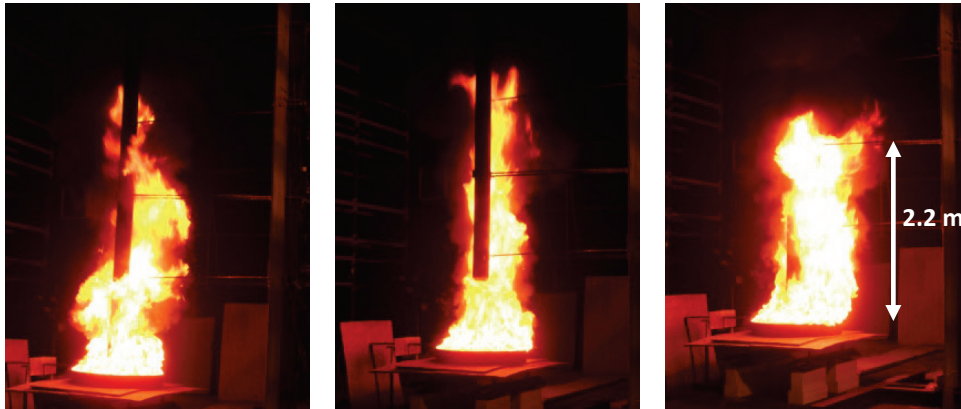
Figure 3. The flame from diesel \varnothing = 1.1 m. The flames are tilted towards position 1.
