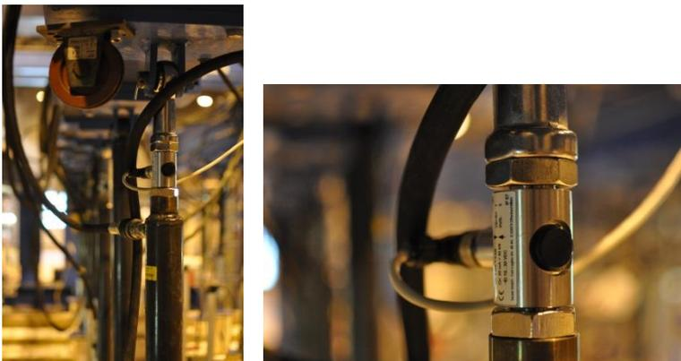
**Figure 3.15, load cell mounted on the actuator**
