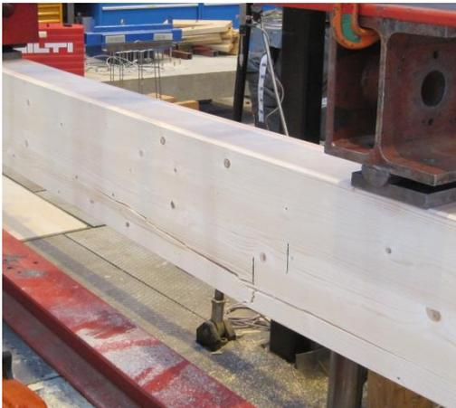
**Figure 2.4, failure of the lower lamella**
