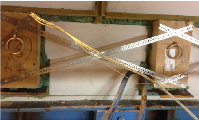
**Figure 3.5, cross-bracing of the ends of the timber beams**
