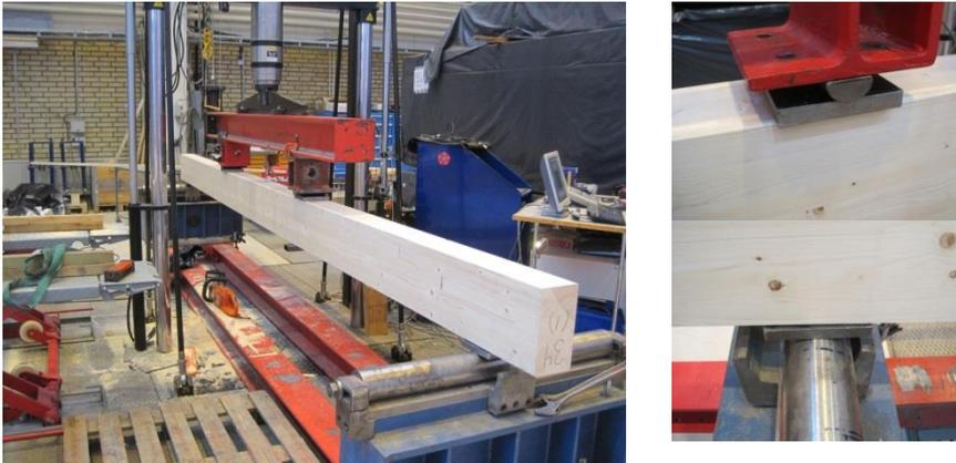
**Figure 2.3, measurement of bending strength and modulus of elasticity in 4-point bending**
