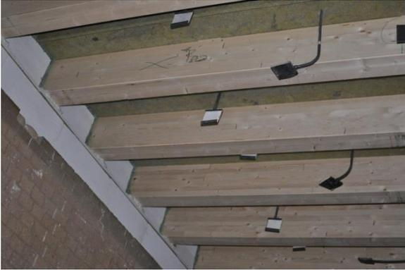
**Figure 3.8, view from inside the furnace showing the test specimens, plate thermometers and insulation of steel beam and roller supports.**
