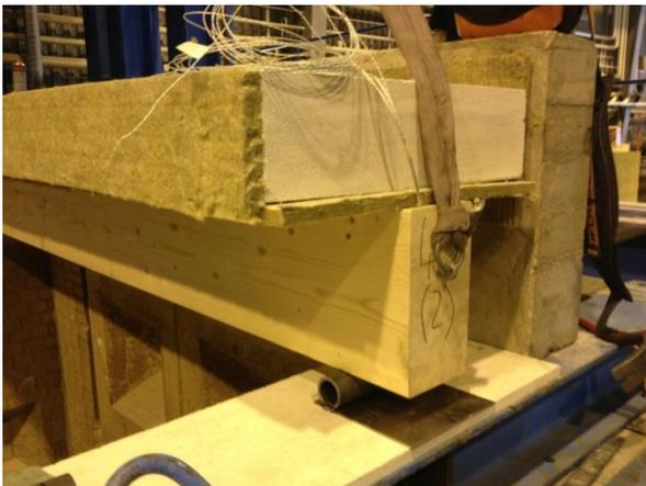
**Figure 3.3, one of the beams just after being placed in position on the furnace for fire test 1 (note the incorrect orientation of the roller support which was later corrected)**
