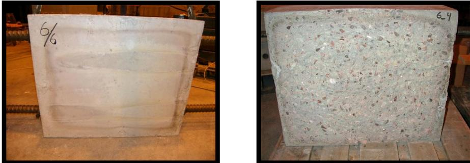
Figure 2.35 (Left) Concrete including PP powder unloaded during the test. (Right) Same concrete loaded in compression during the test.
