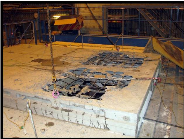
Figure 2.30 Severe fire spalling during fire testing of a high strength concrete floor slab exposed to unilateral fire. Photo Robert Jansson (published with permission of the client).
