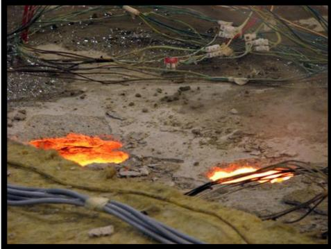
Figure 2.29 Severe spalling breaking through the 200 mm thick concrete specimen after 40 minutes of exposure to the hydrocarbon fire curve. Photo Robert Jansson
