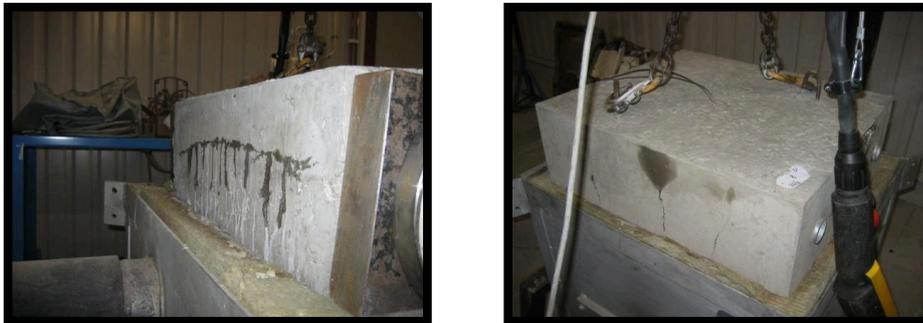
Figure 2.36 One sided heating of small specimens from the underside. (Left) Small slab loaded in compression, example of crack evolution in the load direction. Water is pouring out from the horizontal crack. (Right) Unloaded small slab, cracks develop vertically from the heated surface.
