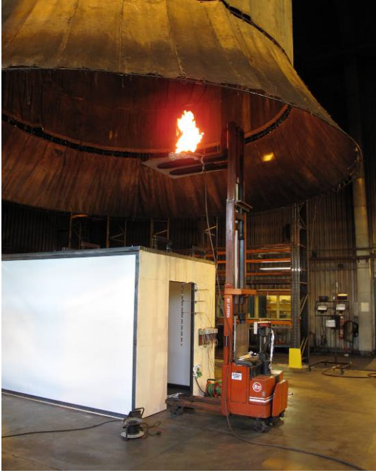
Figure 9 Calibration of HRR measurement with propane burner.
