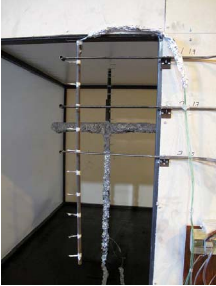
Figure 7 Velocity and temperature measurement in door opening. Smoke measurement and thermocouple tree in middle of room can also be seen.
