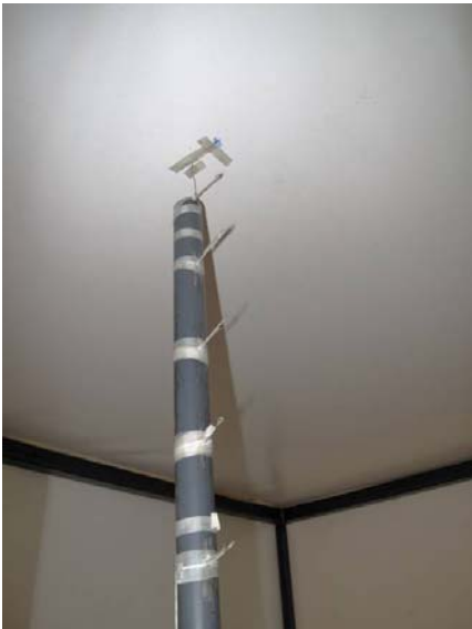
Figure 8 Thermocouple tree and TC mounted on inside of ceiling.
