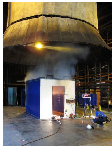
Figure 42 Smoke layer in room and decomposition/evaporation of coating material (Test 3, time: 13:18).
