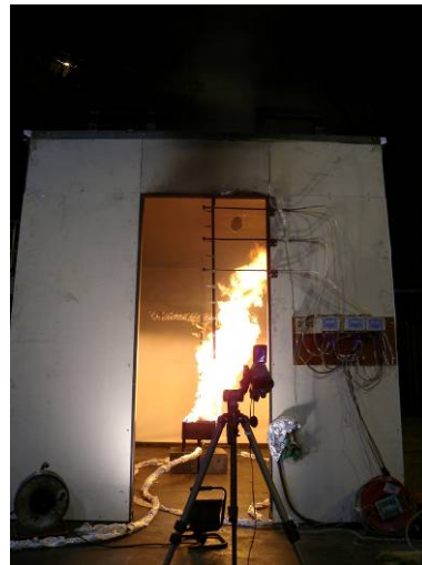
Figure 127 Burner at 300 kW. Flame leaning to the right and a small hole has opened in the ceiling (Test 10, time 22:32).
