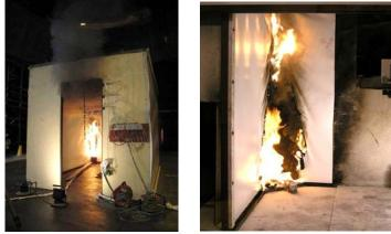
Prescriptive fire safety regulations which in detail regulate the design and classification of building components can exclude the use of textile materials which do not conform to the required fire rating. In such cases, a performance based approach to comply with the overall fire safety level of the building can be a valid alternative. Both these methods of fire design using textile building materials have been used in the Contex-T project, with particular emphasis on textile membranes.
