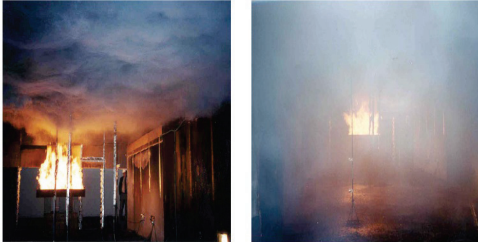
Figure 6.3 Smoke layer characteristics, prior and after sprinkler actuation (Kumar, 2006).
