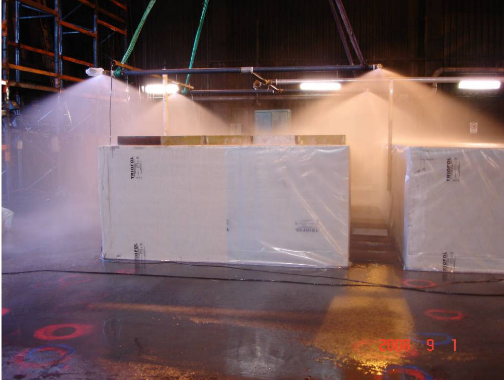
Figure 2- 32 Test 11: The overall water distribution.
