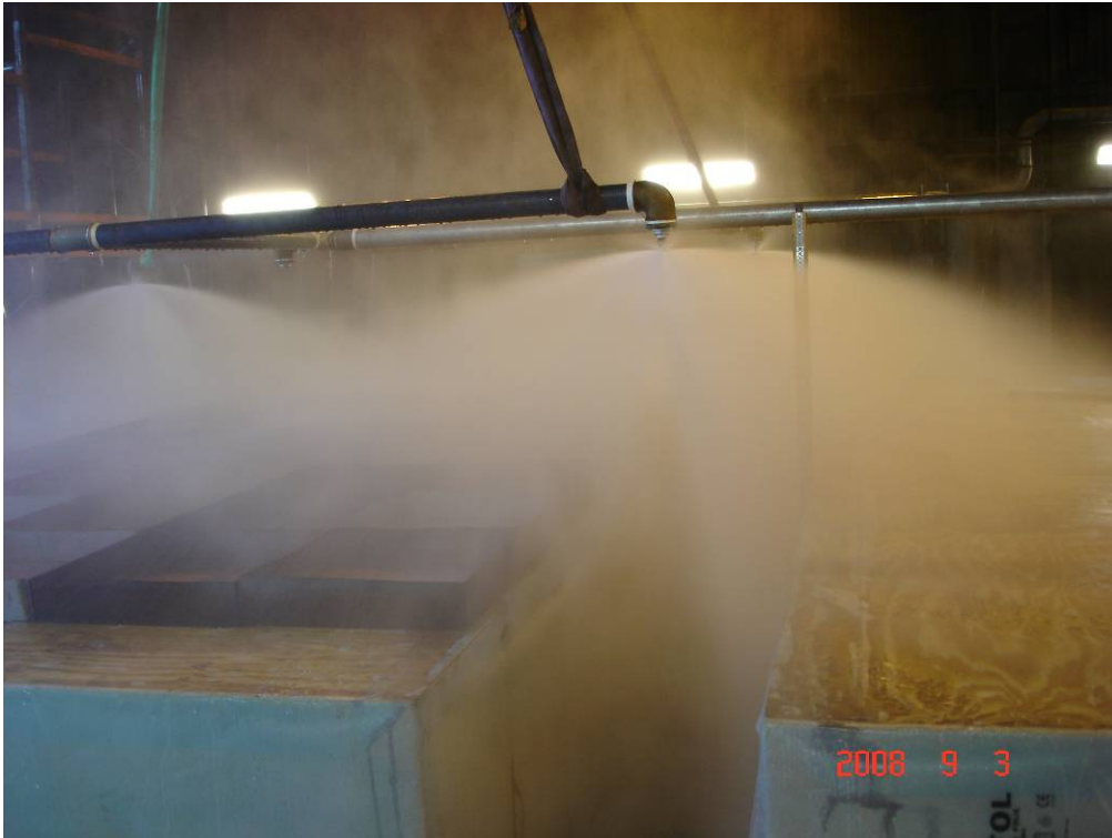
Figure 2- 65 Test 22: A close-up image of the water distribution down the flue space between the stands.
