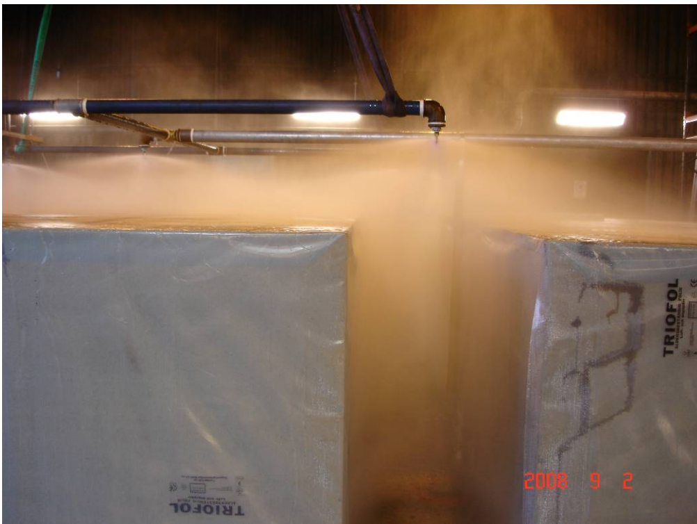
Figure 2- 54 Test 18: A close-up image of the water distribution down the flue space between the stands.
