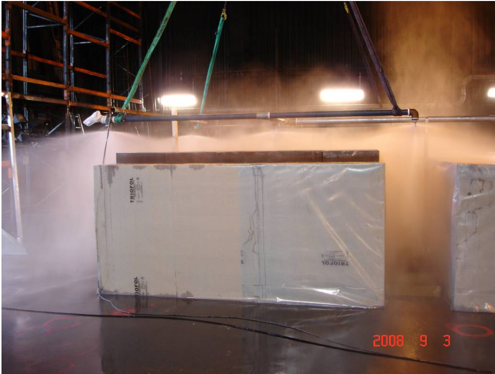
Figure 2- 59 Test 20: The overall water distribution.
