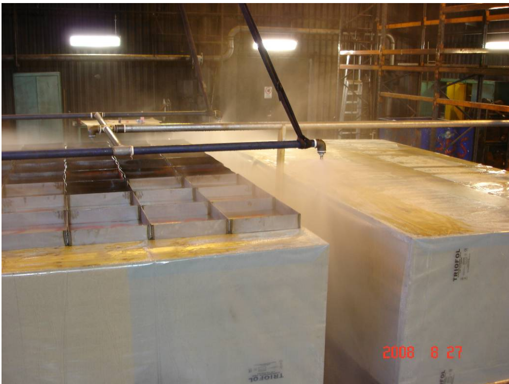
Figure 2- 3 Test 1: The water distribution over the tops of the stands.
