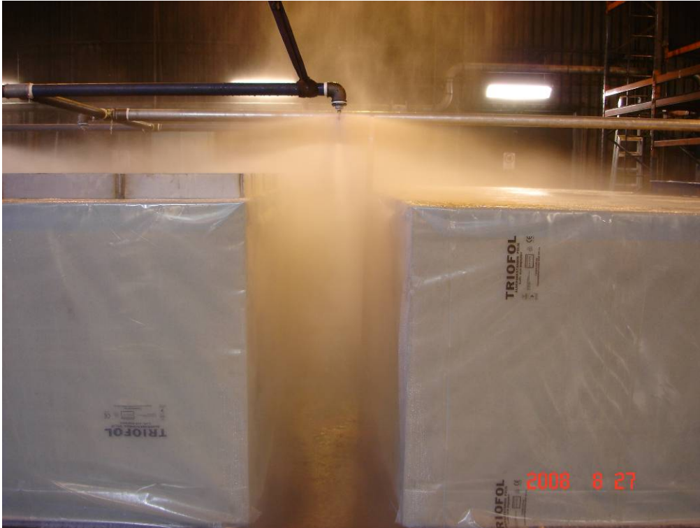
Figure 2- 2 Test 1: The water distribution in the flue space between the stands.
