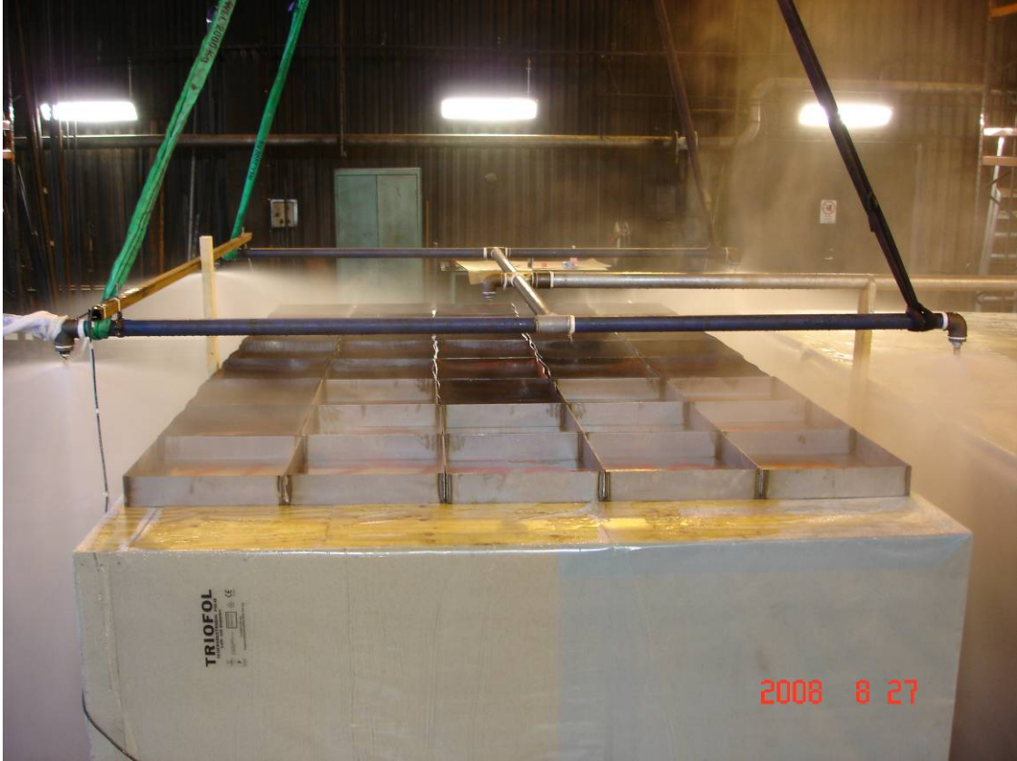
Figure 1 The test set-up shown when flowing four medium velocity nozzles installed 250 mm above the top rim of the 40 water collector trays positioned at the top of the left hand side stand. Eight additional trays were positioned at the floor, between the two stands.
