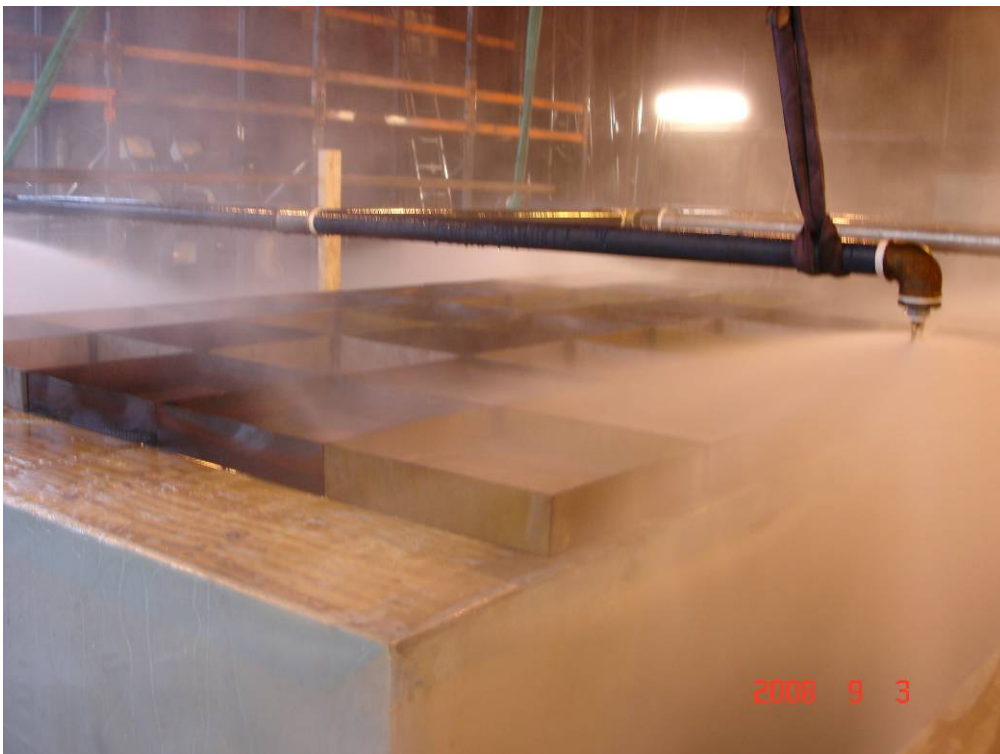
Figure 2- 57 Test 19: A close-up image of the water distribution down the flue space between the stands.
