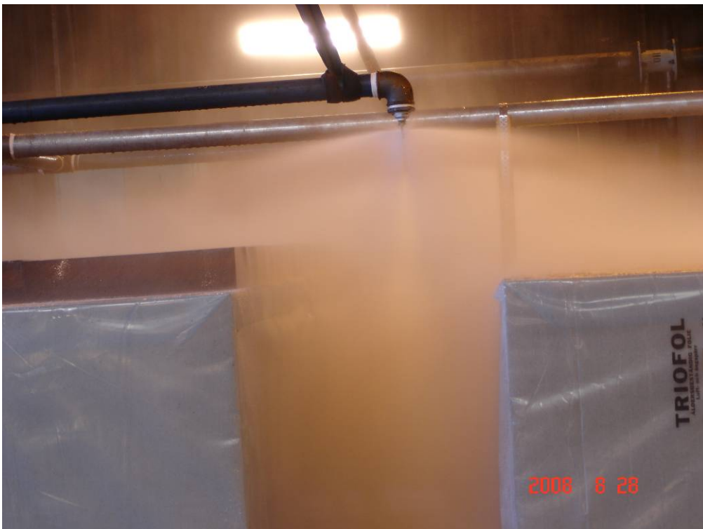
Figure 2- 9 Test 3: A close-up image of one of the medium velocity nozzles.
