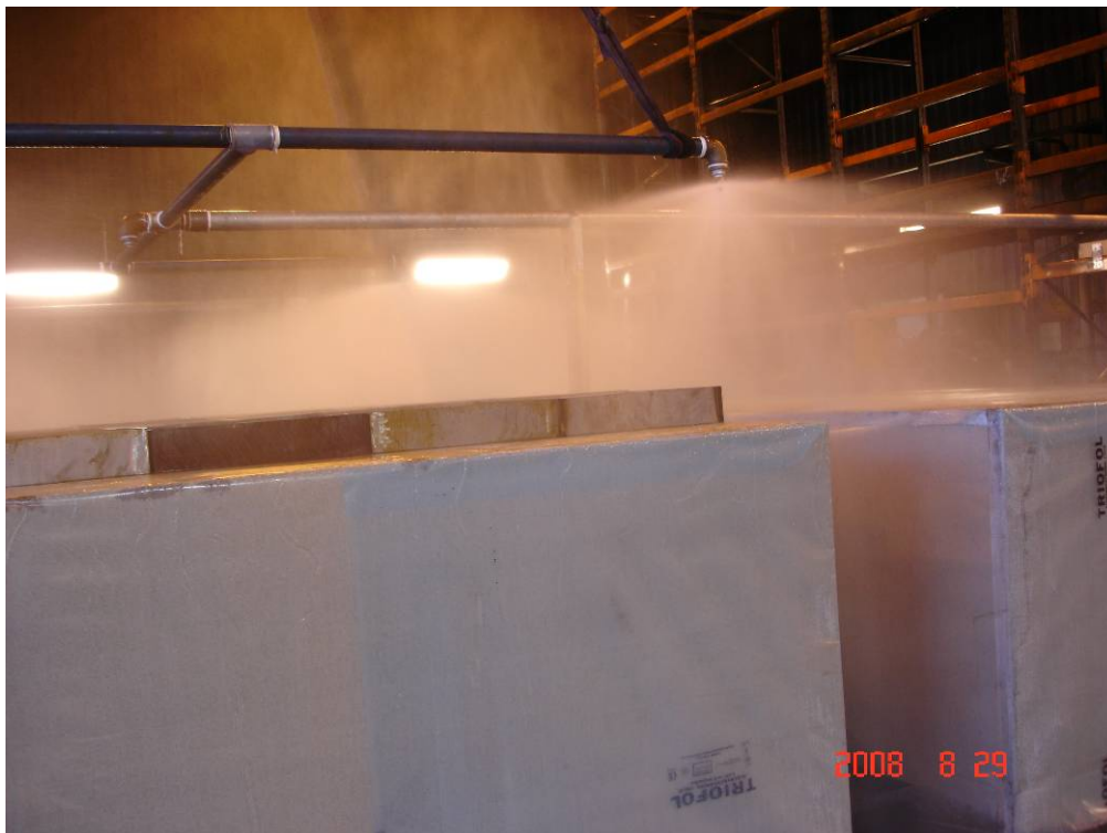
Figure 2- 21 Test 7: The water distribution from one of the medium velocity nozzles.
