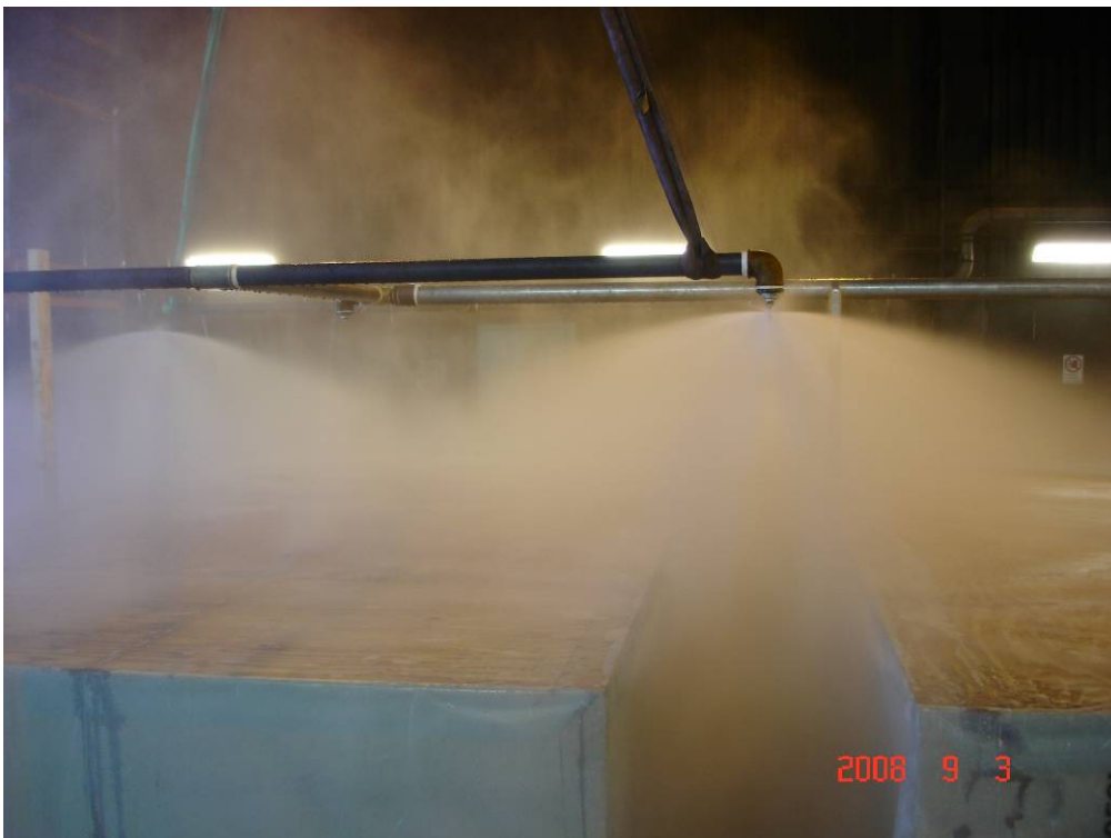
Figure 2- 63 Test 21: A close-up image of the water distribution down the flue space between the stands (shown without the water collector trays).
