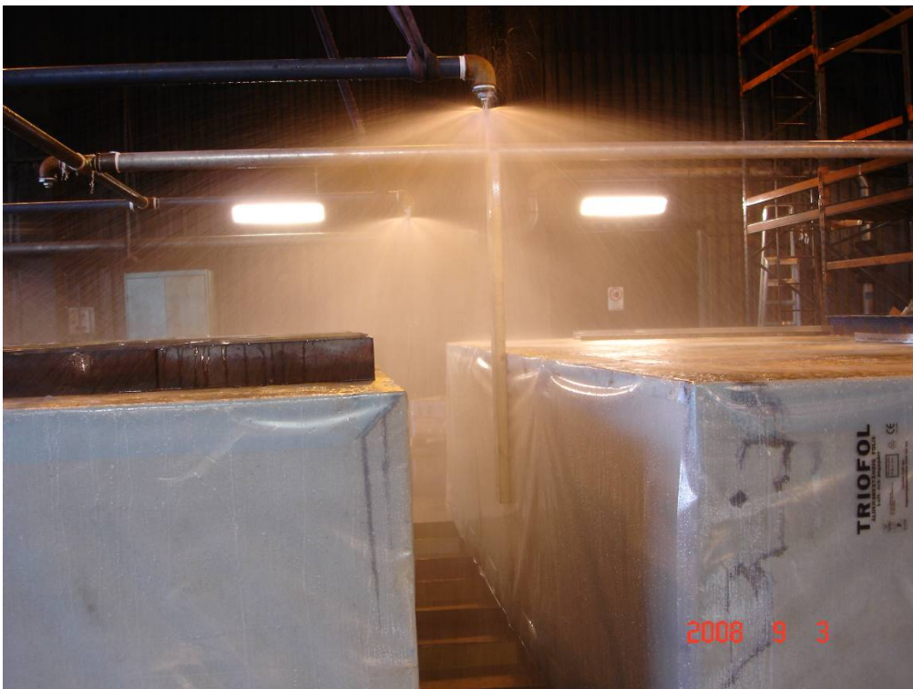
Figure 2- 69 Test 23: A close-up image of the water distribution down the flue space between the stands.
