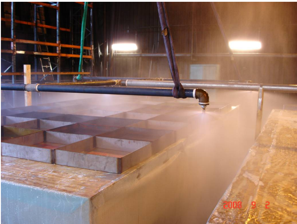
Figure 2- 51 Test 17: A close-up image of the spray patterns of the medium velocity nozzles.
