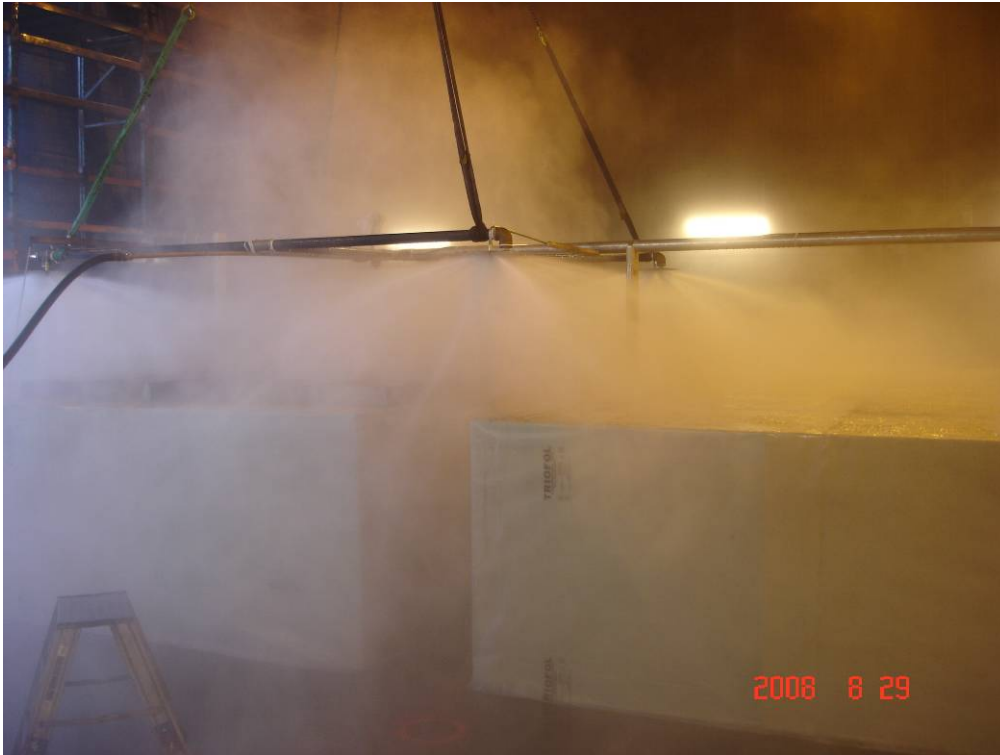
Figure 2- 17 Test 6: The overall water distribution. Note the mobility of the small water droplets in the area between the four nozzles.
