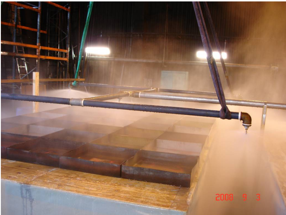
Figure 2- 60 Test 20: A close-up image of the water distribution down the flue space between the stands.
