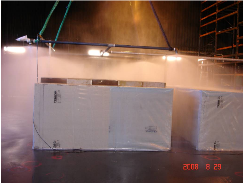
Figure 2- 20 Test 7: The overall water distribution.
