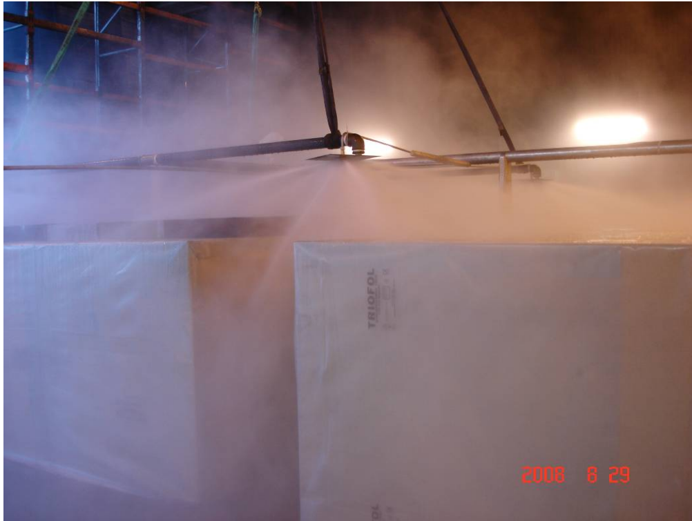
Figure 2- 14 Test 5: The overall water distribution.
