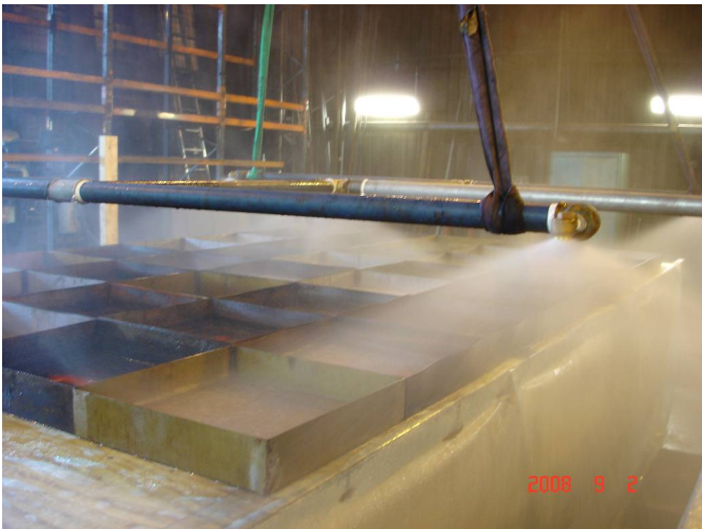
Figure 2- 45 Test 15: A close-up image of one of the medium to high velocity nozzles.
