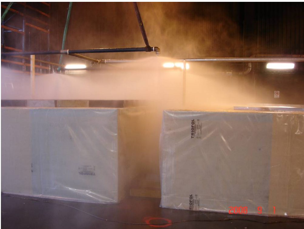
Figure 2- 27 Test 9: The overall water distribution.
