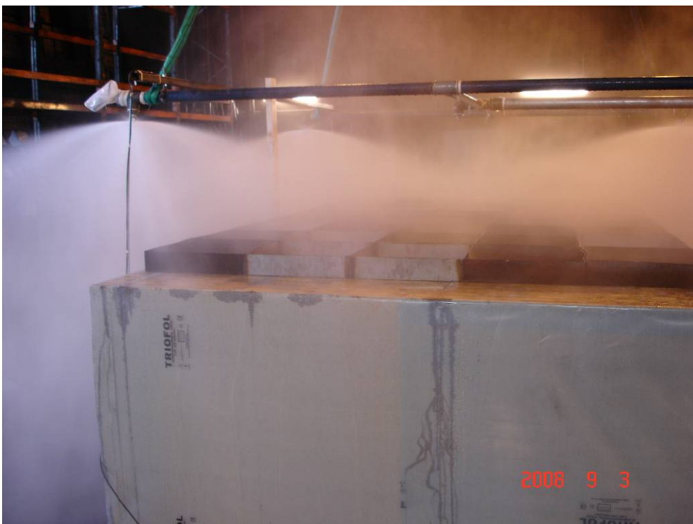
Figure 2- 66 Test 22: A close-up image of the water distribution down over the left hand side stand.
