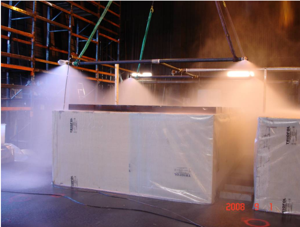
Figure 2- 38 Test 13: The overall water distribution.
