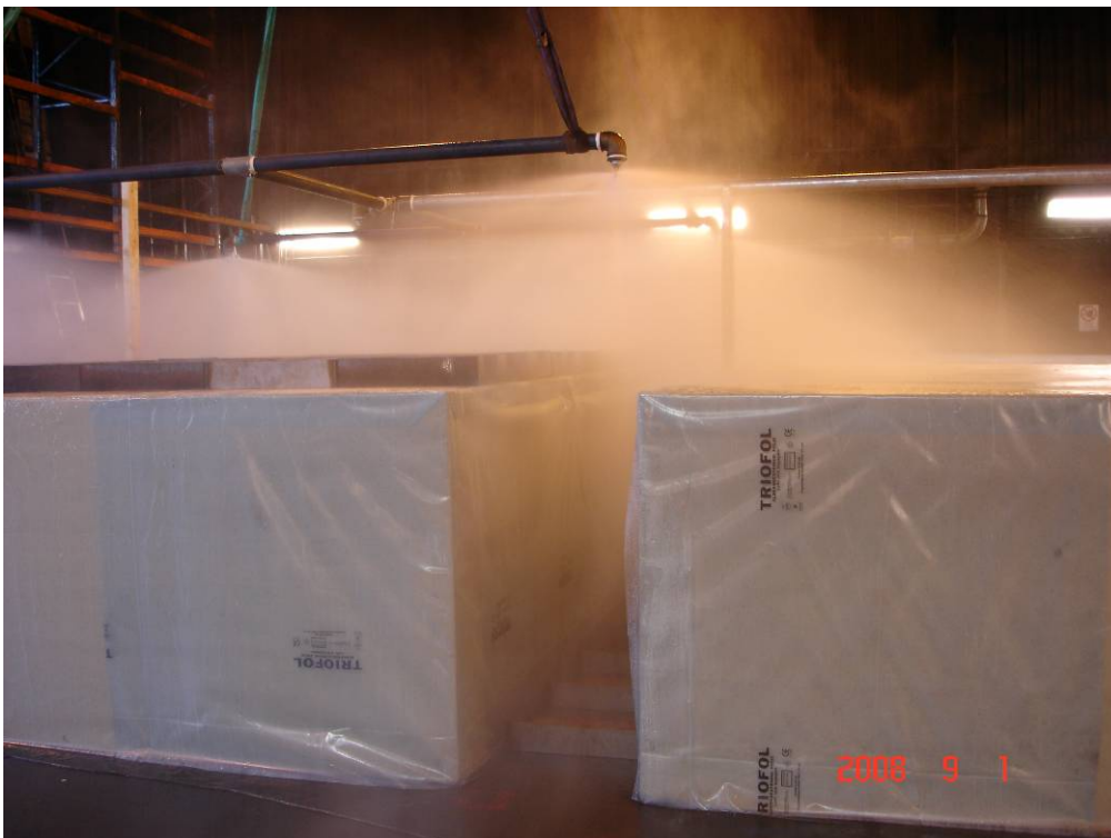
Figure 2- 24 Test 8: A close-up image of one of the medium velocity nozzles.
