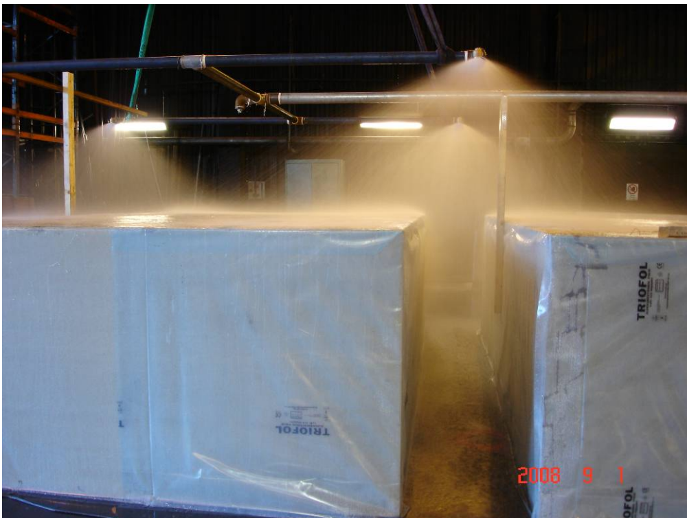
Figure 2- 39 Test 13: The overall water distribution (shown without the water collector trays).
