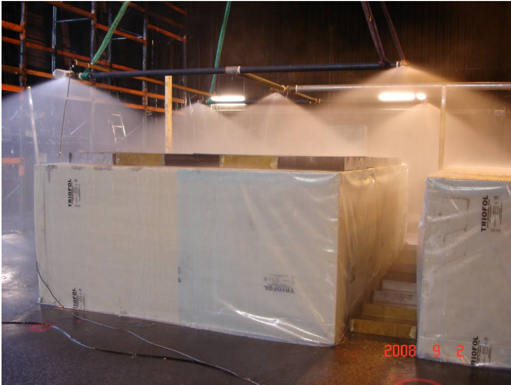
Figure 2- 41 Test 14: The overall water distribution.
