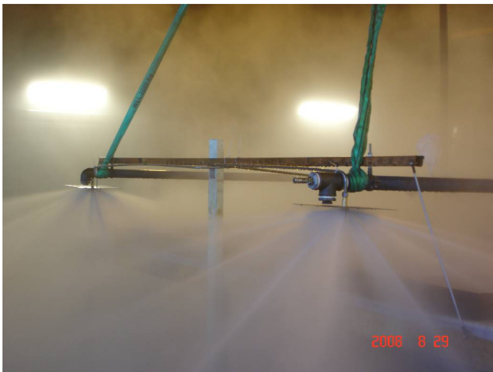
Figure 2- 15 Test 5: A close-up image of two of the water mist nozzles that shows the spray patterns as well as the small steel plate above the nozzles.
