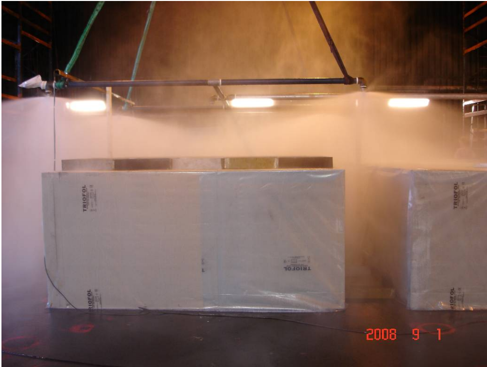
Figure 2- 26 Test 9: The overall water distribution.
