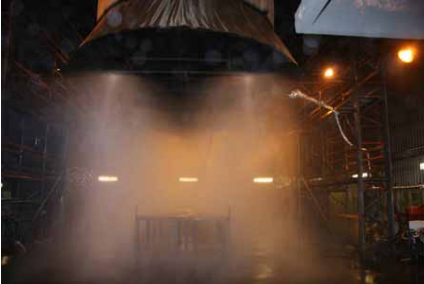
Figure A- 81 Test 8E(10): The water spray from the nozzles prior to the test.
