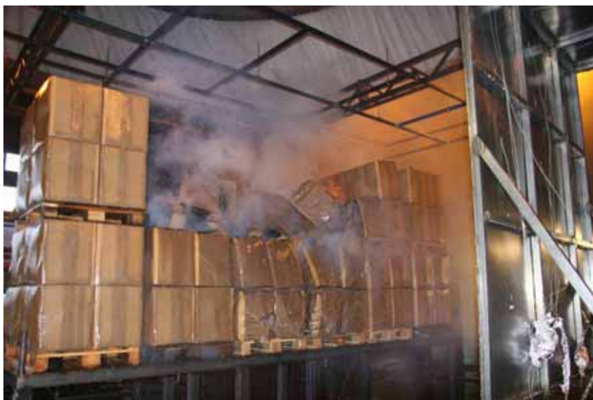
Figure A-32 Test 3E(10): Fire damages as seen from the right hand side.
