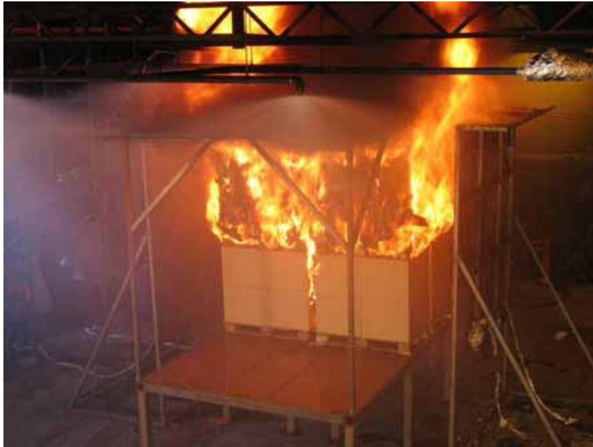
Figure 16 The fire size at the manual activation of the system for the tests without the roof of the trailer mock-up, here exemplified with Test 5S(15). Time 02:13 [min:sec] after fire ignition.
