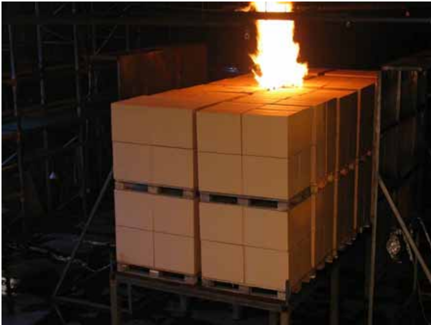
Figure A-82 Test 8E(10): Photo taken 30 seconds after fire ignition.
