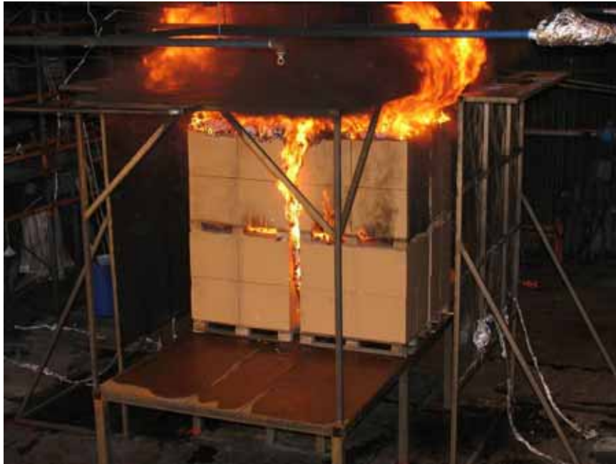
Figure A-131 Test 4S(5): Photo taken 01:30 [min:sec] after fire ignition.
