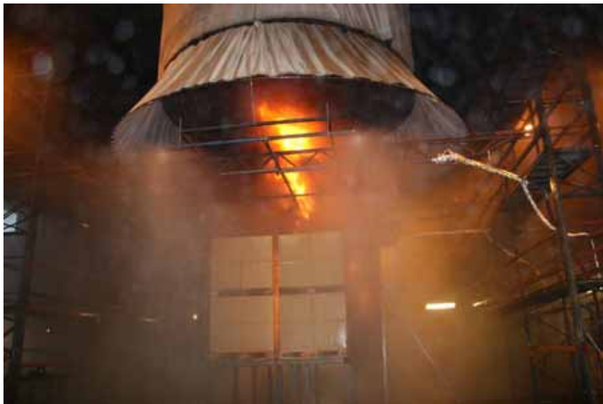
Figure A-28 Test 3E(10): Photo taken 03:00 [min:sec] after fire ignition.
