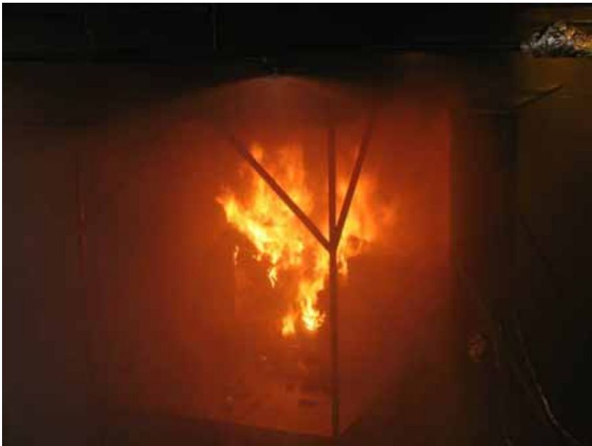
Figure A-114 Test 2S(10): Photo taken at 20:00 [min:sec] after fire ignition. The upper pallet loads have been consumed in the fire.
