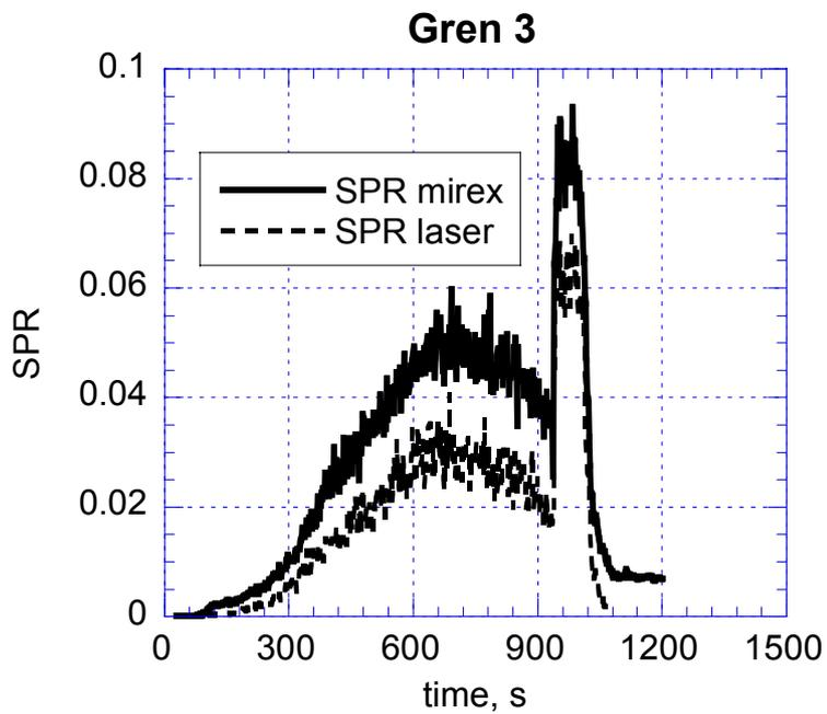
Figure 16 Comparison of SPR obtained by the MIREX and the cone calorimeter for test Gren3.
