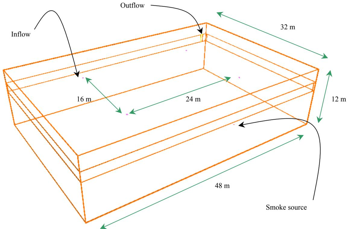
**Figure 17** Schematic of the ventilation system room for the second case where the smoke source is placed right under an air inlet.
