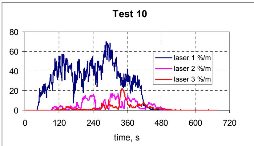
**Figure 21** Smoke signals from lasers, test 10.
