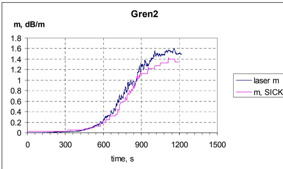
Figure 37 Smoke obscuration measured using a diode laser and the SICK for test Gren2.
