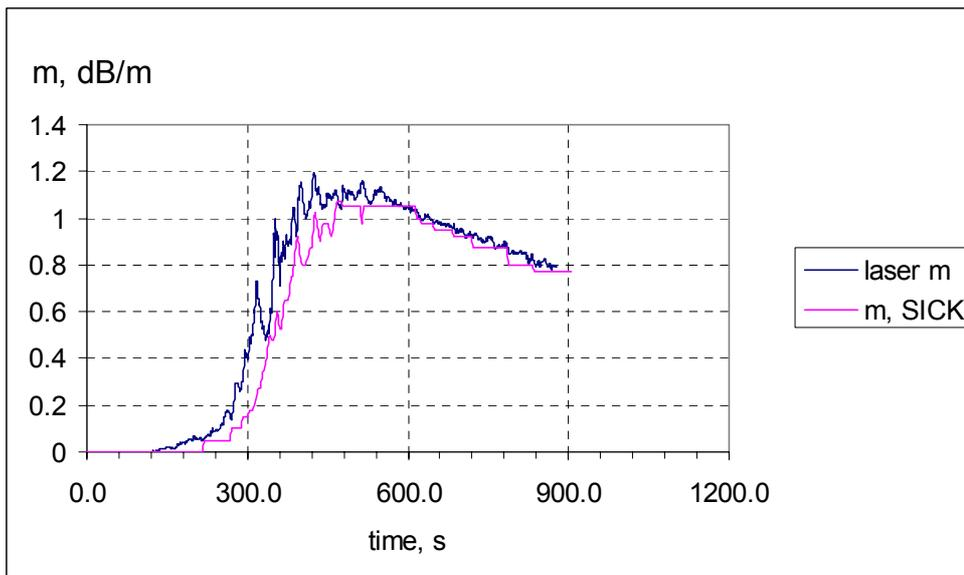
**Figure 8** Smoke obscuration measured using a diode laser and the SICK for test PE1.
