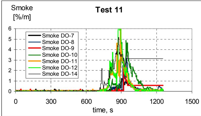
Figure 23 Smoke signals from detectors 7-14, test 11.
