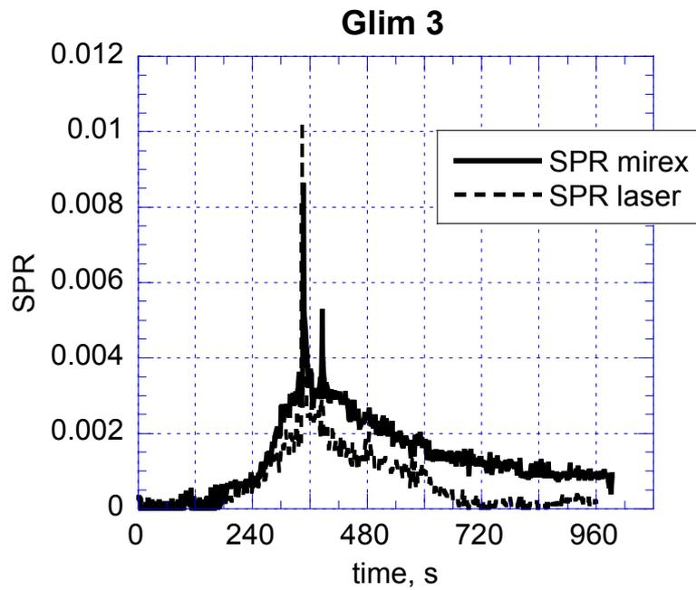
Figure 13 Comparison of SPR obtained by the MIREX and the cone calorimeter for test Lighter3.
