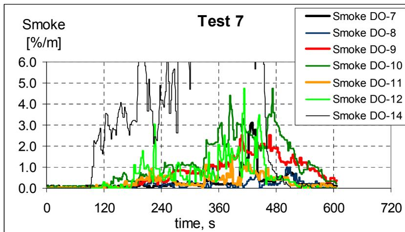
**Figure 17 Smoke signals from detector 7-14, test7.**
