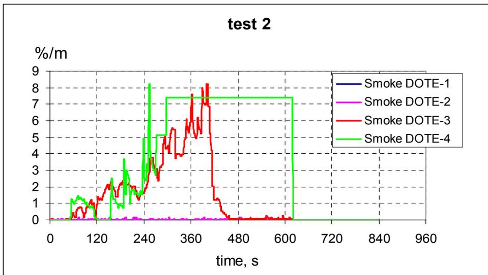
Figure 11 Smoke signals from DOTEs, test2.
