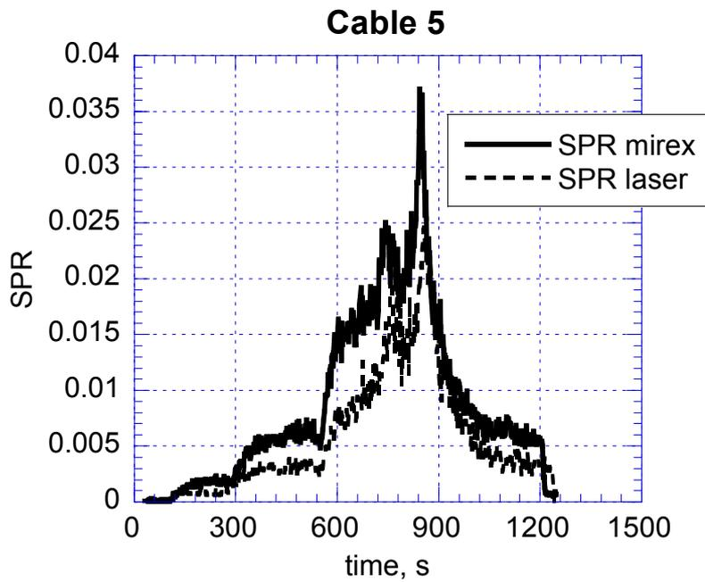
Figure 23 Comparison of SPR obtained by the MIREX and the cone calorimeter for test Cable5.
