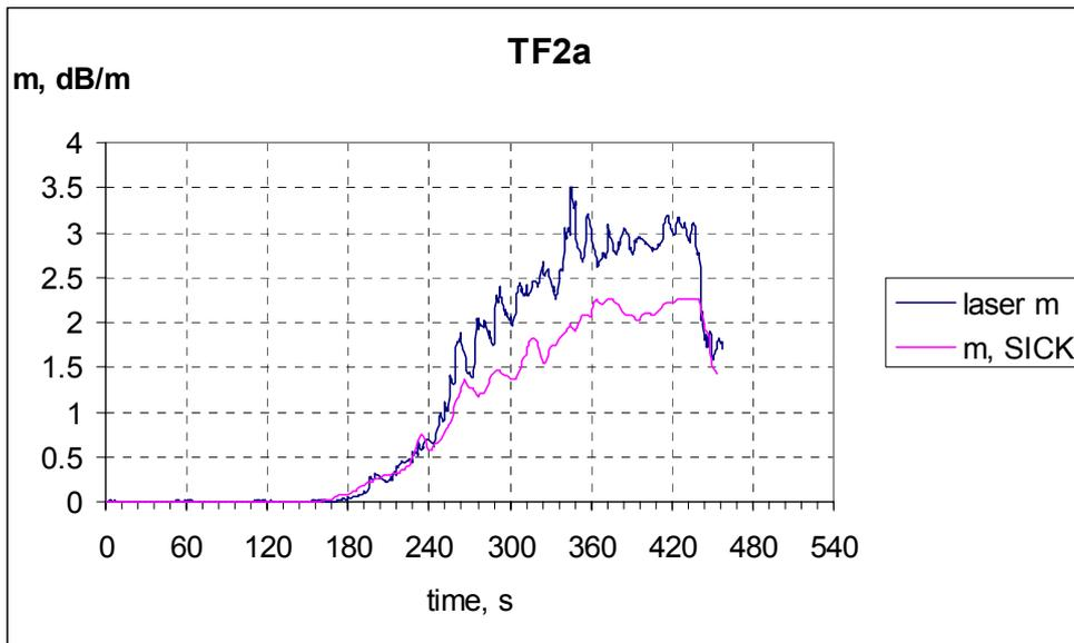
Figure 42 Smoke obscuration measured using a diode laser and the SICK for test TF2a.
