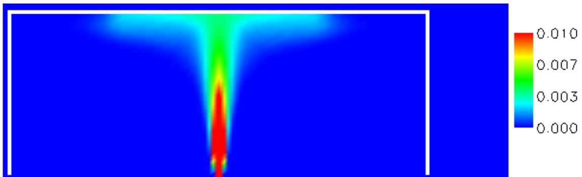
**Figure 11** Smoke profile in the  $1^{\circ}\text{C}/\text{m}$  case after 1 minute.
