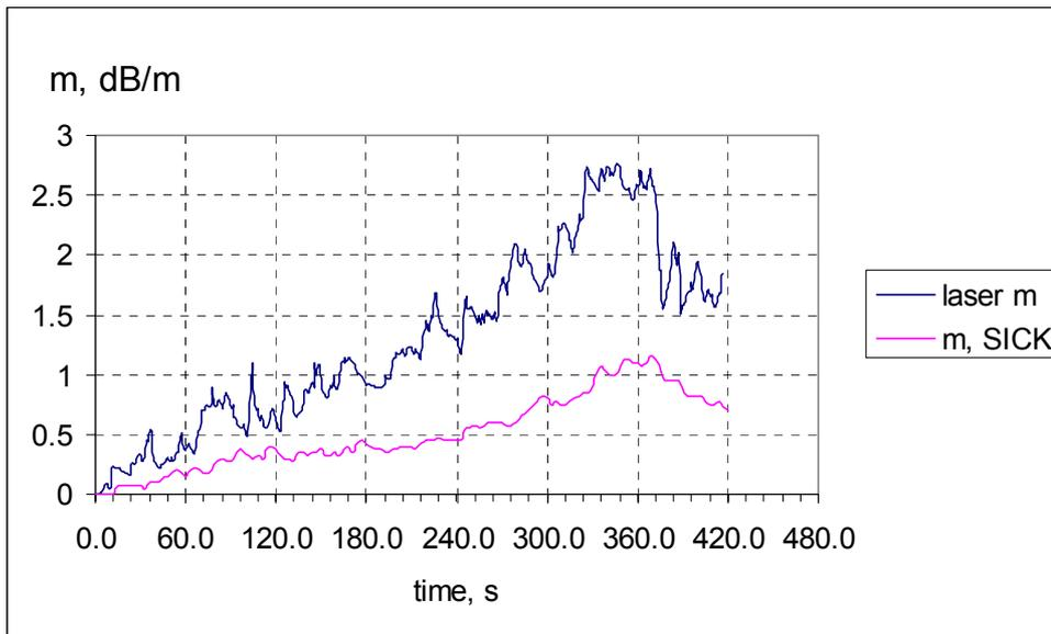
**Figure 7** Smoke obscuration measured using a diode laser and the SICK for test SG3001.
