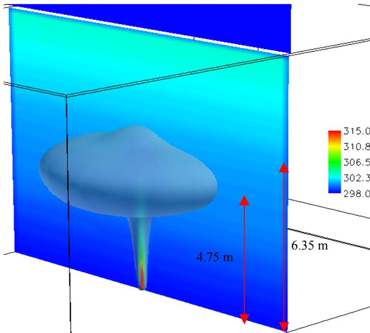
**Figure 12** Smoke profile after 10 minutes in the 0.5 °C/m case.
