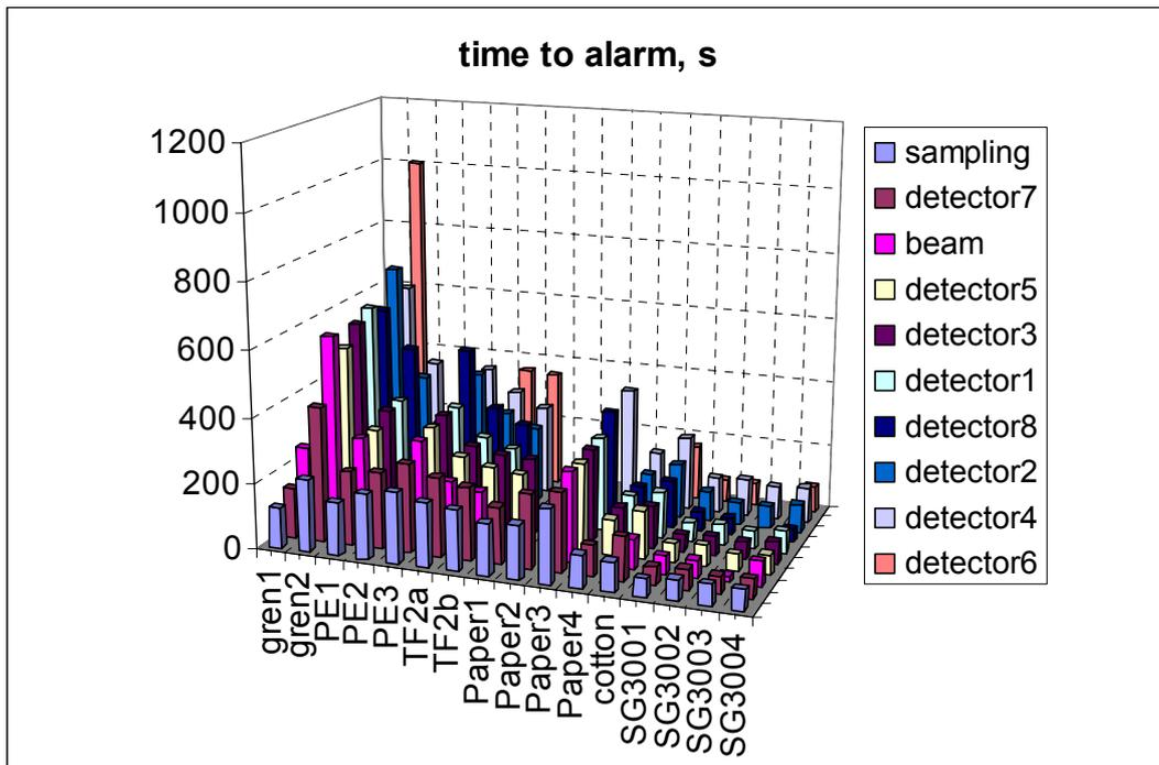
**Figure 6** Time to alarm for the different tests and detectors. For the sampling system level three was used as time to alarm. When no alarm was registered no bar is shown for that case.
