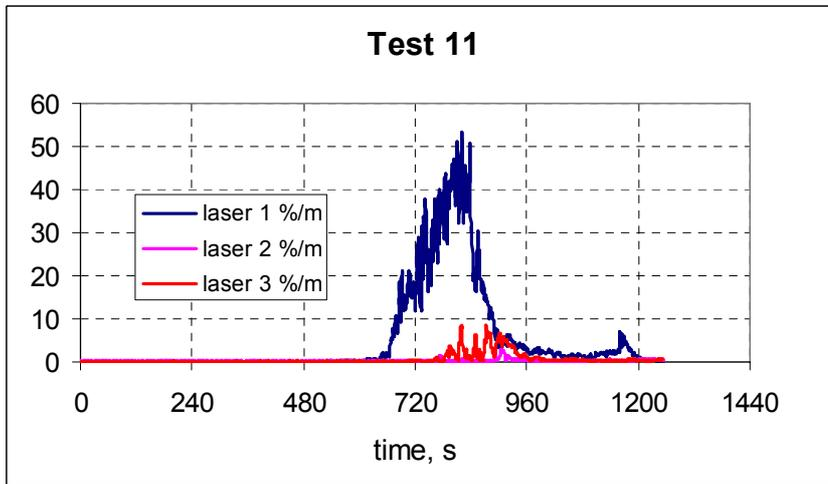
Figure 24 Smoke signals from lasers, test11.
