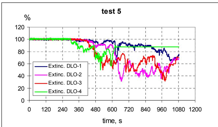
Figure 33 Smoke signals from beam detectors, test5.
