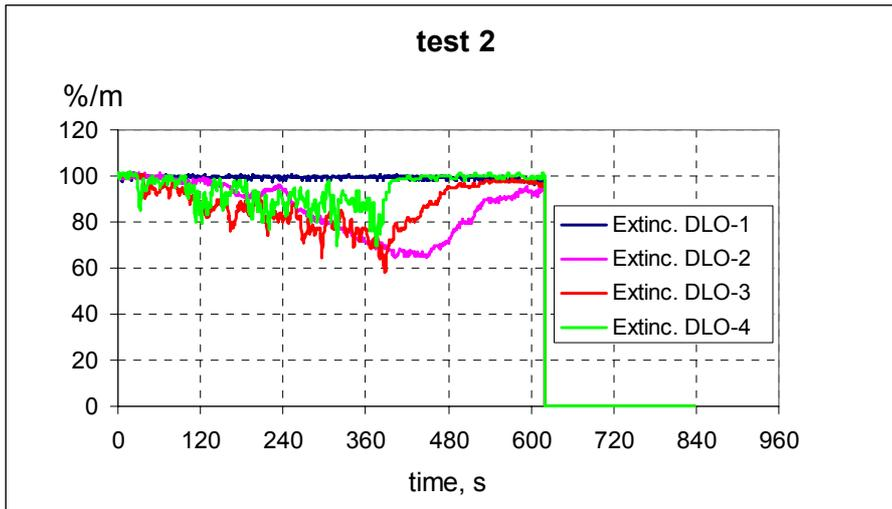
Figure 13 Smoke signals from beam detectors, test 2.
