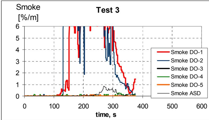
Figure 6 Smoke signals from Detector 1-5 and ASD test3.
