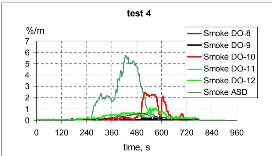
**Figure 23** Smoke signals from detector 8-12 and ASD, test.
