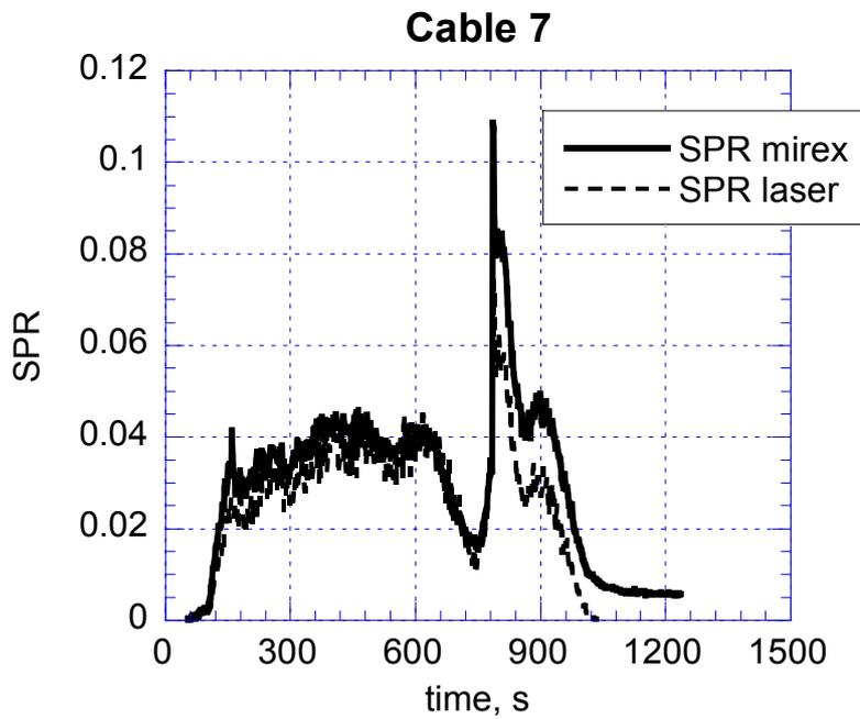
Figure 25 Comparison of SPR obtained by the MIREX and the cone calorimeter for test Cable7.
