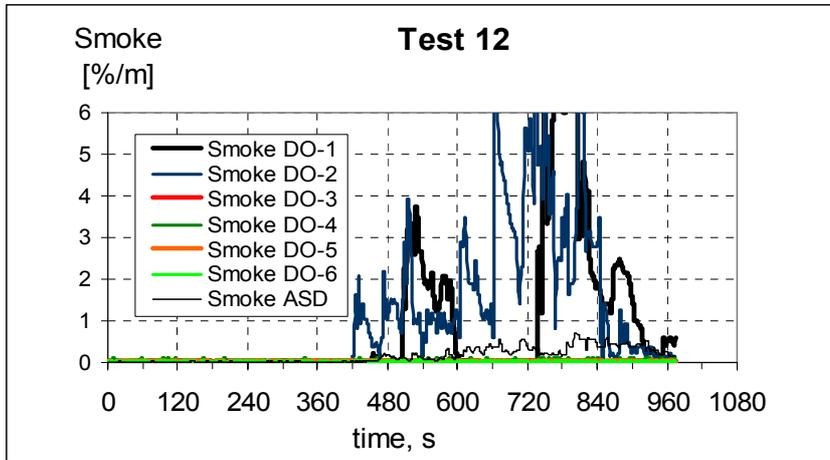
Figure 25 Smoke signals from detector 1-6 and ASD, test 12.
