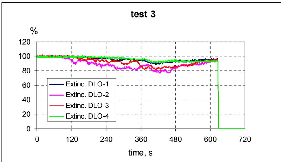
Figure 20 Smoke signal from beam detectors, test3.
