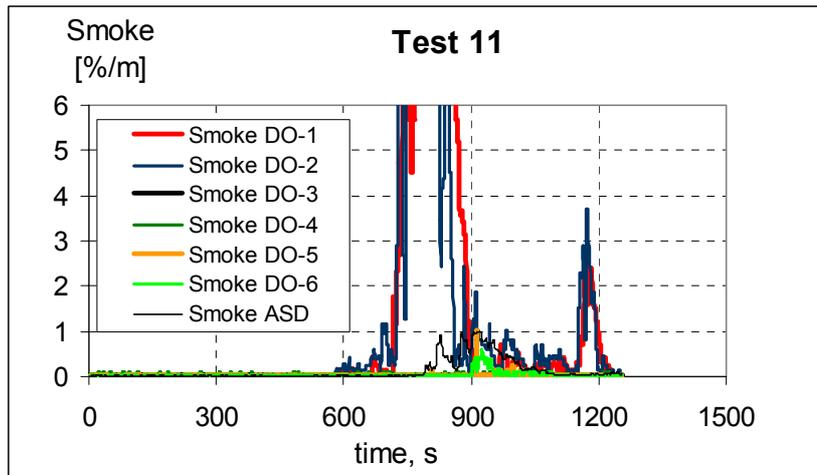
**Figure 22 Smoke signals from detectors 1-6 and ASD, test 11.**
