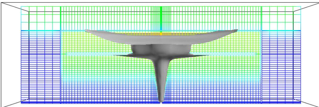
**Figure 35** 3%/m seen from the staircase after 6 minutes. The simulation was made using the Bill and Nam turbulence coefficients; the source had a velocity of 1.5 m/s and a temperature of 340 K.
