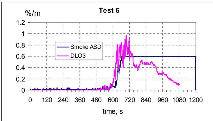
Figure 41 Comparison between sampling system and the beam detector in the vicinity.
