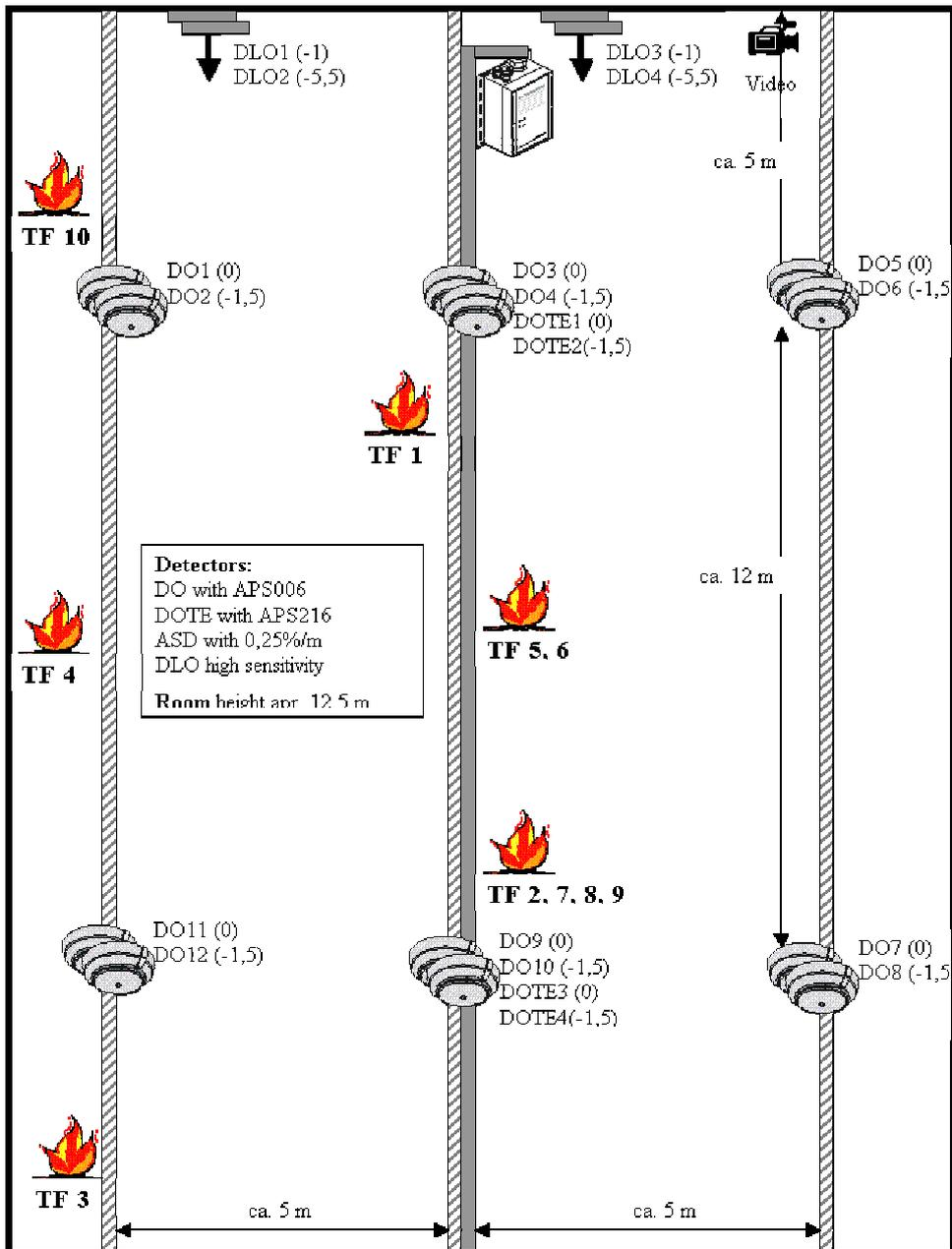
Figure 1 Schematic of detector and fire placement.
