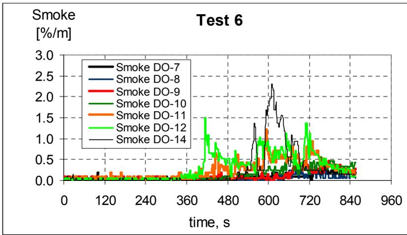
Figure 14 Smoke signals from detector 7-14, test 6.
