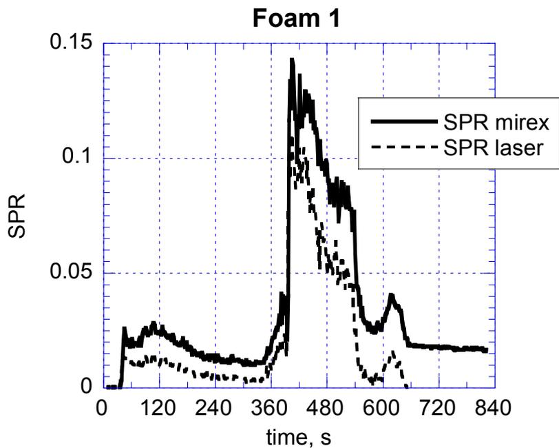
Figure 20 Comparison of SPR obtained by the MIREX and the cone calorimeter for test Foam1.
