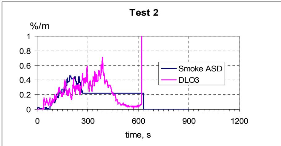
Figure 14 Comparison between ASD and the beam detector in the vicinity, test2.
