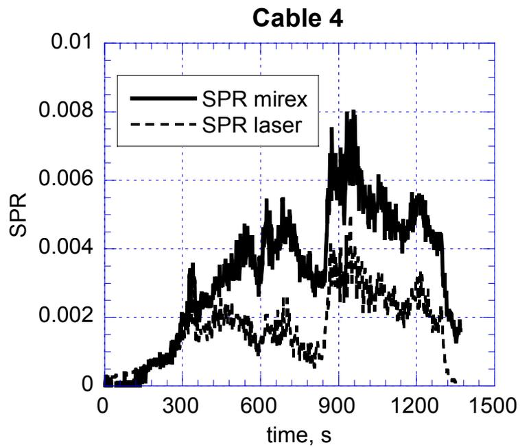
Figure 22 Comparison of SPR obtained by the MIREX and the cone calorimeter for test Cable4.
