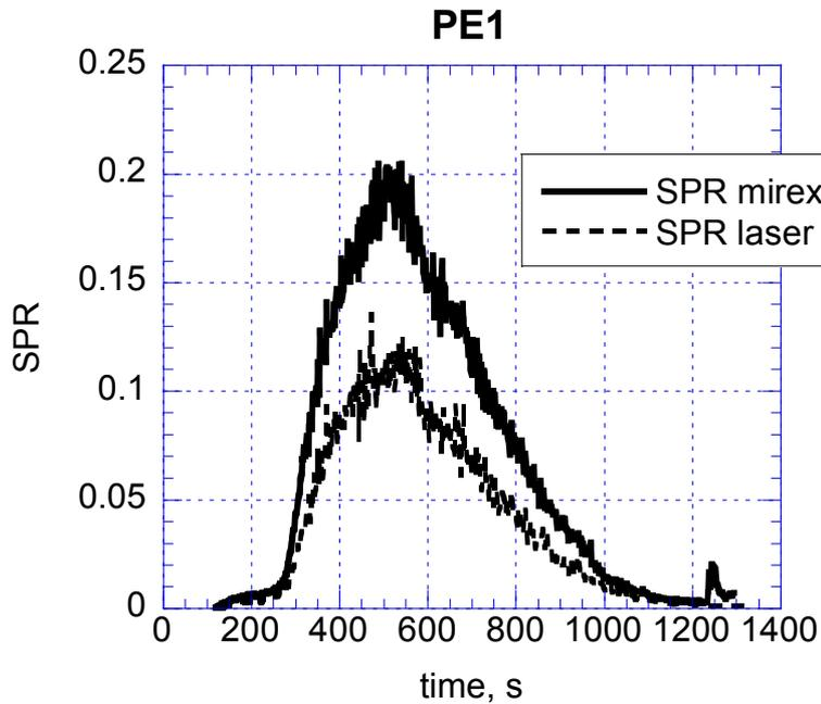
Figure 3 Comparison of SPR (Smoke Production Rate) obtained by the MIREX and the cone calorimeter for test PE1.
