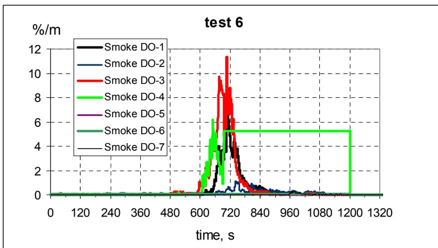
Figure 35 Smoke signals from detector 1-7, test6.
