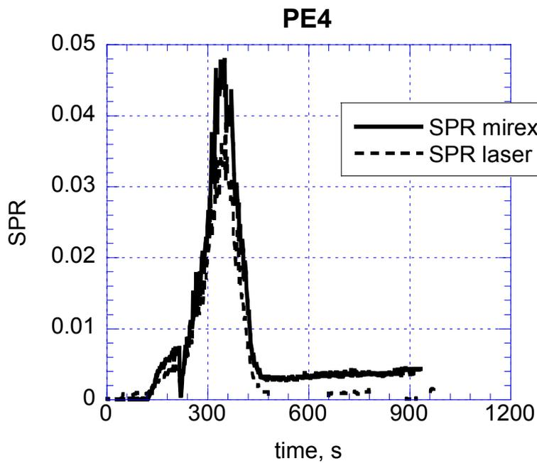
Figure 4 Comparison of SPR obtained by the MIREX and the cone calorimeter for test PE4.
