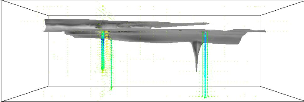
**Figure 43** 0.2%/m for the test 10 case where the smoke generator is placed on the roof to the measuring room. The smoke source is placed below the coloured area in the closest left hand corner.
