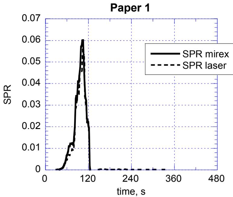
Figure 5 Comparison of SPR obtained by the MIREX and the cone calorimeter for test Paper1.
