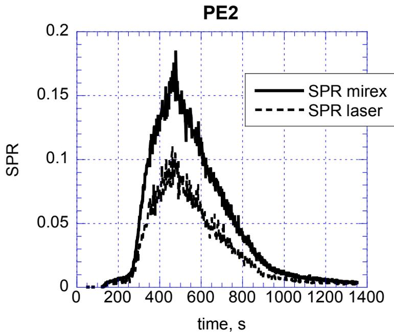
Figure 2 Comparison of SPR obtained by the MIREX and the cone calorimeter for test PE2.
