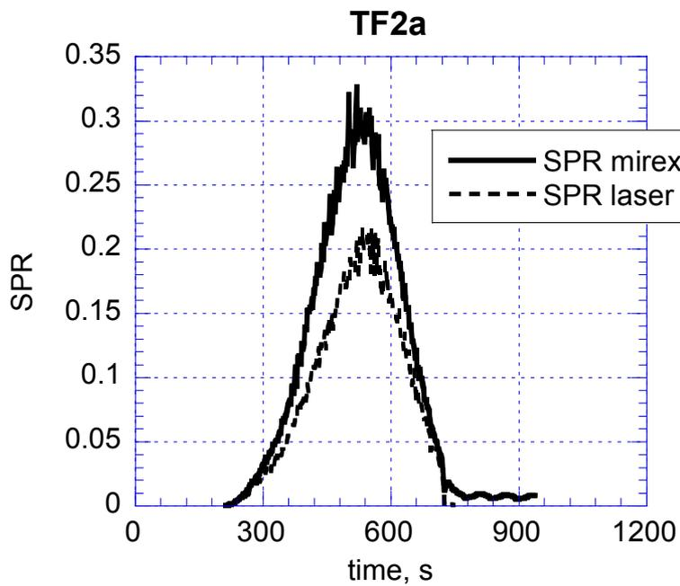
Figure 26 Comparison of SPR obtained by the MIREX and the cone calorimeter for test TF2a.
