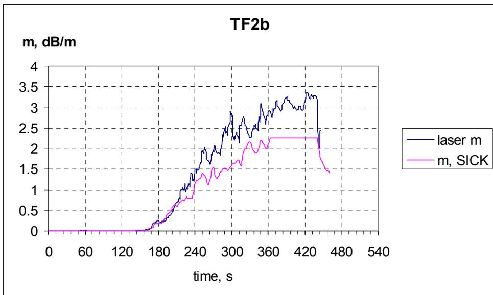
Figure 43 Smoke obscuration measured using a diode laser and the SICK for test TF2b.
