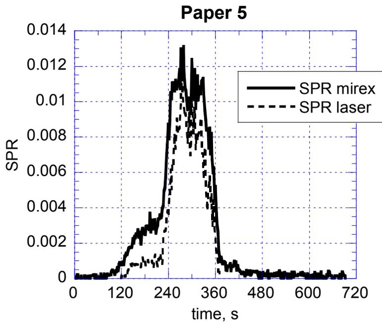
Figure 9 Comparison of SPR obtained by the MIREX and the cone calorimeter for test Paper5.
