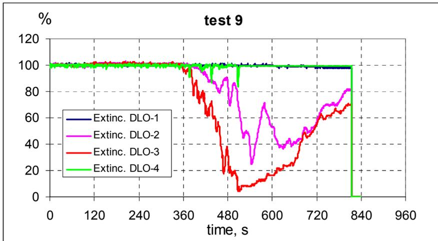
Figure 61 Smoke signals from beam detector, test9.
