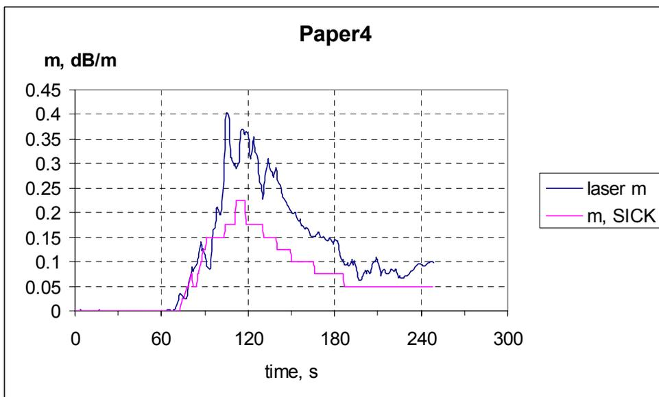
Figure 35 Smoke obscuration measured using a diode laser and the SICK for test Paper4.
