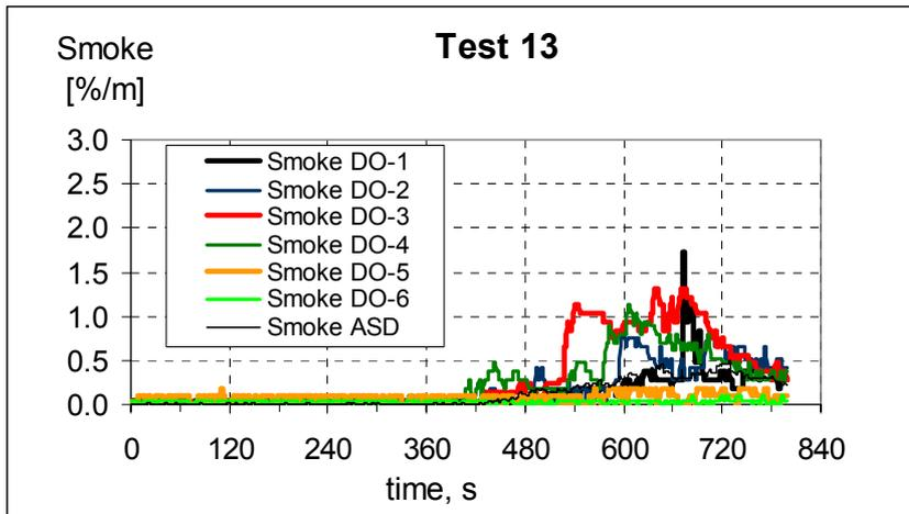
**Figure 28 Smoke signals from detector 1-6 and ASD, test 13.**
