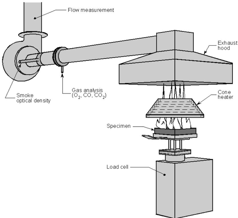
**Figure 1 The Cone calorimeter.**
