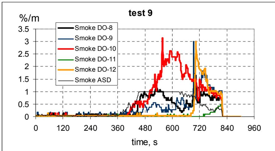
Figure 57 Smoke signals from detectors 8-12 and ASD, test9.
