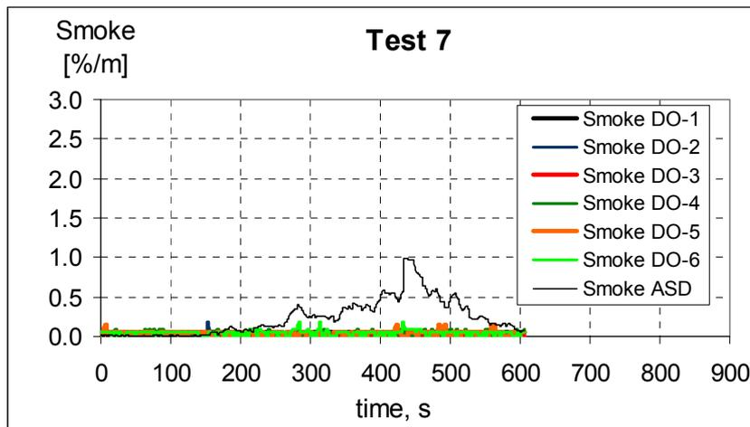
**Figure 16 Smoke signals from detector 1-6 and ASD, test7**
