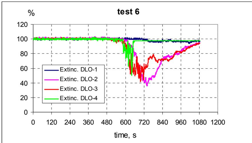
Figure 40 Smoke signals from beam detector, test6.
