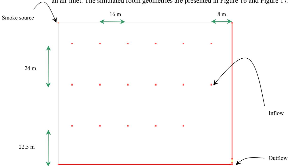
**Figure 16** Schematic of the ventilation system room in the first case with the smoke source in between the air inlets.
