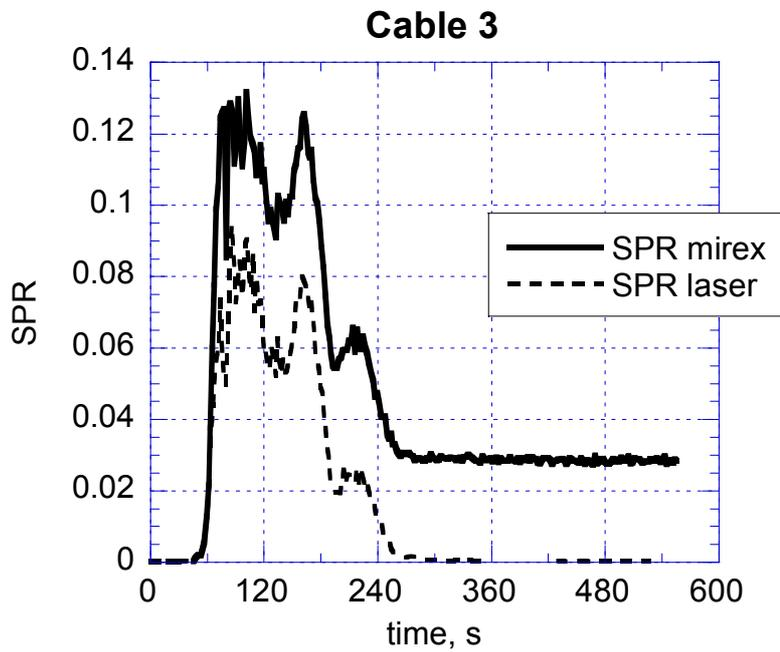
Figure 19 Comparison of SPR obtained by the MIREX and the cone calorimeter for test Cable3.
