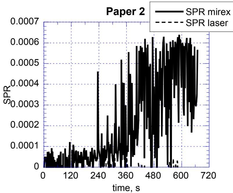
Figure 6 Comparison of SPR obtained by the MIREX and the cone calorimeter for test Paper2.
