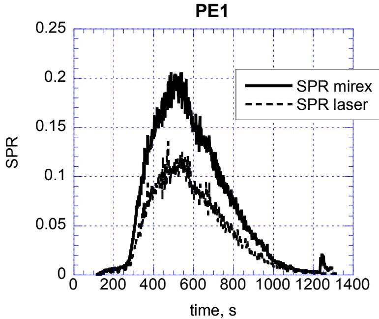
Figure 1 Comparison of SPR obtained by the MIREX and the cone calorimeter for test PE1.
