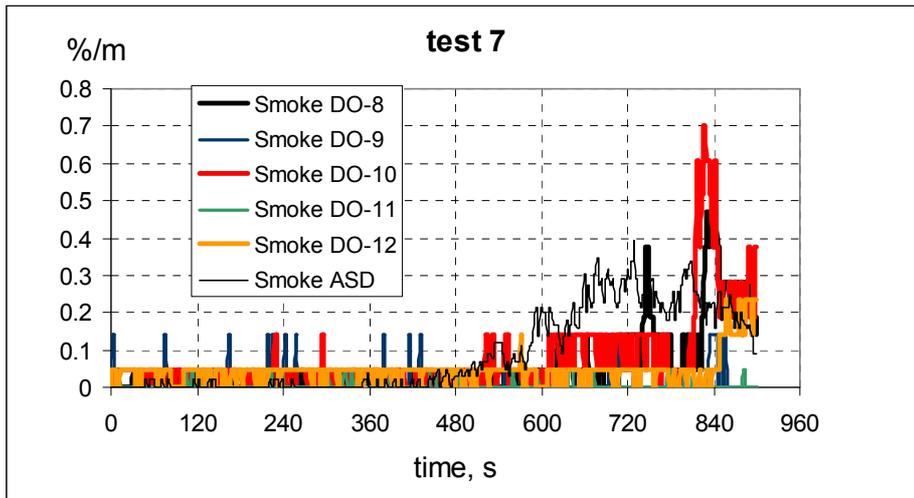
Figure 43 Smoke signals from detector 8-12 and ASD, test7.
