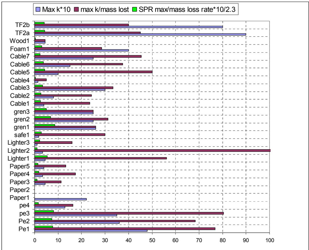
**Figure 2** Maximum extinction coefficient times 10, maximum extinction coefficient divided by mass loss rate (g/s) and SPR divided by mass loss rate recalculated to  $\text{ob}/\text{m}^3$  for the experiments conducted.
