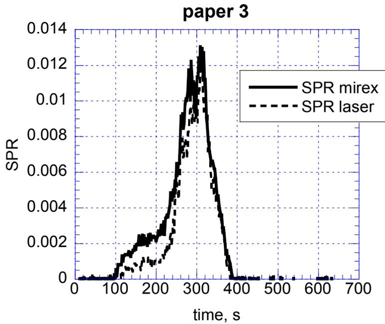
Figure 7 Comparison of SPR obtained by the MIREX and the cone calorimeter for test Paper3.
