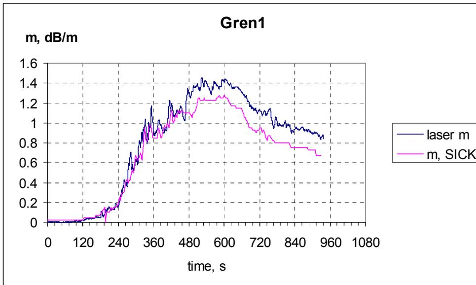
Figure 36 Smoke obscuration measured using a diode laser and the SICK for test Gren1.
