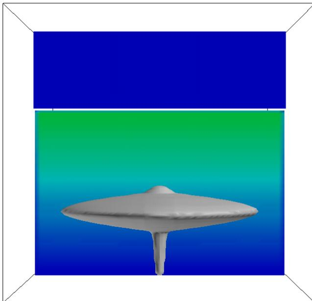
**Figure 15** Smoke field after 5 minutes for the volumetric source and a temperature gradient of  $1^{\circ}\text{C}/\text{m}$ . The smoke levels out at 3.9 m. This should be compared with the 3.75 m in Figure 13.
