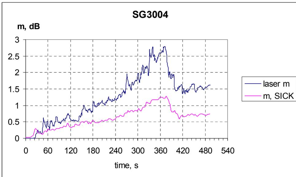
Figure 31 Smoke obscuration measured using a diode laser and the SICK for test SG3004.
