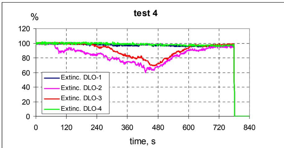
Figure 26 Smoke signals from beam detectors, test4.
