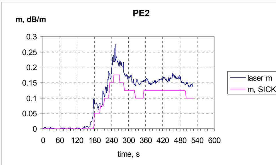
Figure 40 Smoke obscuration measured using a diode laser and the SICK for test PE2.
