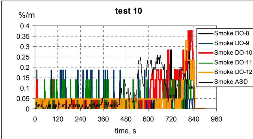
Figure 64 Smoke signals from detector 8-12 and sampling system, test 10.
