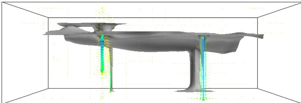
**Figure 42** 0.1%/m for the test 10 case where the smoke generator is placed on the roof to the measuring room. The smoke source is placed below the coloured area in the closest left hand corner.
