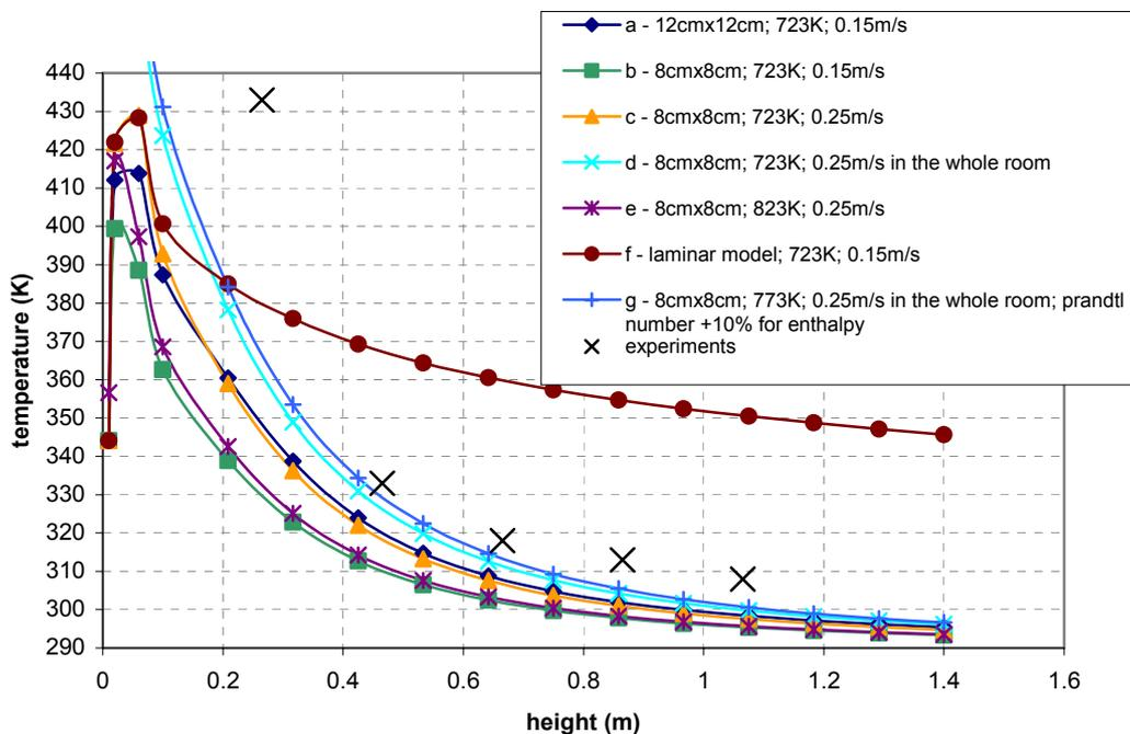
Figure 9 Temperature profile above the smoke source.
