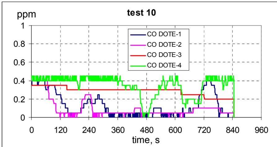
Figure 67 CO signals test 10.
