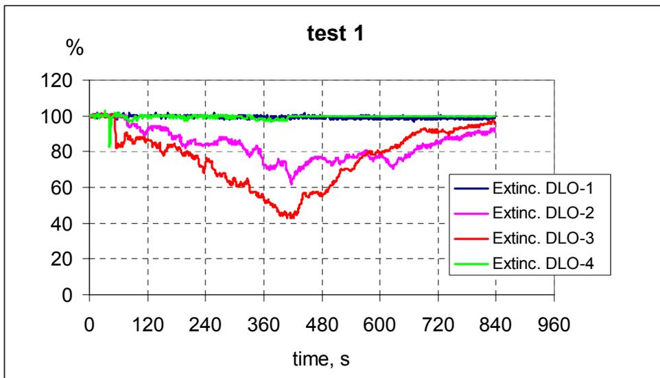
Figure 6 Smoke signals from the beam detectors, test1.
