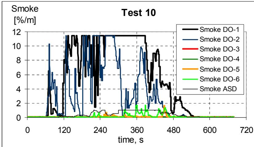
**Figure 19** Smoke signals from detector 1-6 and ASD, test 10.
