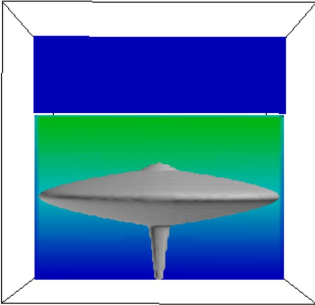
**Figure 14** Smoke field for the volumetric source case after 5 minutes. Temperature gradient of  $0.5^{\circ}\text{C}/\text{m}$ , results in that the smoke levels out at 5 m.
