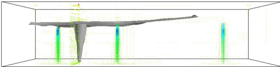
**Figure 45** 0.2 %/m for the test1 case seen from the measuring room towards the workshop.
