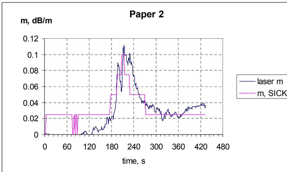
Figure 33 Smoke obscuration measured using a diode laser and the SICK for test Paper2.
