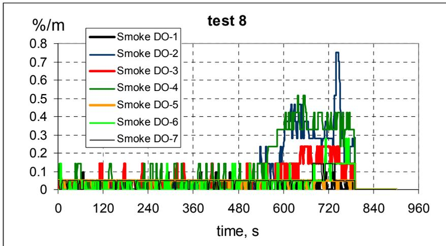
Figure 49 Smoke signals from detectors 1-7, test8.
