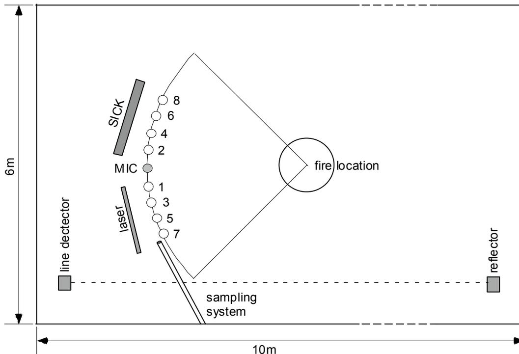
Figure 5 Placement of detectors in the EN54 room at Delta Electronics.
