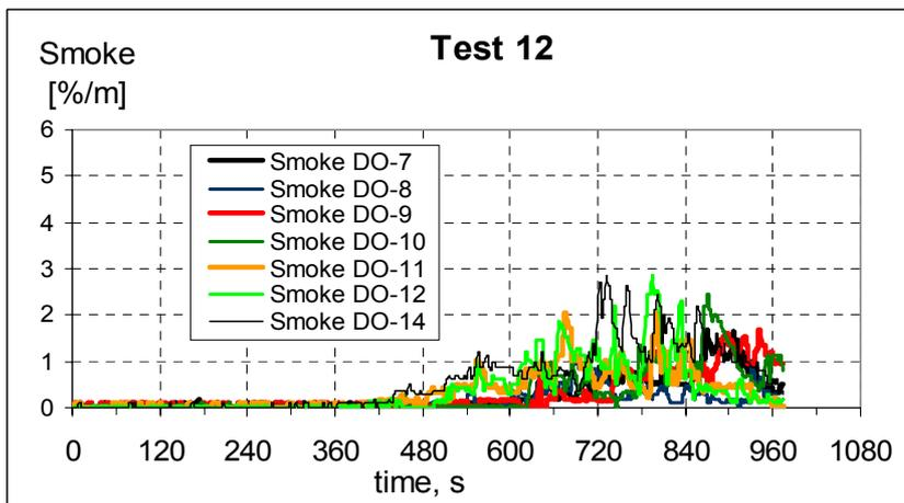
Figure 26 Smoke signals from detector 7-14, test 12.
