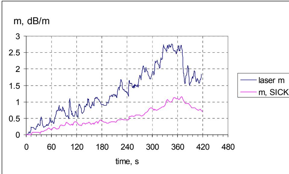
Figure 28 Smoke obscuration measured using a diode laser and the SICK for test SG3001.
