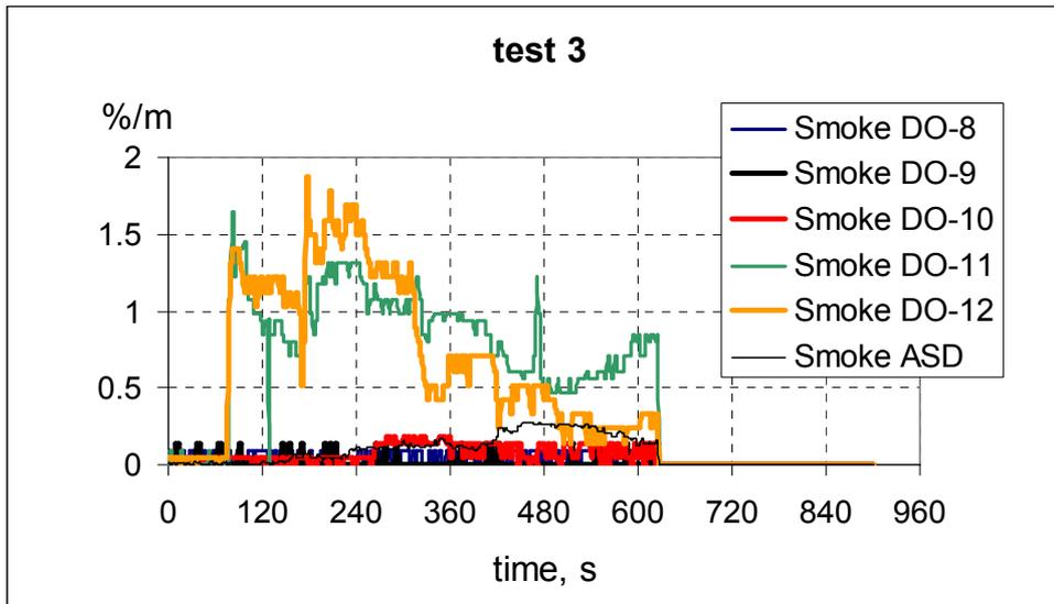
Figure 16 Smoke signals from detectors 8-12 and ASD, test3.
