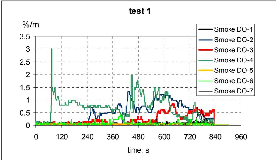
Figure 1 Smoke signals from detector 1-7, test 1
