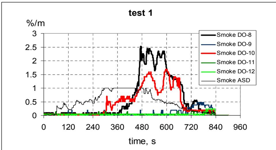
Figure 2 Smoke signals from detector 8-12 and ASD, test1.
