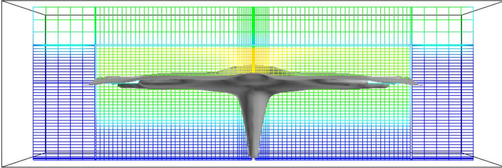
**Figure 33** The iso-curve for 1%/m seen from the staircase looking into the building after 6 minutes using the Bill and Nam k-ε model. The smoke is slowed down by the beam but reaches the ceiling even if the plume is wider in this case.
