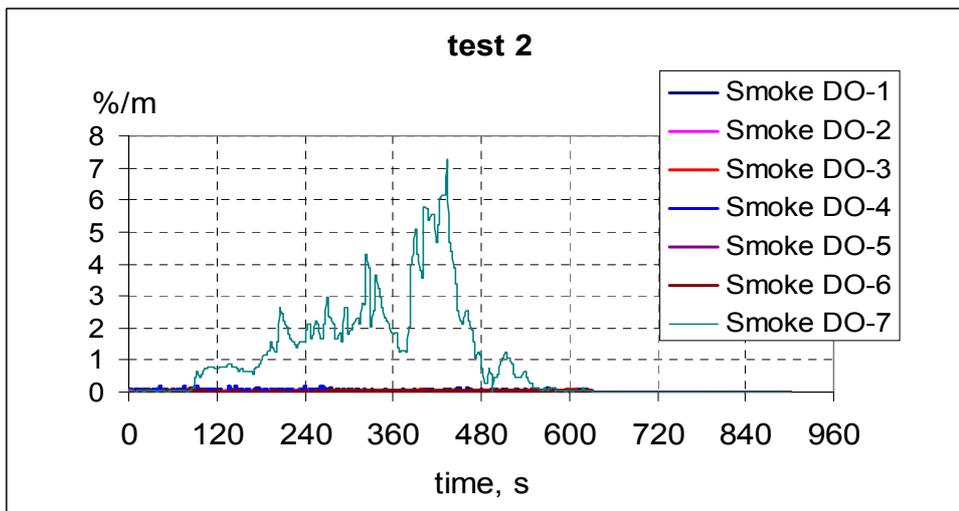
Figure 8 Smoke signals from detector 1-7, test 2.
