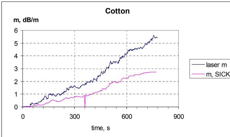
Figure 38 Smoke obscuration measured using a diode laser and the SICK for test Cotton1.
