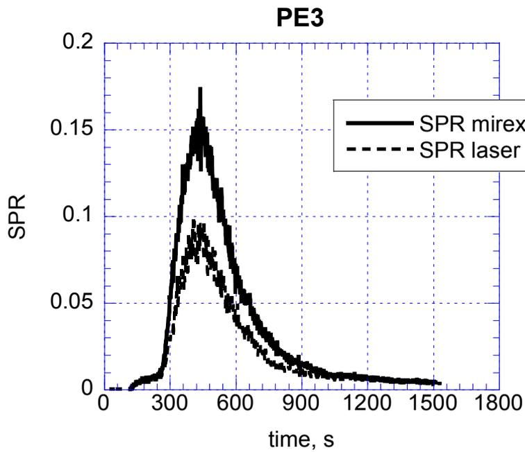
Figure 3 Comparison of SPR obtained by the MIREX and the cone calorimeter for test PE3.
