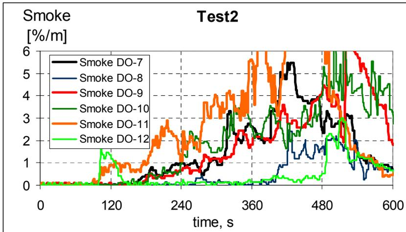
Figure 4 Smoke signals from detector 7-12 test2.
