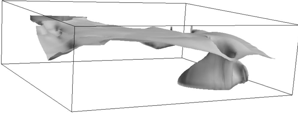
**Figure 19** The smoke field after 15 minutes when the smoke source is placed just under an air inlet. The smoke source is placed on the right hand side in the figure where the smoke emerges from the floor level.
