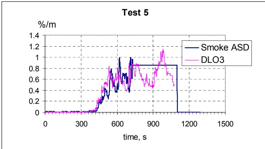
Figure 34 Comparison between ASD and the beam detector in the vicinity.
