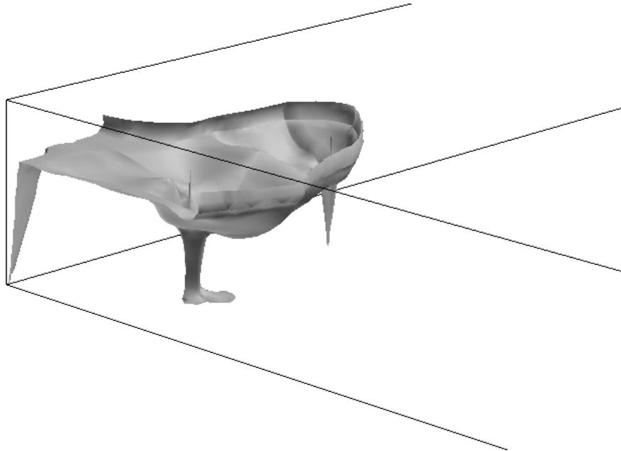
**Figure 20** Smoke field after 10 minutes same scenario as in Figure 18 but this time using the volumetric source.
