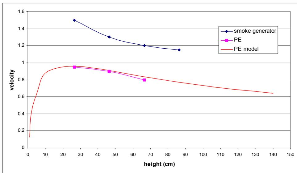
Figure 25 Velocity profile for the SG3000 and the PE box from the cone calorimeter.
