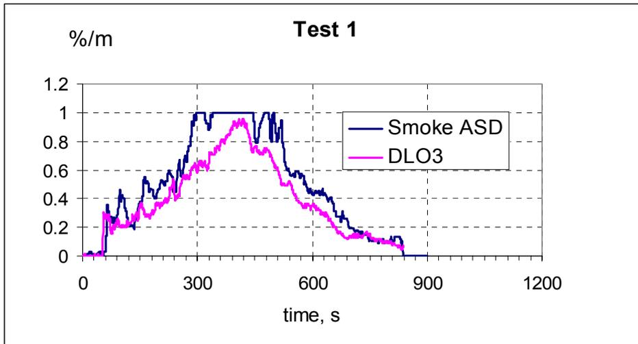
Figure 7 Comparison between sampling system and the beam detector in the vicinity, test1.
