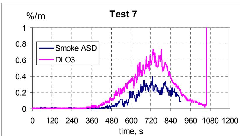
Figure 48 Comparison between sampling system and the beam detector nearby.
