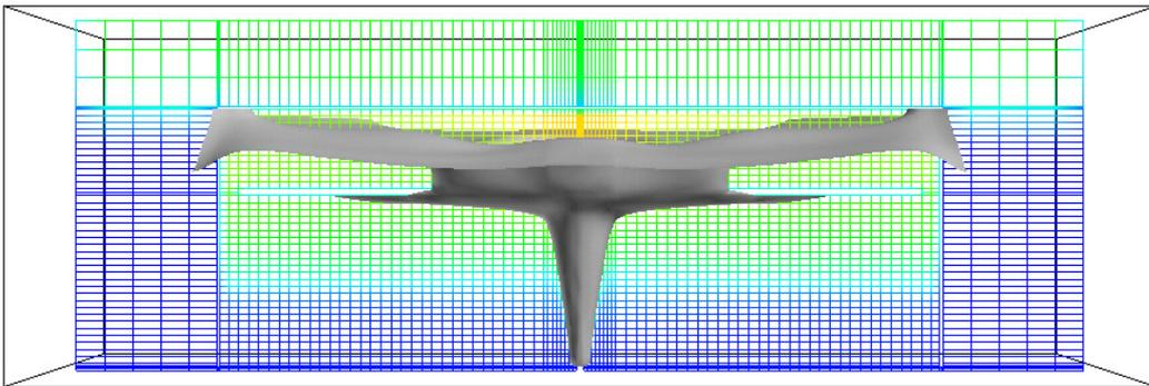
**Figure 34** 2%/m seen from the staircase after 6 minutes. The simulation was made using the Bill and Nam turbulence coefficients; the source had a velocity of 1.5 m/s and a temperature of 340 K.
