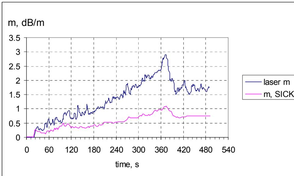
Figure 30 Smoke obscuration measured using a diode laser and the SICK for test SG3003.
