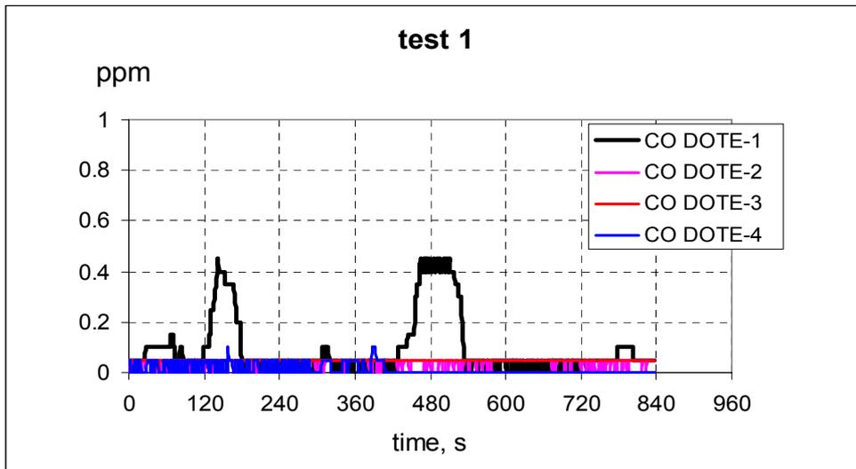
Figure 5 CO signals from the DOTEs, test1.
