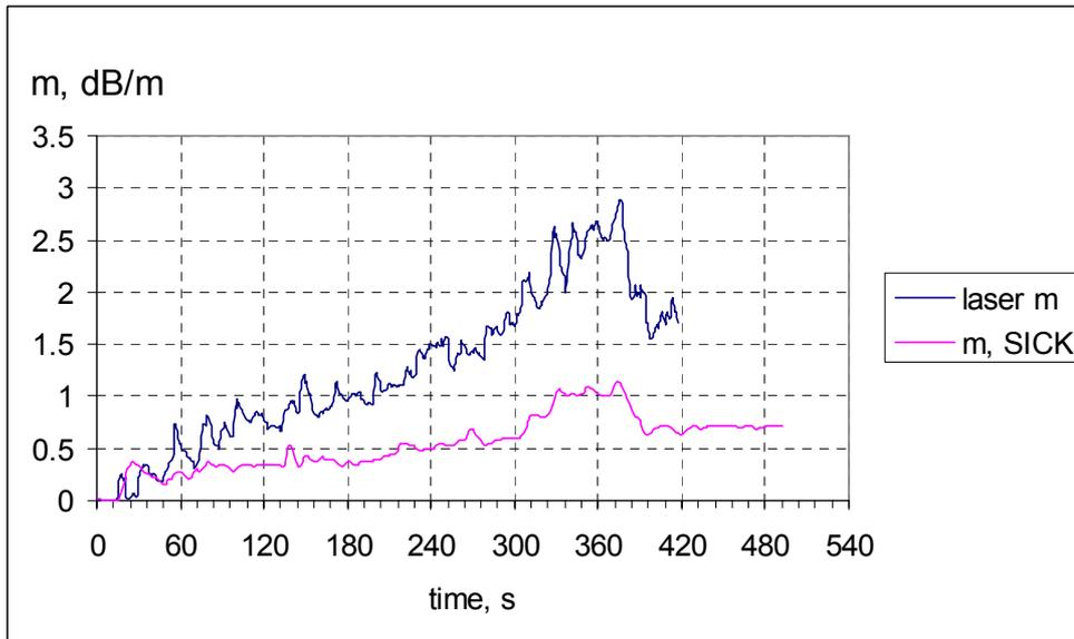
Figure 29 Smoke obscuration measured using a diode laser and the SICK for test SG3002.
