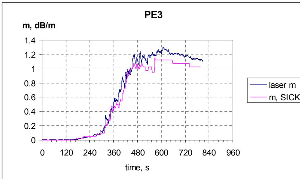
Figure 41 Smoke obscuration measured using a diode laser and the SICK for test PE3.
