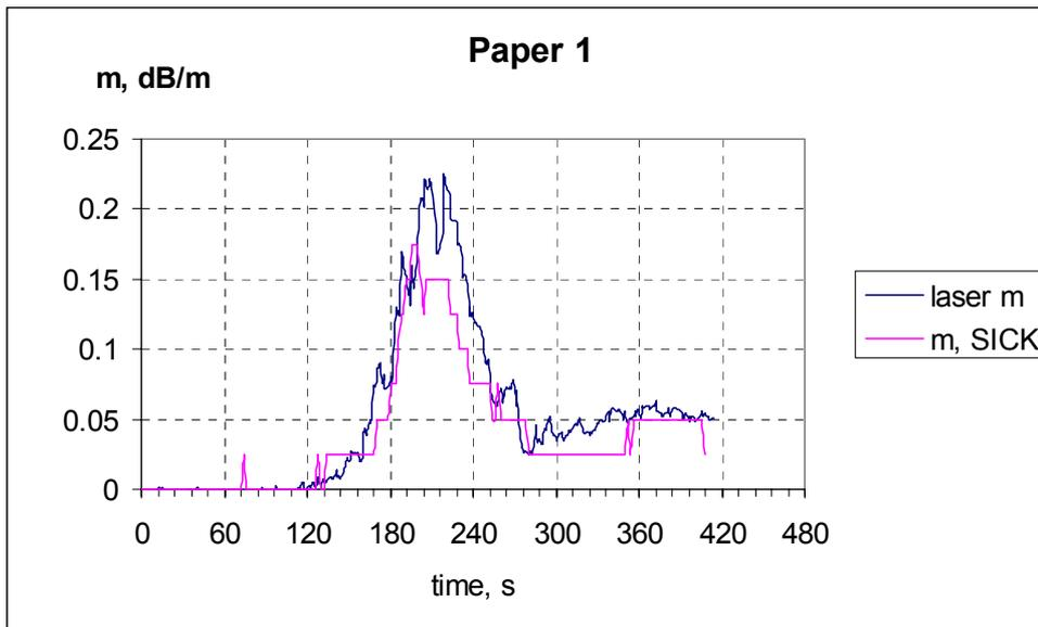
Figure 32 Smoke obscuration measured using a diode laser and the SICK for test Paper1.
