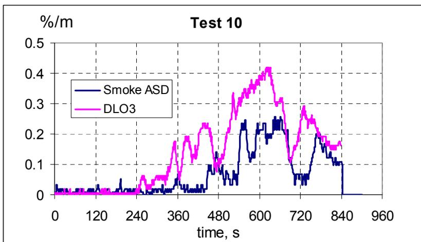
Figure 69 Comparison between the sampling system and the nearby beam detector, test 10.
