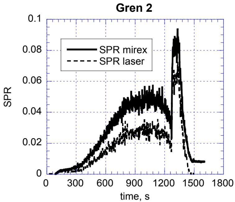
Figure 15 Comparison of SPR obtained by the MIREX and the cone calorimeter for test Gren2.
