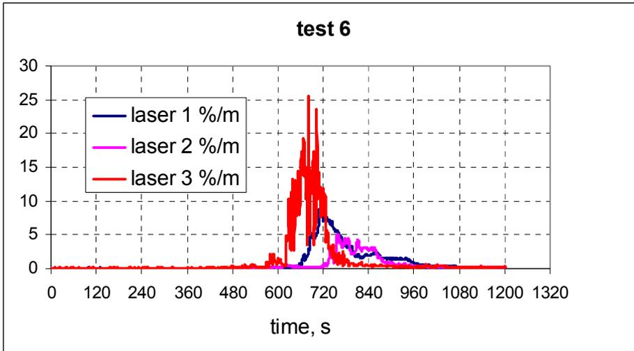
Figure 37 Smoke signals lasers, test6.
