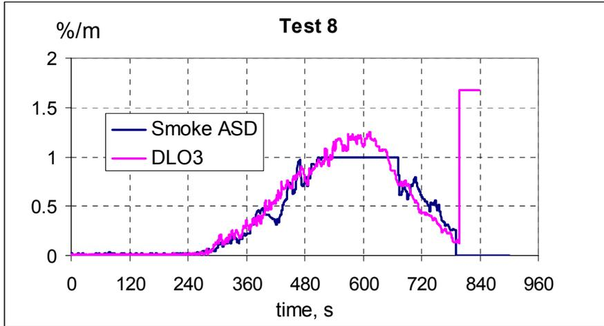
Figure 55 Comparison between sampling system and the beam detector nearby, test8.
