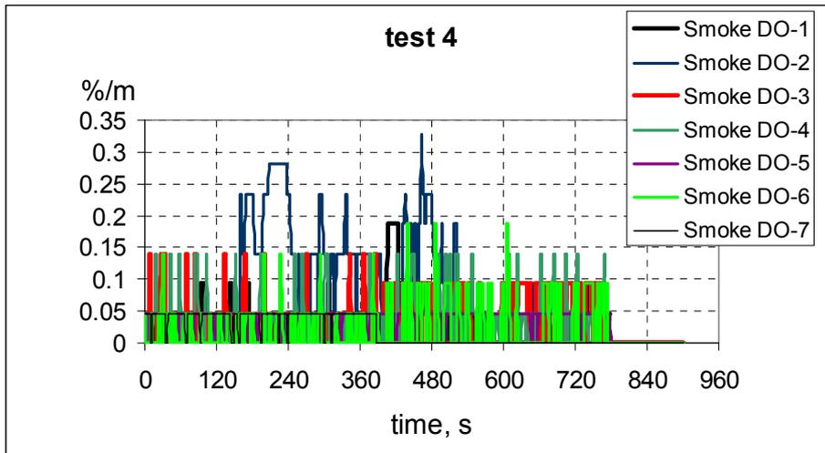
**Figure 22** Smoke signals from detector 1-7, test4.
