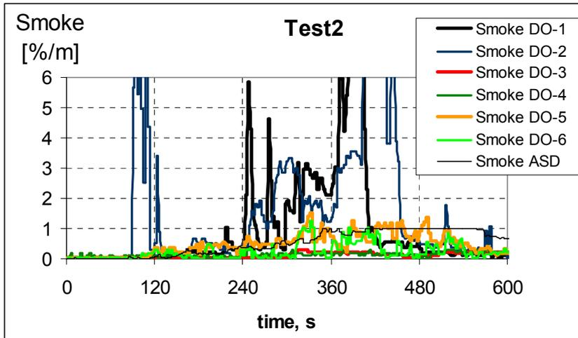
Figure 3 Smoke signals from detector 1-6 and ASD, test 2.
