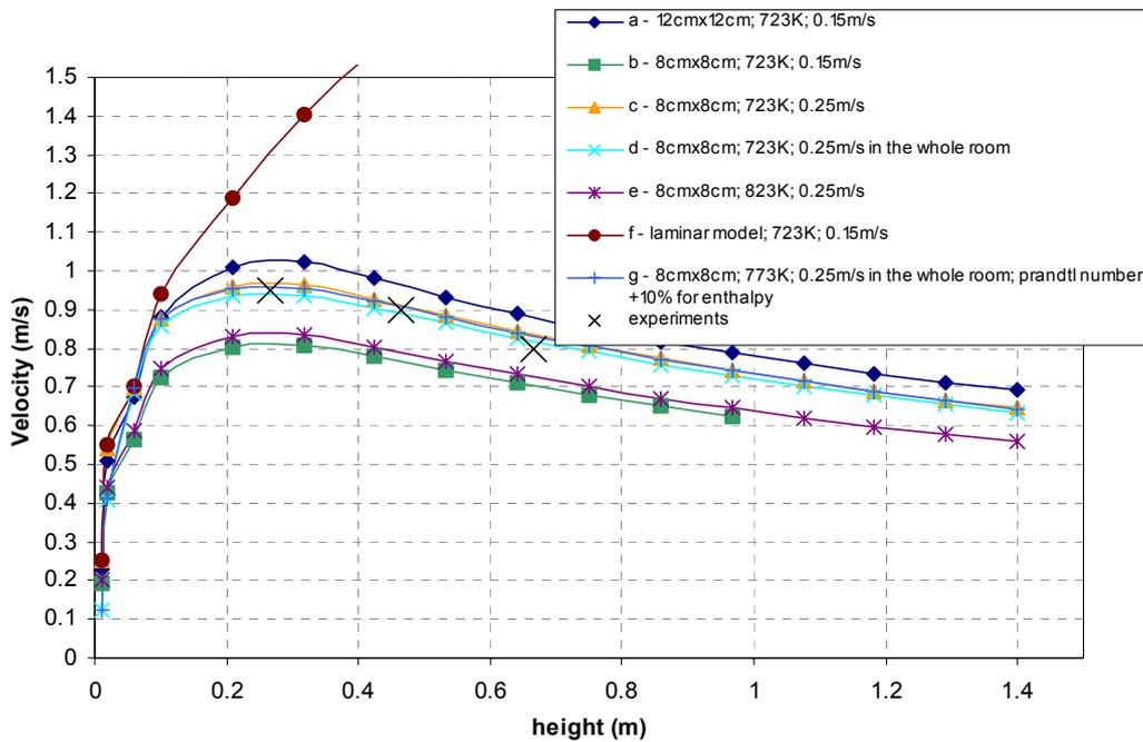
**Figure 10** Velocity profile above the smoke source
