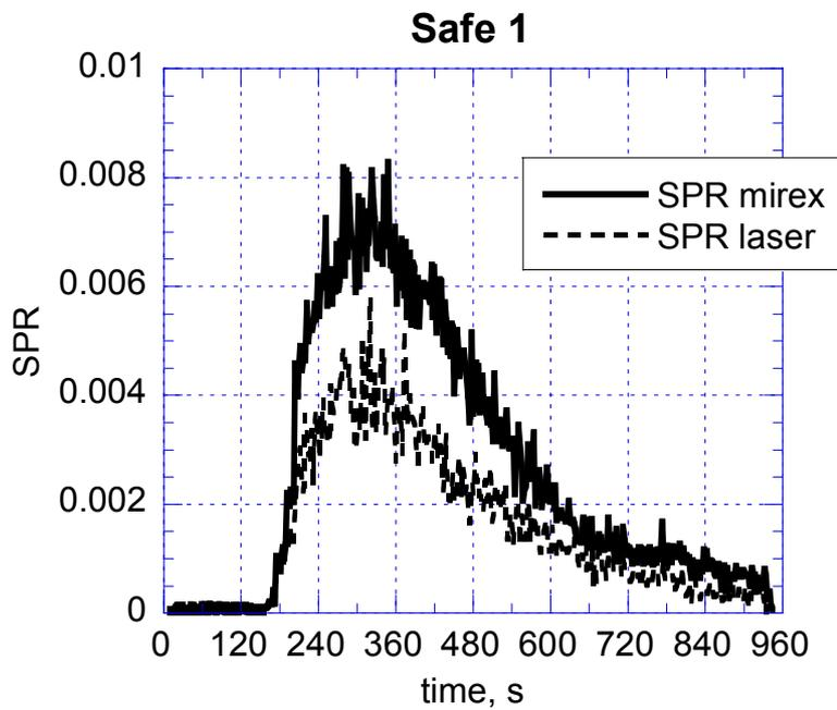
Figure 12 Comparison of SPR obtained by the MIREX and the cone calorimeter for test Safe1.
