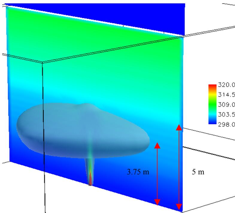
**Figure 13** Smoke profile after 10 minutes in the 1 °C/m case.
