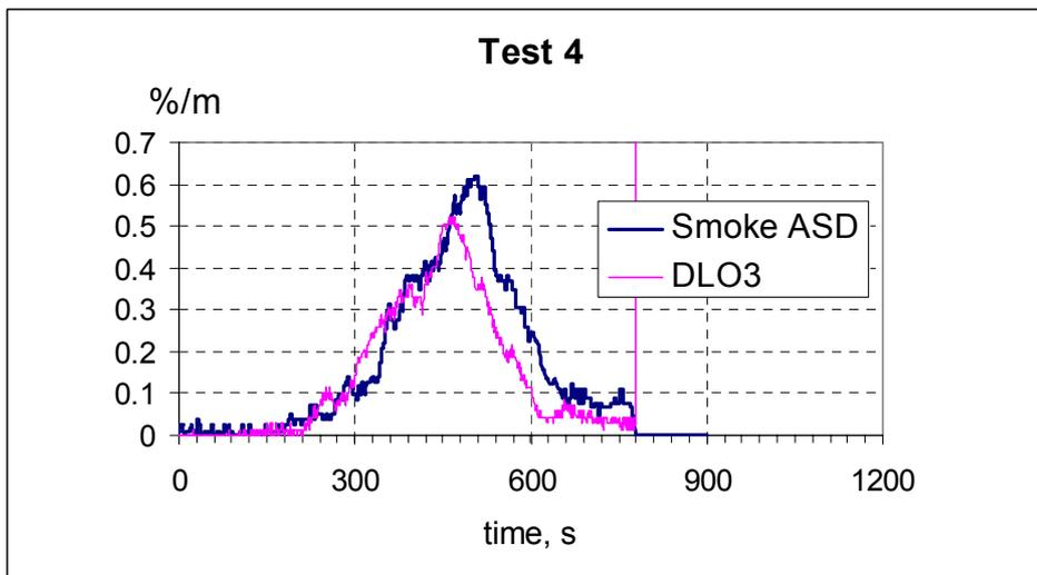
Figure 27 Comparison between sampling system and the beam detector in the vicinity.
