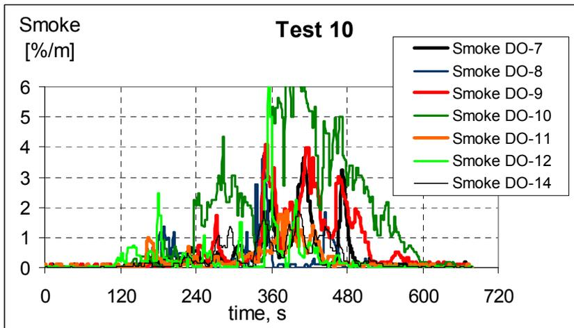
**Figure 20** Smoke signals detector 7-14, test 10.
