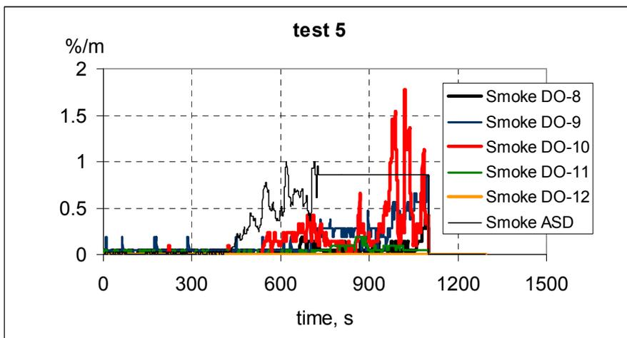
Figure 29 Smoke signals from detectors 8-12 and ASD, test 5.
