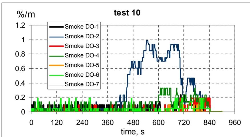
Figure 63 Smoke signals from detector 1-7, test 10.
