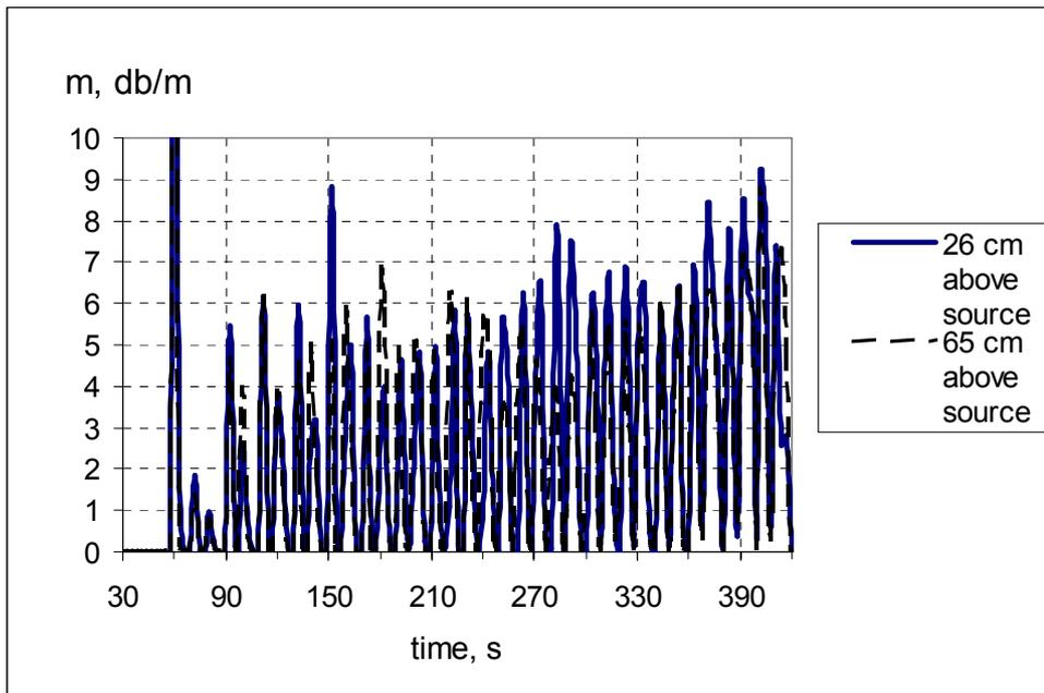
**Figure 26** Smoke obscuration measured at different heights above the SG3000. The cyclic behaviour of the SG3000 is clearly seen. No difference between different heights can be observed, which means that the measuring laser covers the entire plume at the different heights.
