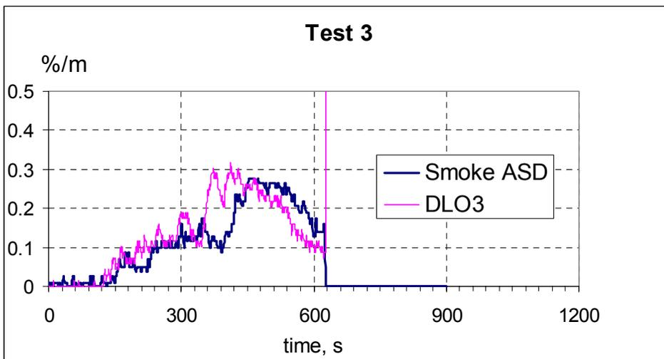
Figure 21 Comparison between the sampling system and the beam detector in the vicinity.
