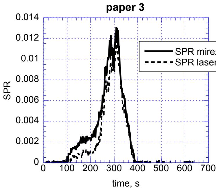
Figure 4 Comparison of SPR (Smoke Production Rate) obtained by the MIREX and the cone calorimeter for test Paper3.
