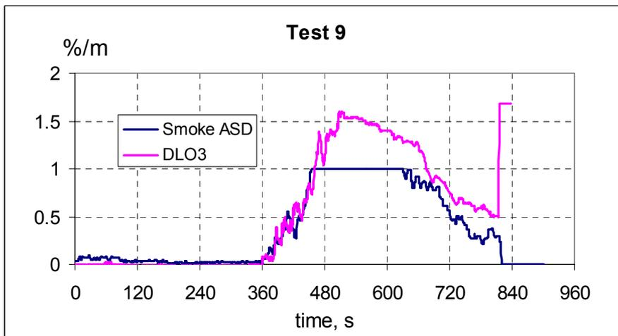
Figure 62 Comparison between sampling system and the beam detector nearby.
