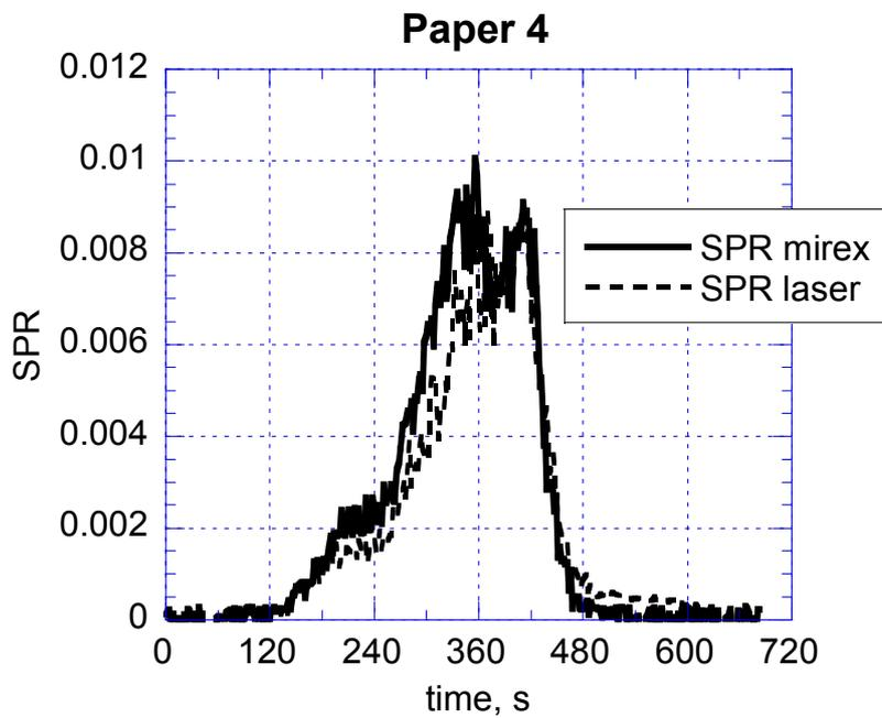
Figure 8 Comparison of SPR obtained by the MIREX and the cone calorimeter for test Paper4.
