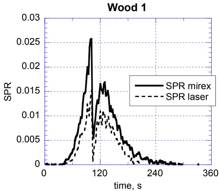
Figure 21 Comparison of SPR obtained by the MIREX and the cone calorimeter for test Wood1.
