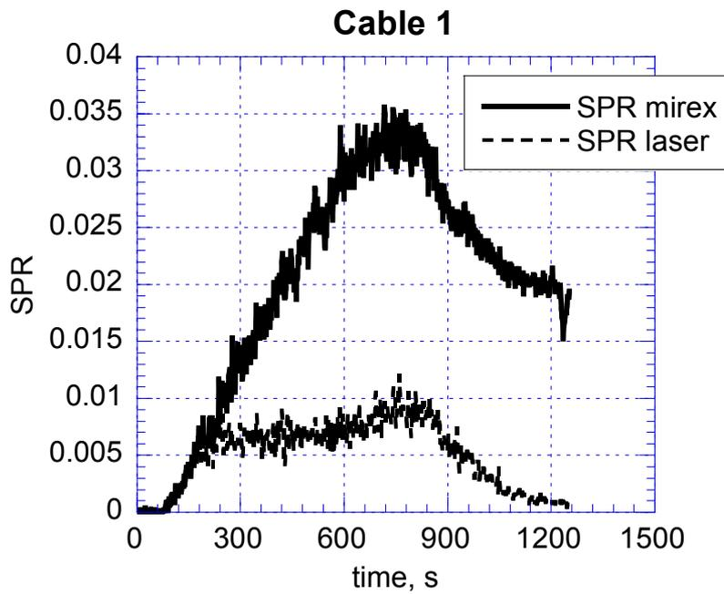
Figure 17 Comparison of SPR obtained by the MIREX and the cone calorimeter for test Cable1.
