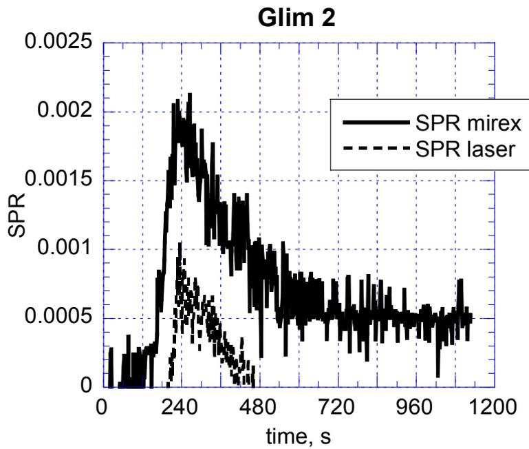
Figure 11 Comparison of SPR obtained by the MIREX and the cone calorimeter for test Lighter2.
