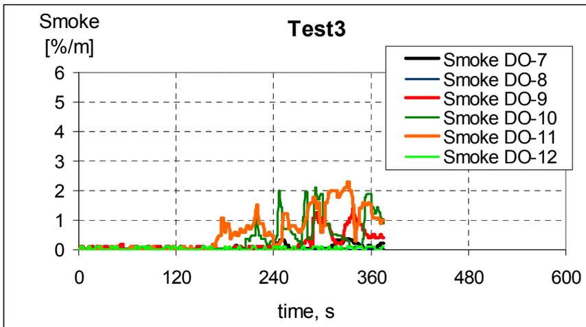
Figure 7 Smoke signals from detector 7-12 test 3.
