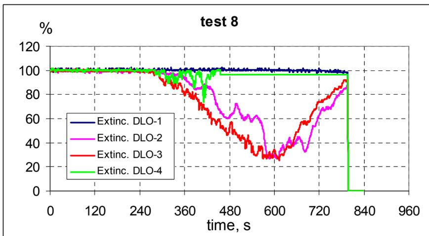
Figure 54 Smoke signals from beam detectors, test8.
