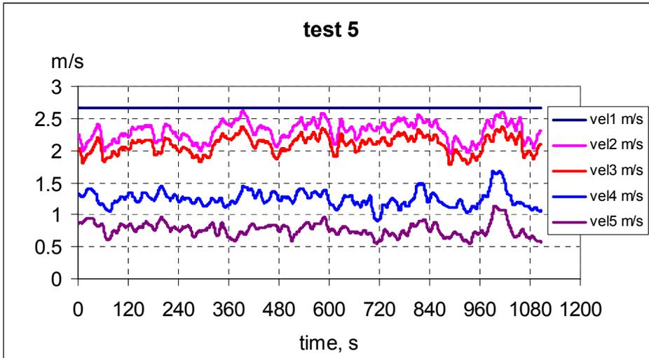
Figure 73 Velocity below an air inlet test5.
