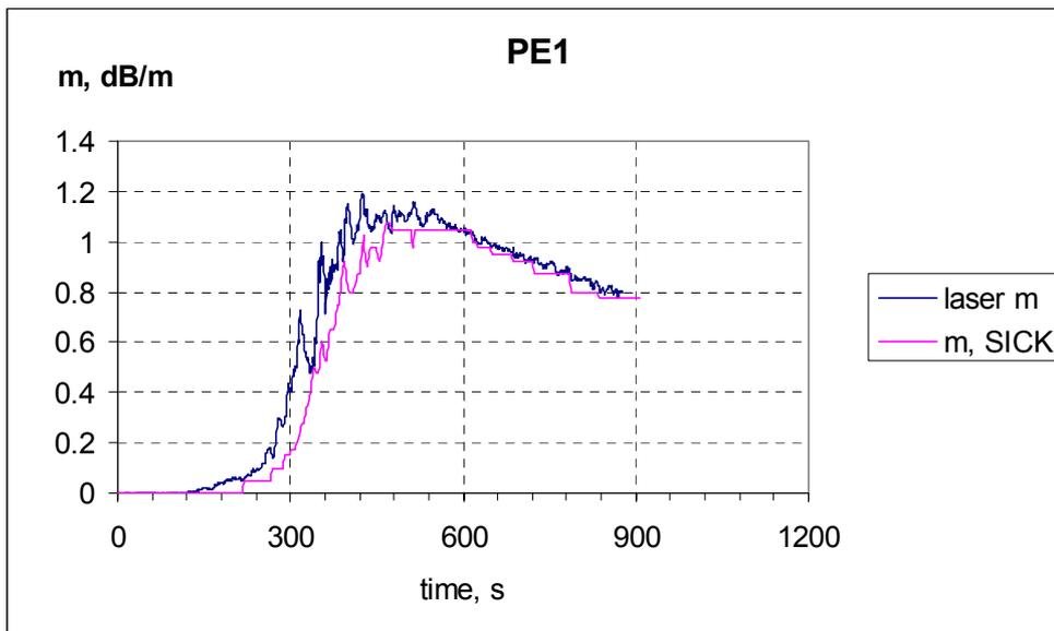
Figure 39 Smoke obscuration measured using a diode laser and the SICK for test PE1.
