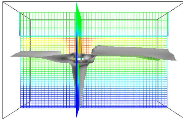
**Figure 28** The 1%/m isocurve seen from the reception after 6 minutes using the normal k- $\epsilon$  model. The smoke is slowed down by the beam but reaches the ceiling.
