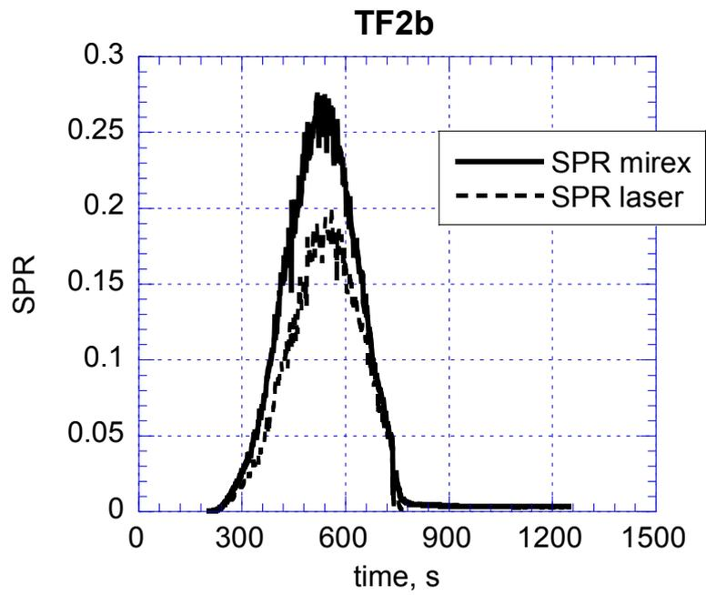
Figure 27 Comparison of SPR obtained by the MIREX and the cone calorimeter for test TF2b.
