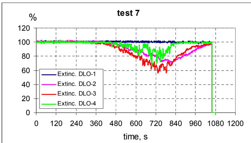
Figure 47 Smoke signals from beam detectors, test7.
