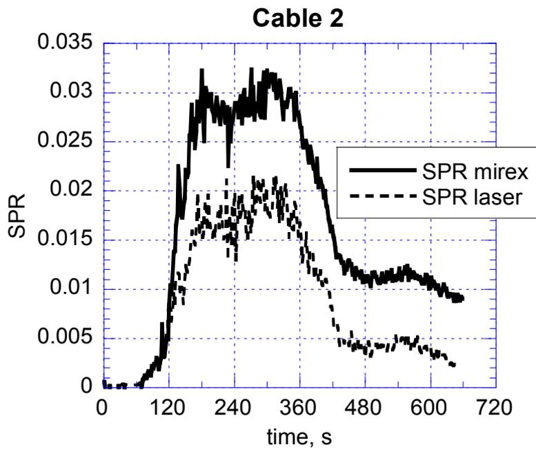
Figure 18 Comparison of SPR obtained by the MIREX and the cone calorimeter for test Cable2.
