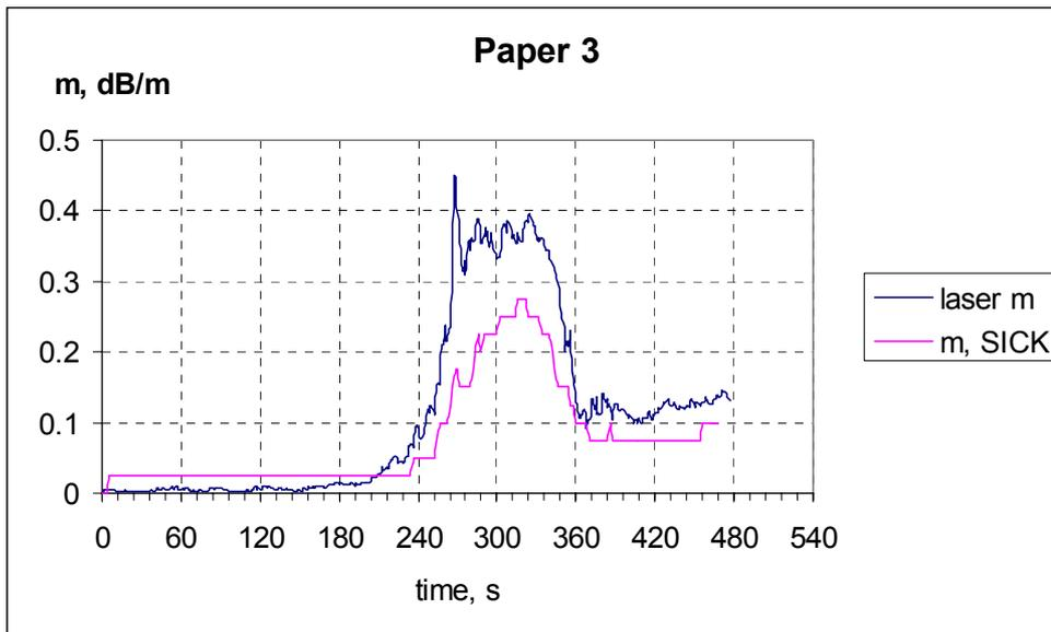
Figure 34 Smoke obscuration measured using a diode laser and the SICK for test Paper3.
