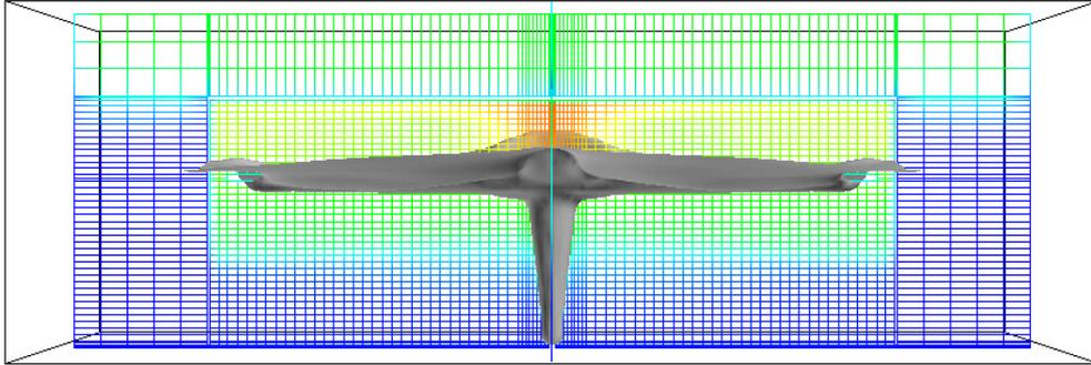
**Figure 27** The iso-curve for 1%/m seen from the staircase looking into the building after 6 minutes using the normal k- $\epsilon$  model. The smoke is slowed down by the beam but reaches the ceiling.
