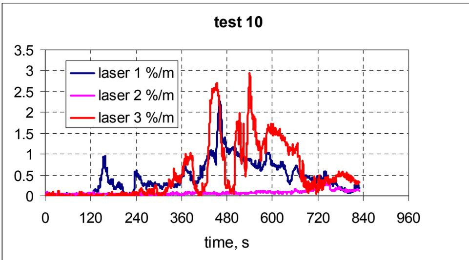
Figure 65 Smoke signals from lasers, test 10.
