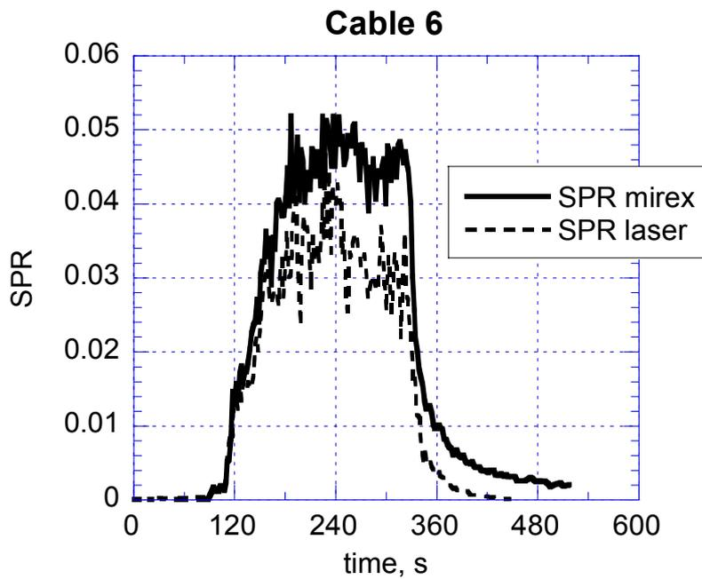
Figure 24 Comparison of SPR obtained by the MIREX and the cone calorimeter for test Cable6.
