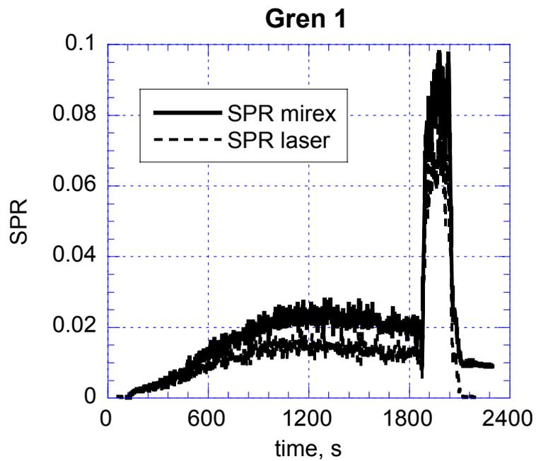
Figure 14 Comparison of SPR obtained by the MIREX and the cone calorimeter for test Gren1.
