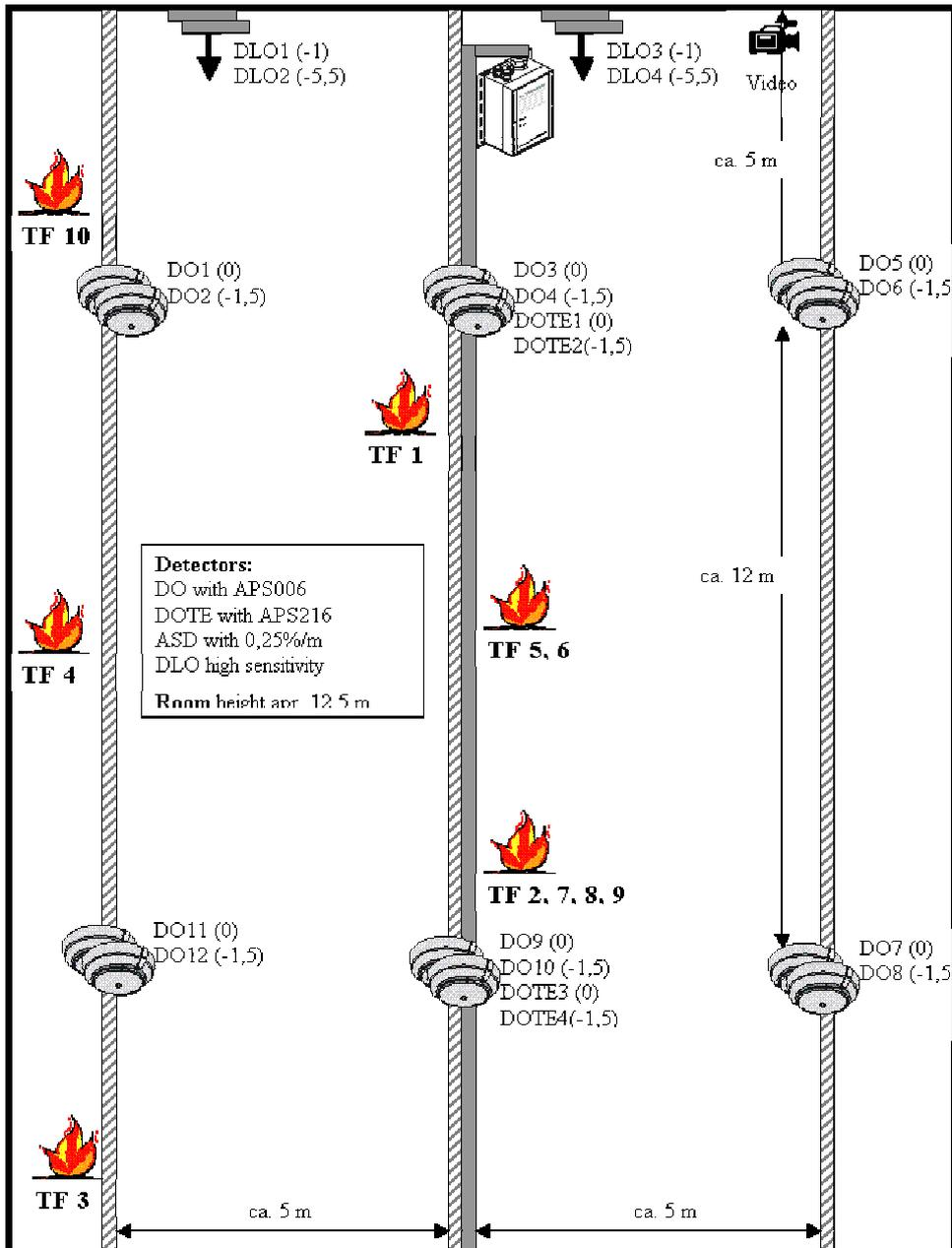
Figure 23 Schematic of detector and fire placement.
