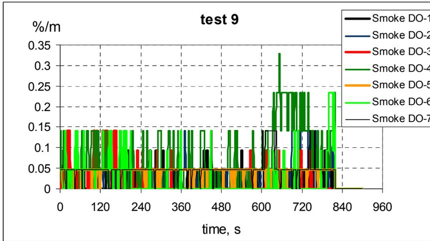
Figure 56 Smoke signals from detectors 1-7, test9.
