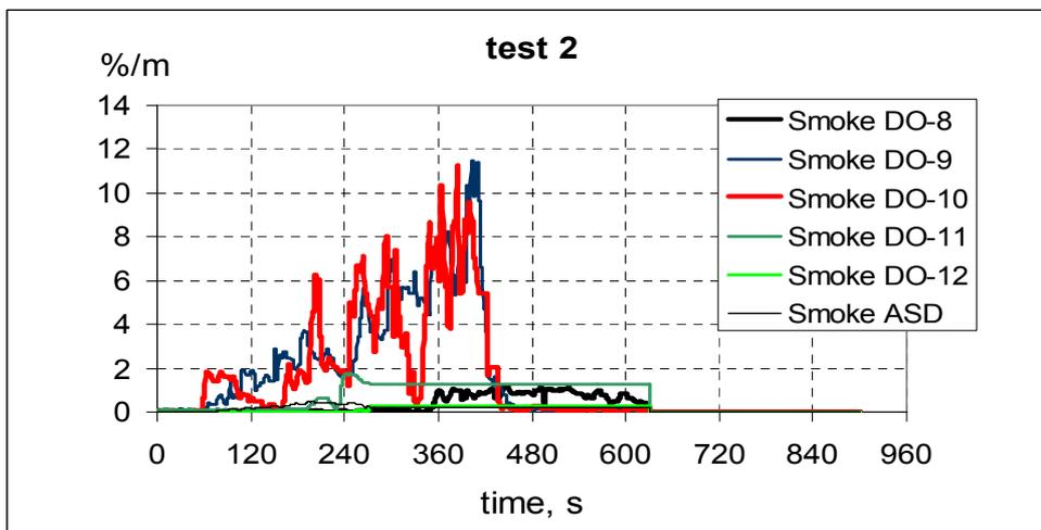
Figure 9 Smoke signals from detector 7-12 and ASD, test 2.
