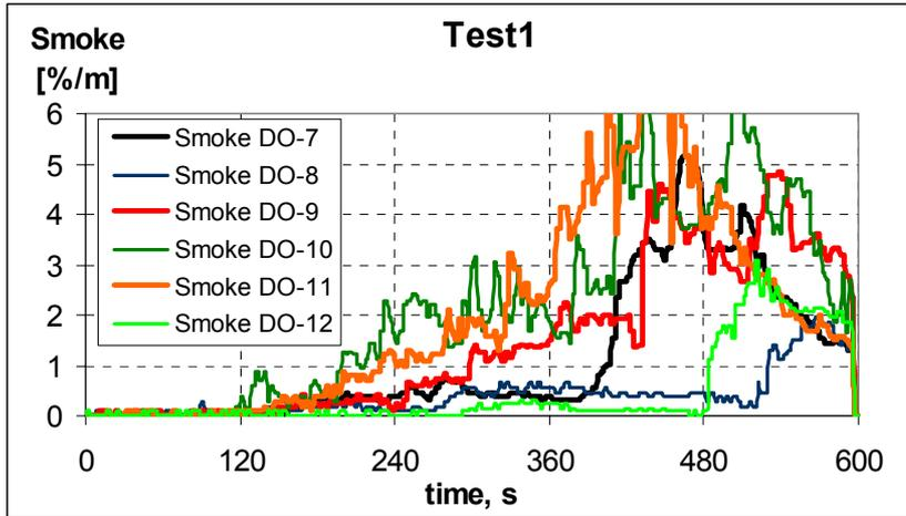
Figure 1 Smoke signal from detector 7-12 test1.
