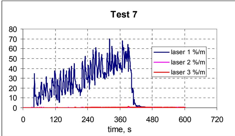
Figure 18 Smoke signals from lasers, test7.
