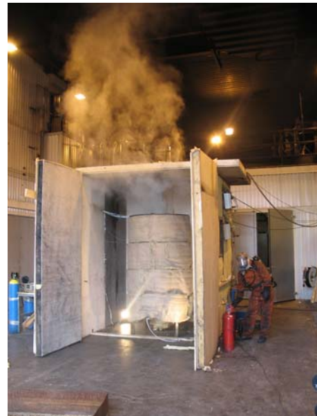
Figure 4. 1\text{m}^3 basket test (oven after the pellets had ignited spontaneously).
