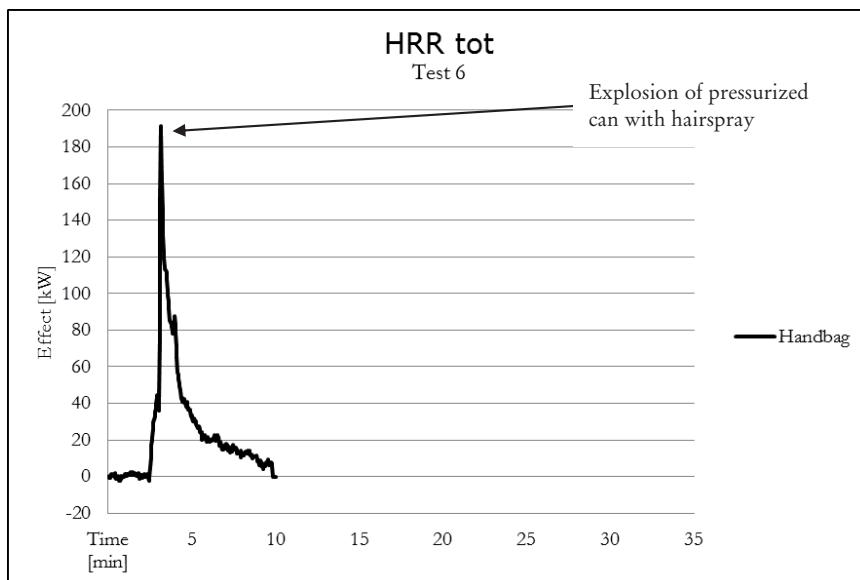
Diagram 6: Total Heat Release Rate for test 6: handbag
