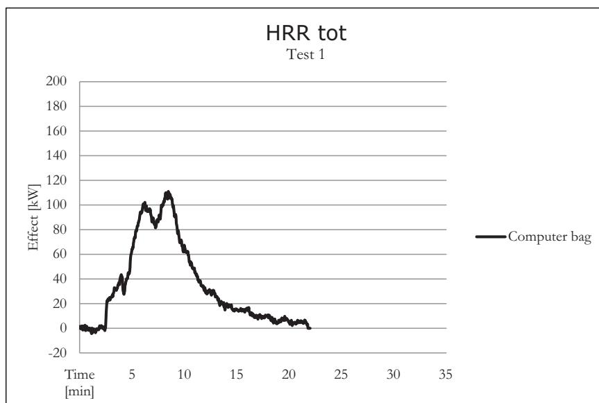
Diagram 1: Total Heat Release Rate for test 1: computer bag
