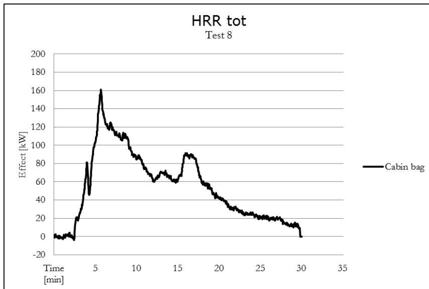
Diagram 8: Total Heat Release Rate for test 8: cabin bag
