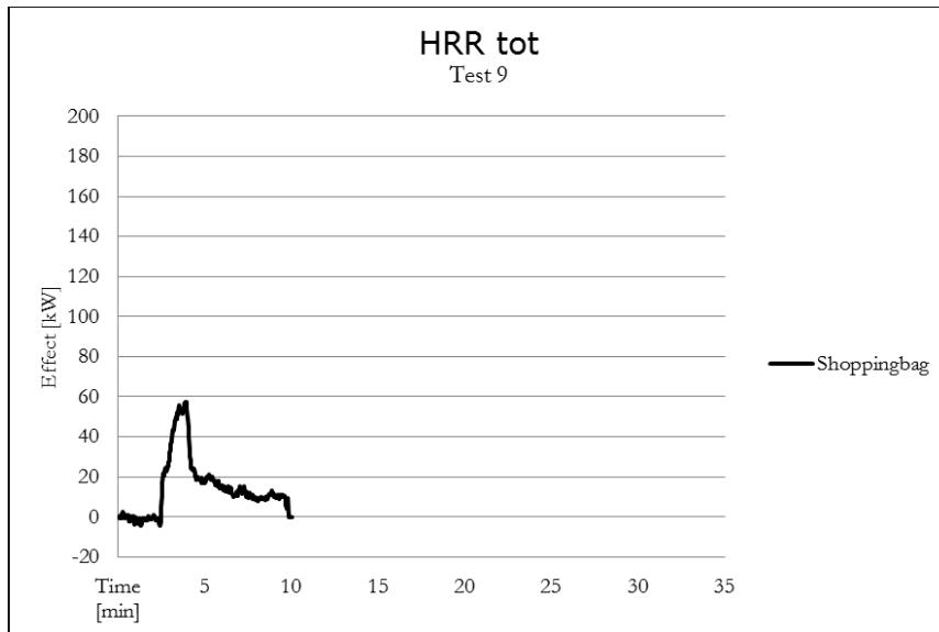
Diagram 9: Total Heat Release Rate for test 9: shopping bag
