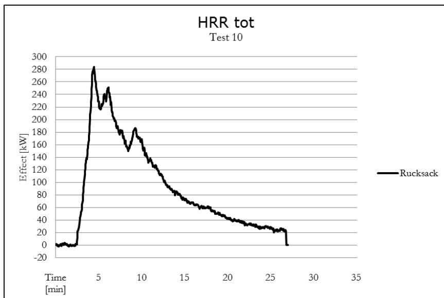
Diagram 10: Total Heat Release Rate for test 10: rucksack
