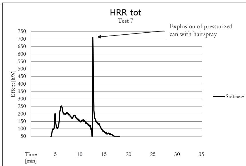
Diagram 7: Total Heat Release Rate for test 7: suitcase
