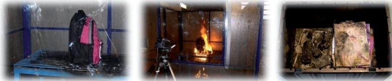
**Pictures 14–16:** From test 4 (bag, fire test and remainders).
