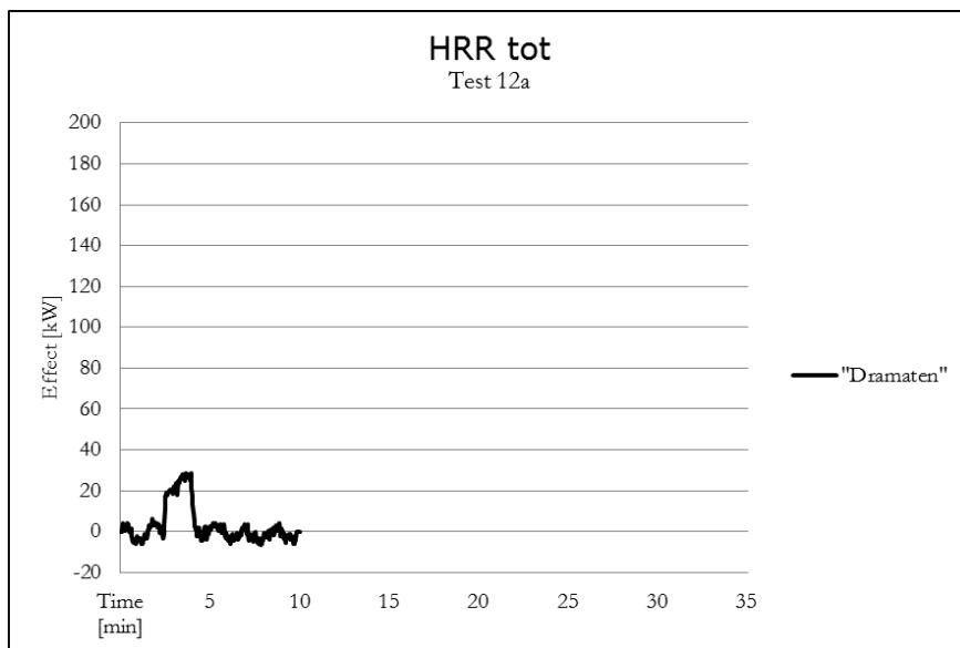
Diagram 12: Total Heat Release Rate for test 12a: trolley bag
