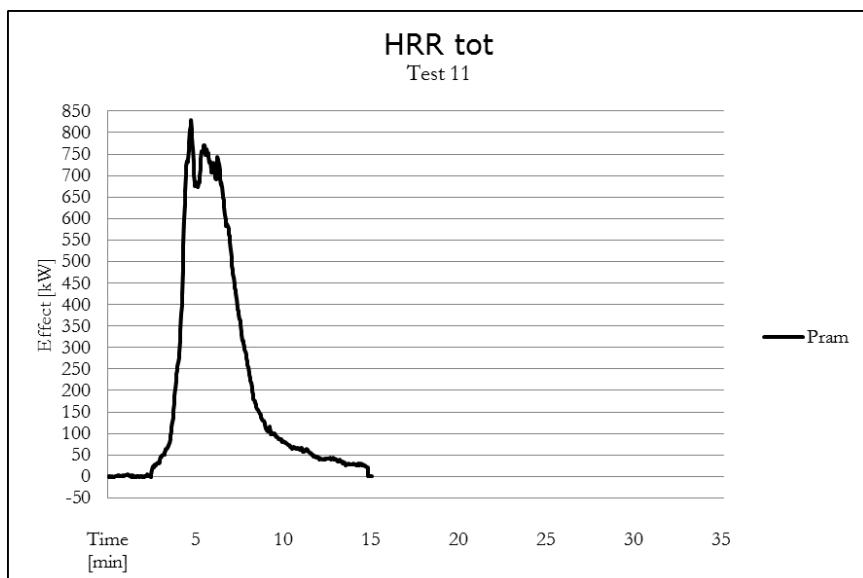
Diagram 11: Total Heat Release Rate for test 11: pram
