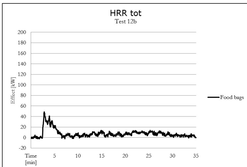
Diagram 13: Total Heat Release Rate for test 12b: food bags
