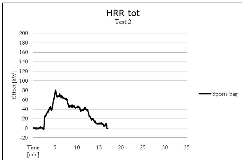
Diagram 2: Total Heat Release Rate for test 2: sports bag
