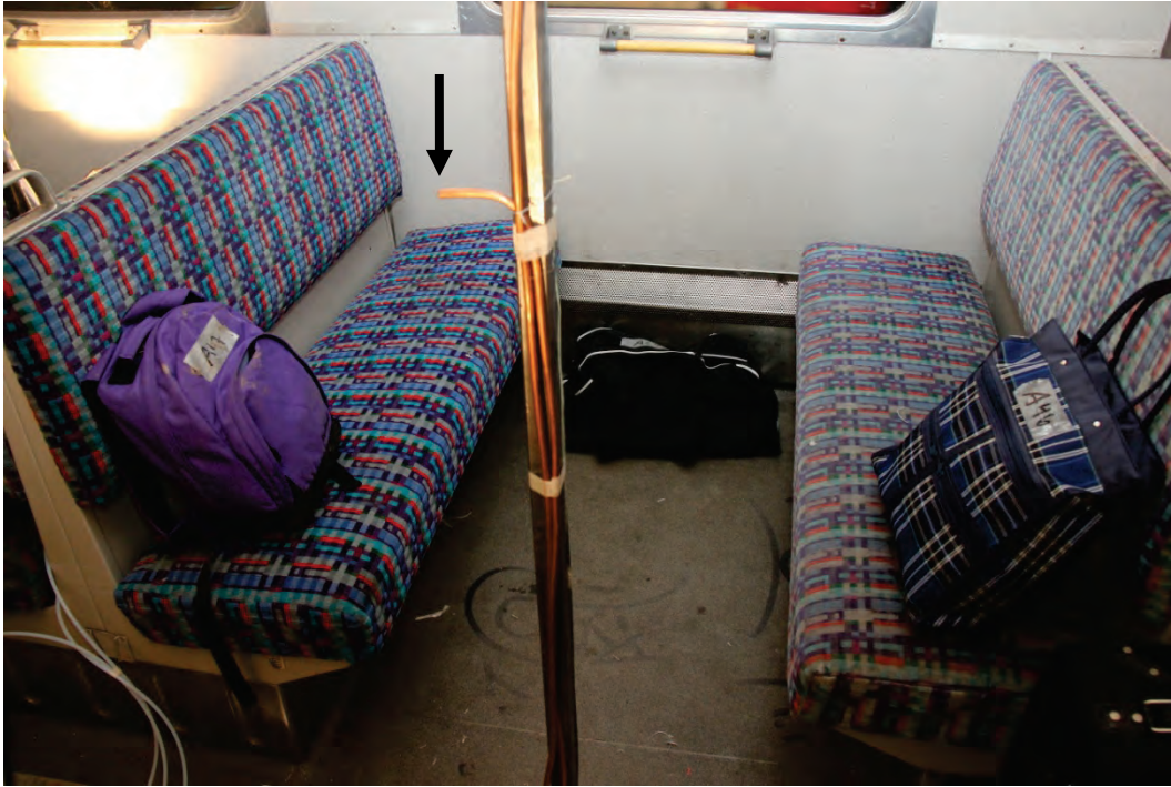
Figure 6.5 Inlet pipe for the gas sampling inside the railway carriage.
