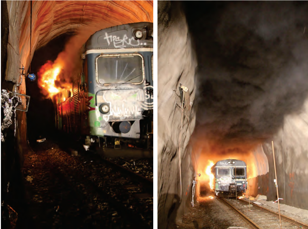
Figure A4.7 Left picture: Flames from the windows on the left side of the carriage approx. 4 min after ignition. (Photo: Per Rohlén) Right picture: Flames from the carriage approx. 7 min after ignition. The backlayering can be seen in the ceiling of the tunnel. (Photo: Per Rohlén)
