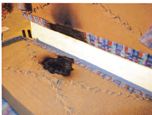
Photo 9 - After test. Some charring is visible around the area where the burner was applied as well as on the lower part of the back.
