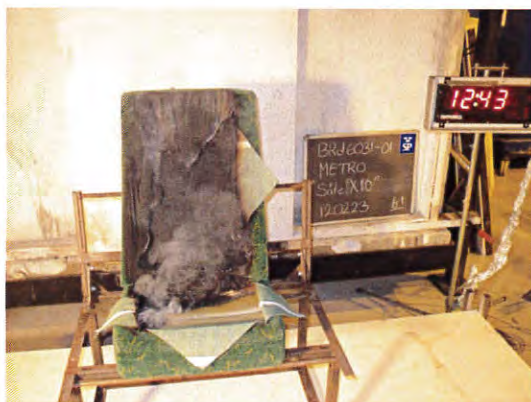
Photo 9 - Time 12:43. The flames on the seat cease.
