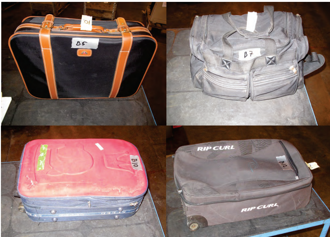
Figure A4.27 Examples of middle sized bags used in test 3, each with a total mass of 10 kg.
