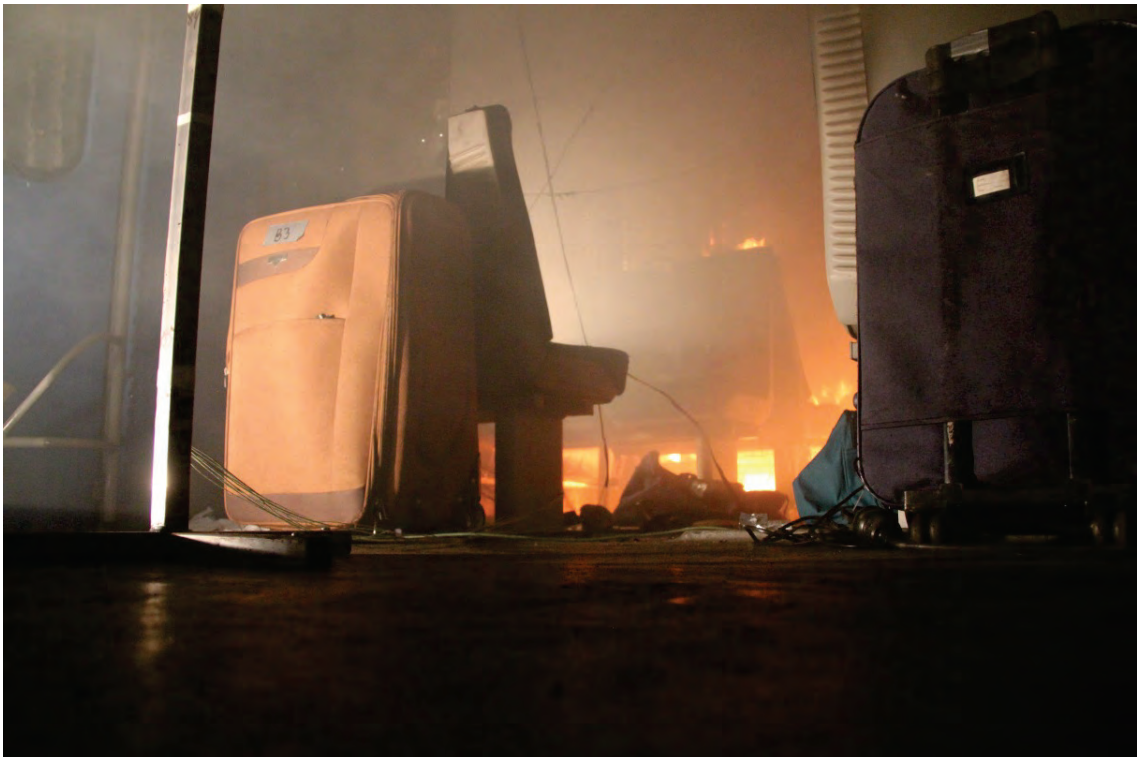
Figure A4.14 There was a long fire growth period in test 3. This picture is taken approx. 40 min after ignition and the fire has still not spread any further than between the seats were it was lit. (Photo: Per Rohlén)
