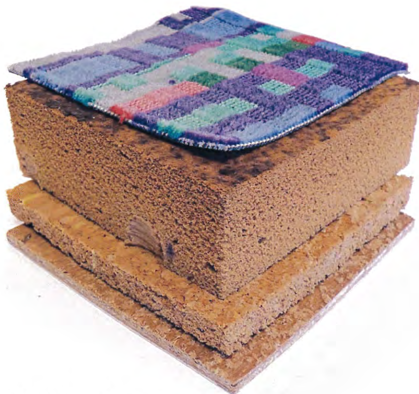
Photo 5 - "X1", material composition of passenger seat
