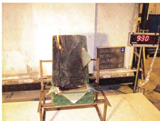
Photo 7 - Time 09:30. The Velcro is burning on the back underneath the pendant piece of fabric.
