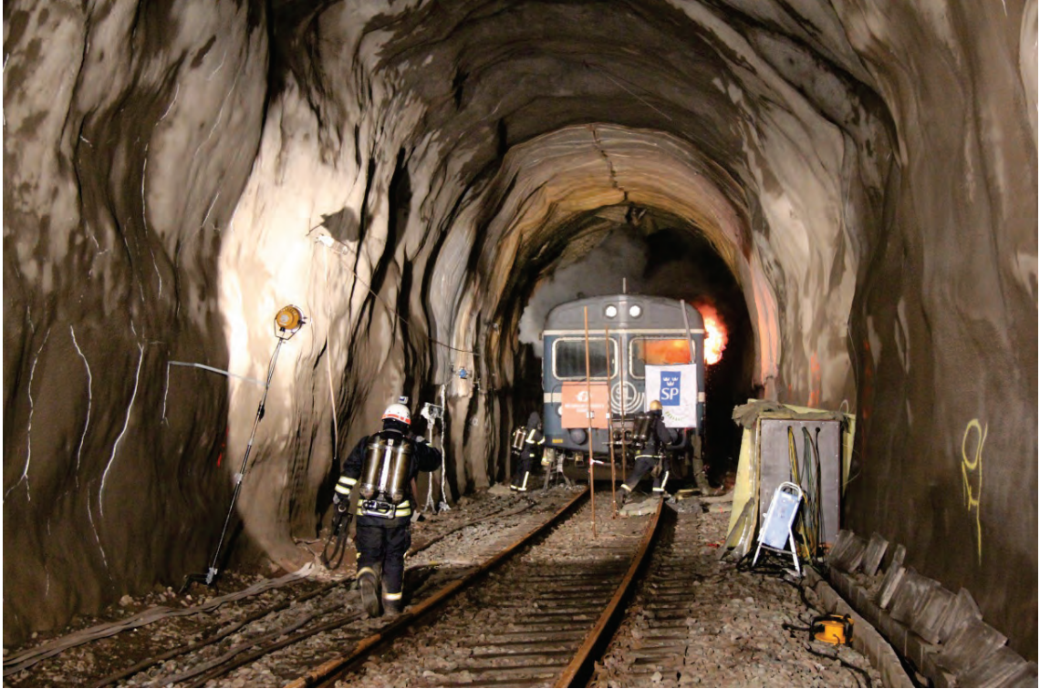
Figure A4.15 This picture shows the first flames outside of the carriage, the picture is taken approx. 1 h 50 min after ignition. In contrast to test 2 the first flames exit from the driver compartment. (Photo: Per Rohlén)
