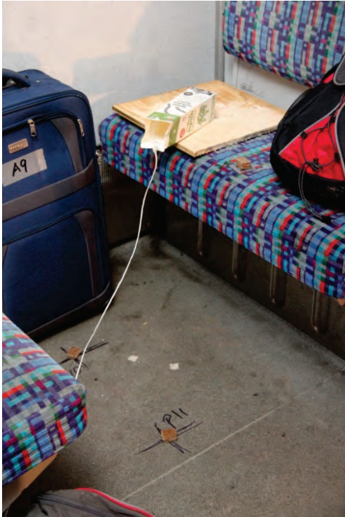
Figure A4.4 The ignition set up in test 2. The milk cartridge was filled with one liter of petrol and the three small fiber board pieces was lit. The petrol was ignited by pulling the string (Photo: Per Rohlén)
