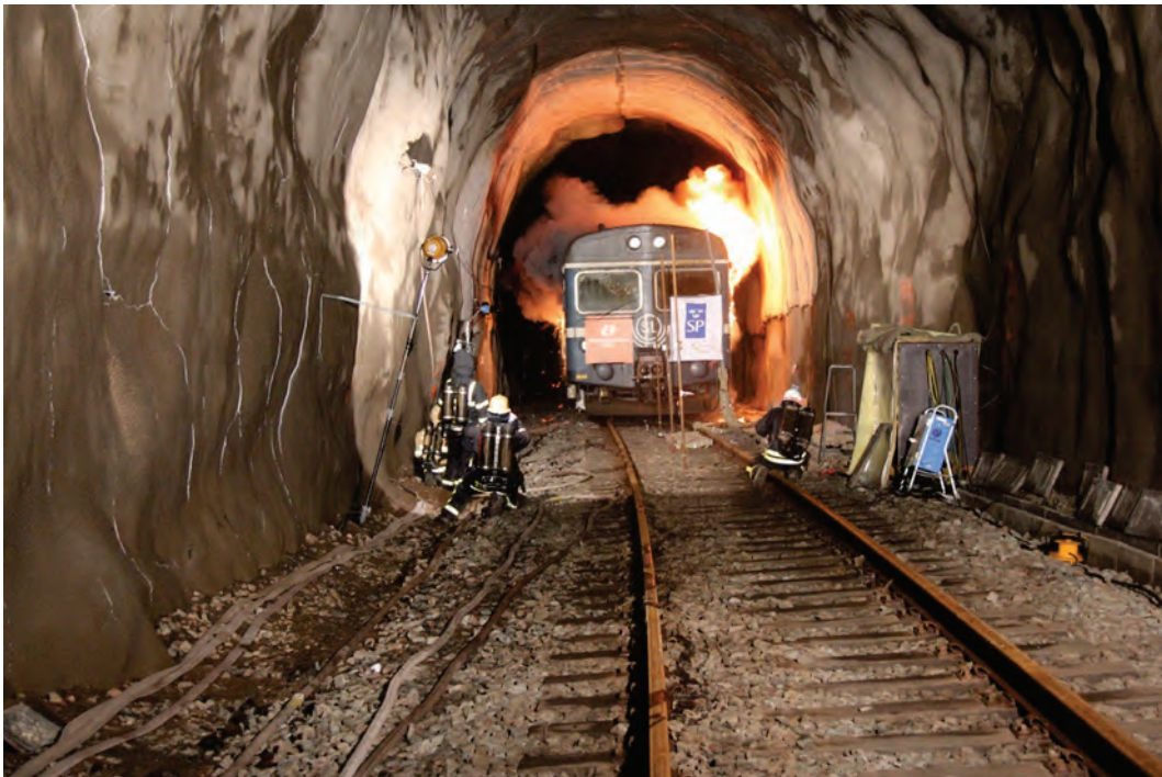
Figure A4.16 Flames from the carriage approx. 1h 55 min after ignition (Photo: Per Rohlén)
