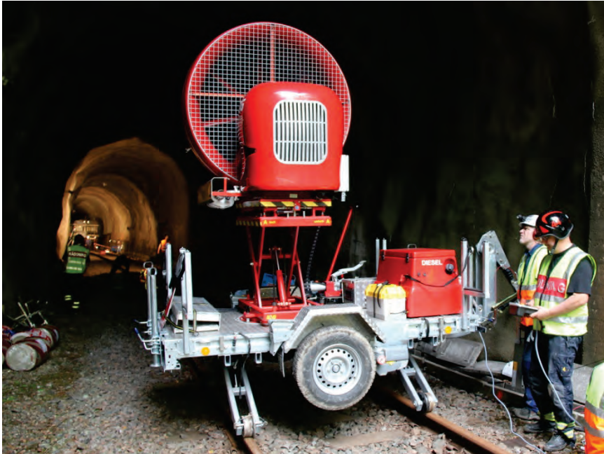
Figure 4.4 The fan was positioned 4 m into the tunnel from the eastern tunnel entrance. (Photo: Per Rohlén)
