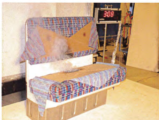
Photo 5 - Time 03:08. The flames cease but progressive smouldering is visible.
