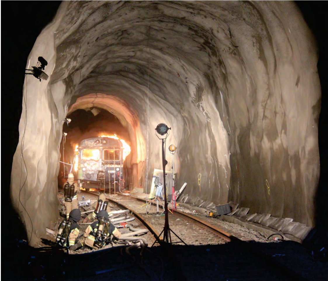
Figure A4.9 Flames from the carriage approx. 45 min after ignition, the driver compartment is now on fire and the right window is broken. (Photo: Per Rohlén)
