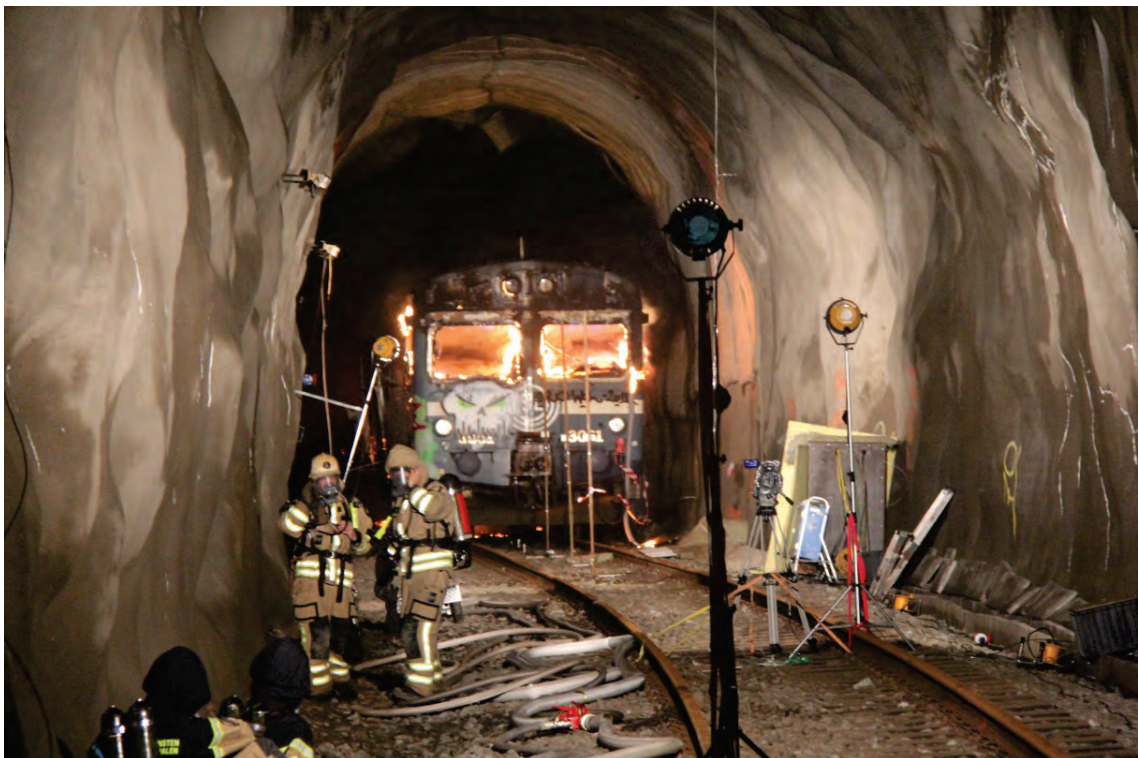
Figure A4.10 The flames from the carriage in the beginning of the decay period. The picture is taken approx. 50 min after ignition. (Photo: Per Rohlén)
