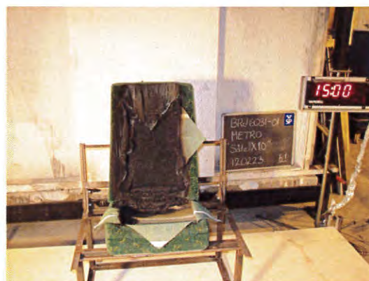
Photo 10 - Time 15:00. The smoke production has stopped.
