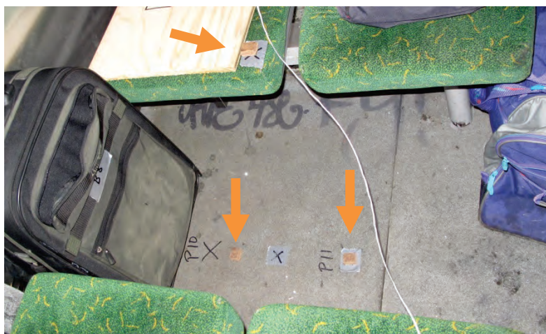
Figure 7.1 Positions of the fibre board pieces used to ignite the petrol.
