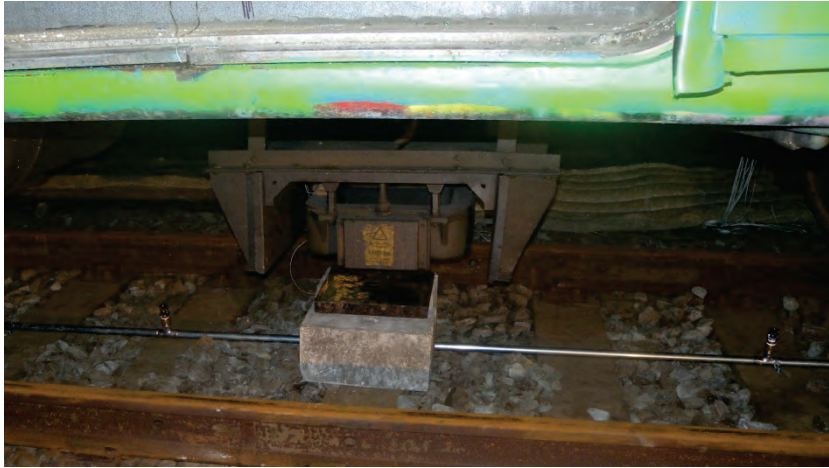
Figure 4.5 Position of the heptane pan in test 1.
