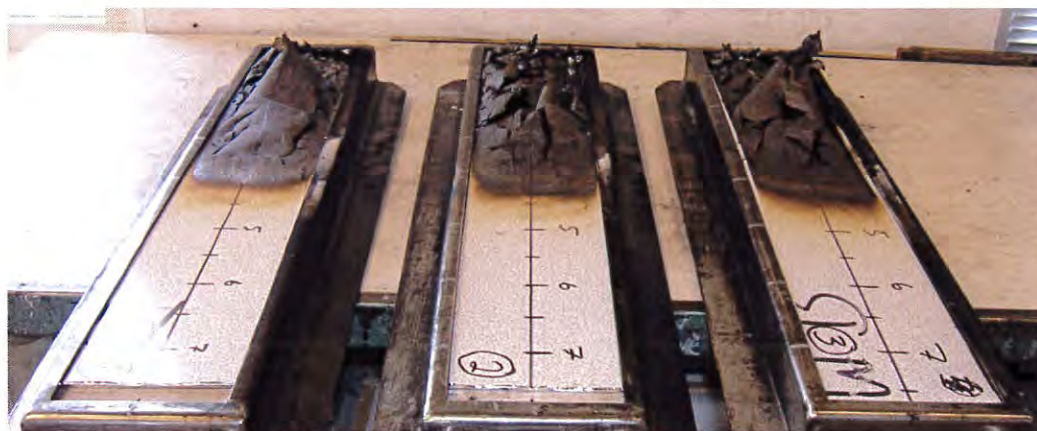
Photo 12 - All three of the tested specimens, no difference detected between specimens with or without insulation layer behind the laminate layer.
