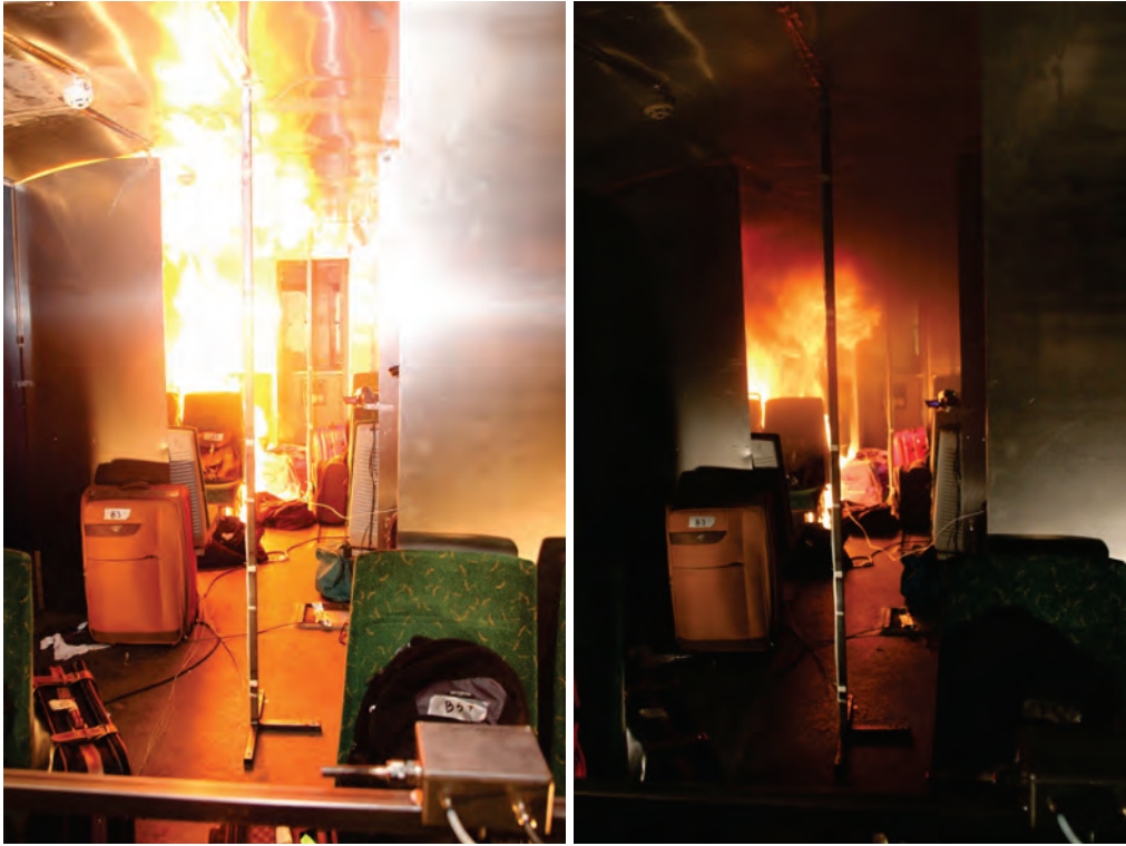
Figure A4.13 Left picture: Picture from inside the carriage shortly after ignition. (Photo: Per Rohlén) Right picture: The fire has started to spread from the ignition source to the surrounding bags, picture is taken approx. 1 – 2 min after ignition. (Photo: Per Rohlén)
