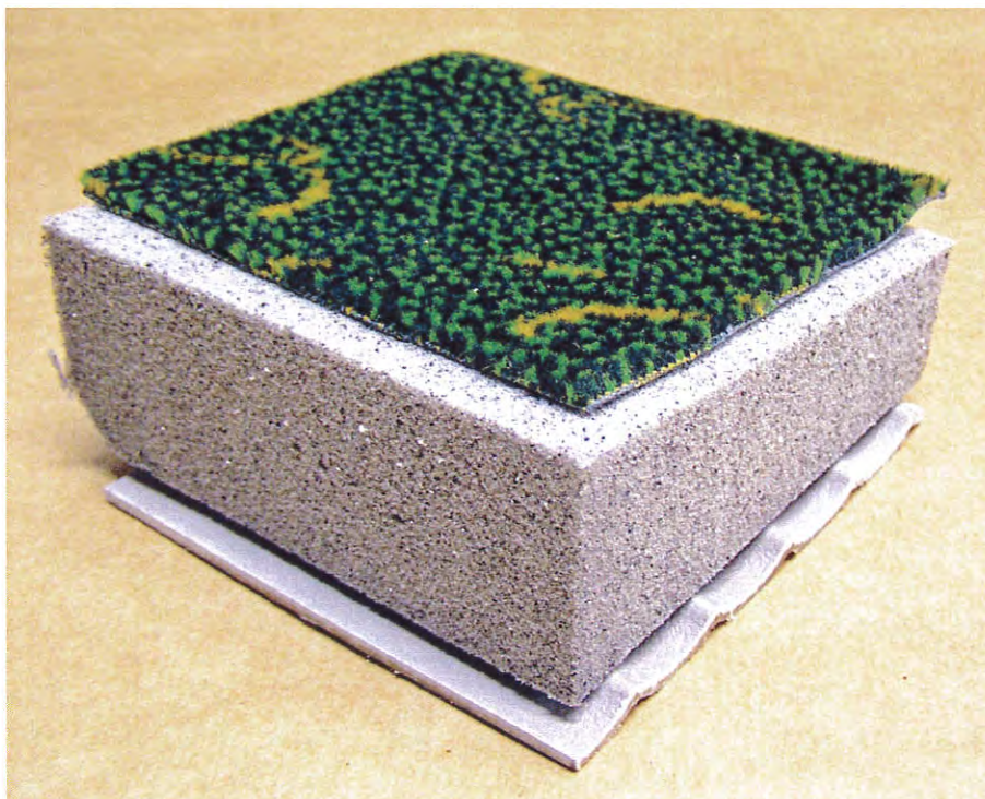
Photo 8 – "C20/X10", Upholstery, material composition of passenger seat*
