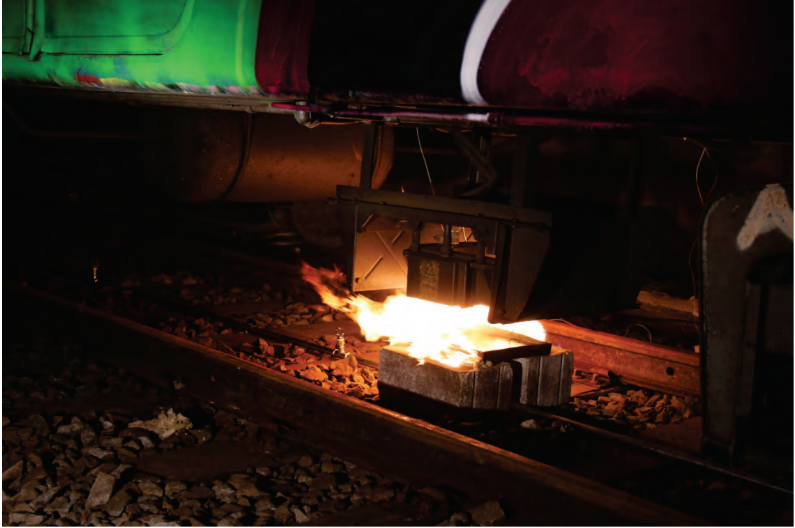
Figure A4.1 Flames from the heptane pool shortly after ignition in test 1.(Photo: Per Rohlén)
