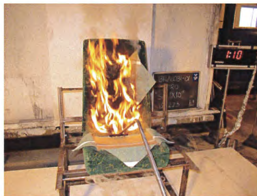
Photo 4 - Time 01:10. All of the exposed foam is burning with large flames and thick, green smoke is coming out from under the seat.
