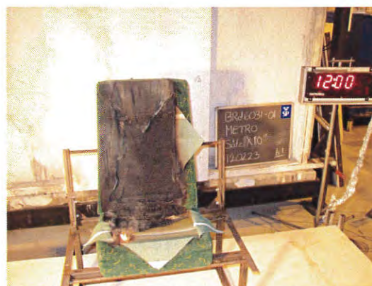
Photo 8 - Time 12:00. The flames on the backrest cease.
