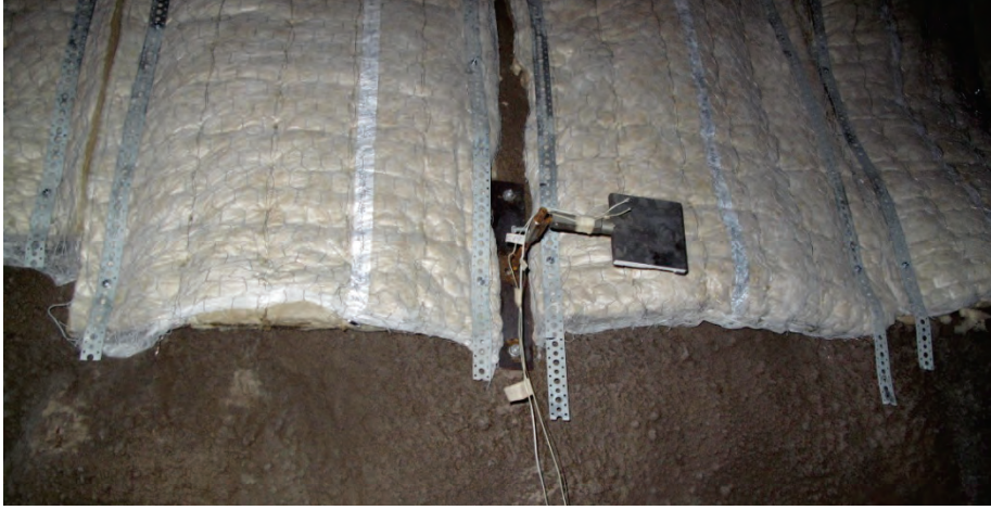
Figure 6.4 Plate thermometer mounted on the wall to measure the radiation from the fire in the carriage.
