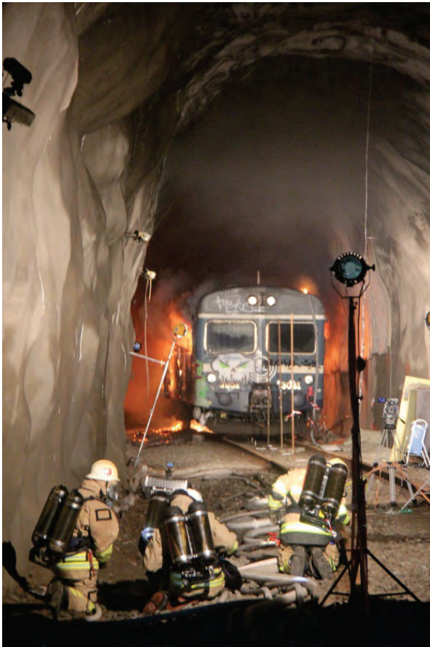
Figure A4.8 Flames from the carriage approx. 20 min after ignition. Most of the carriage is now on fire but the driver compartment is still intact. (Photo: Per Rohlén)
