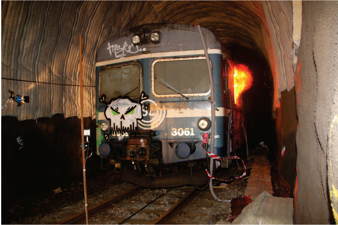
Figure A4.6 Flames from the windows on the right side of the carriage approx. 4 min after ignition. (Photo: Per Rohlén)
