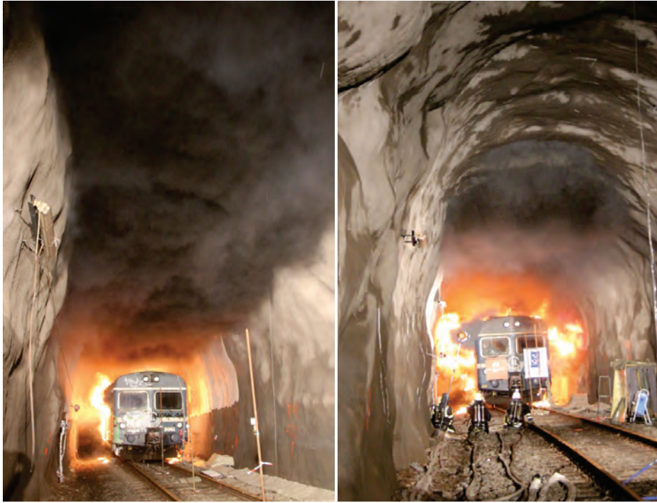
Figure 8.3 Developed backlayering in test 2 (left) and large flames and progressing backlayering in test 3 (right). (Photo: Per Rohlén)
