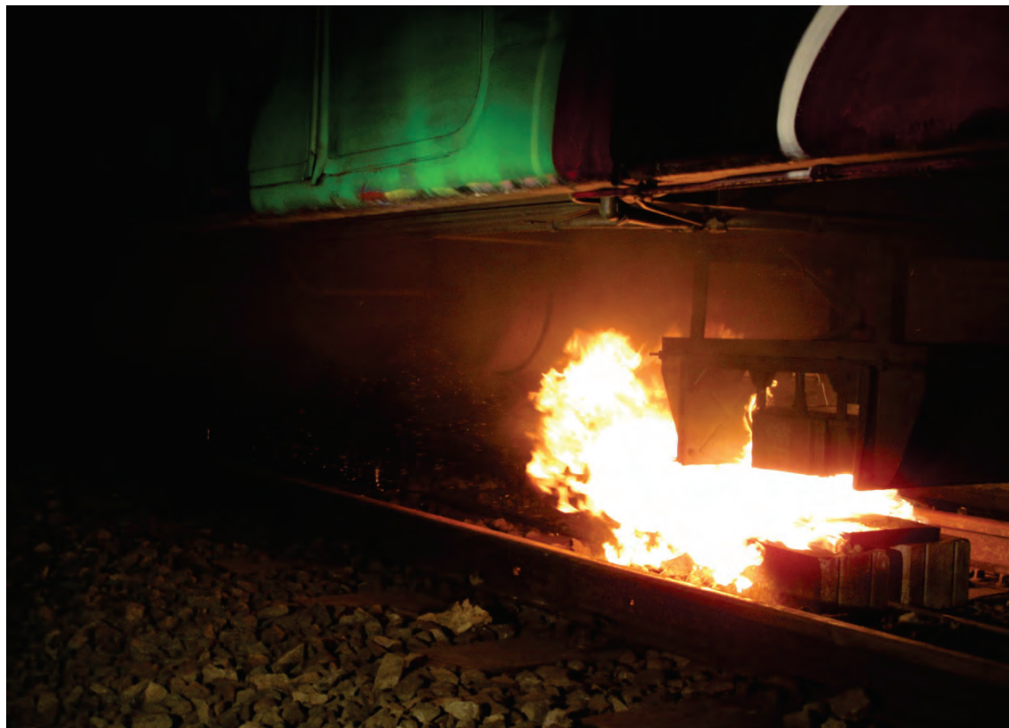
Figure A4.2 Flames from the heptane pool a few minutes after ignition in test 1.(Photo: Anders Lönnermark)
