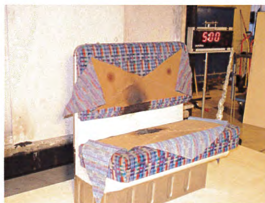
Photo 6 - Time 05:00. The smoke production has decreased.
