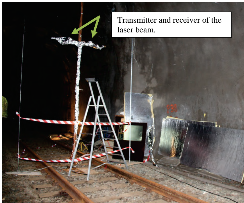
Figure 6.9 Position of the laser equipment in the measurement station.
