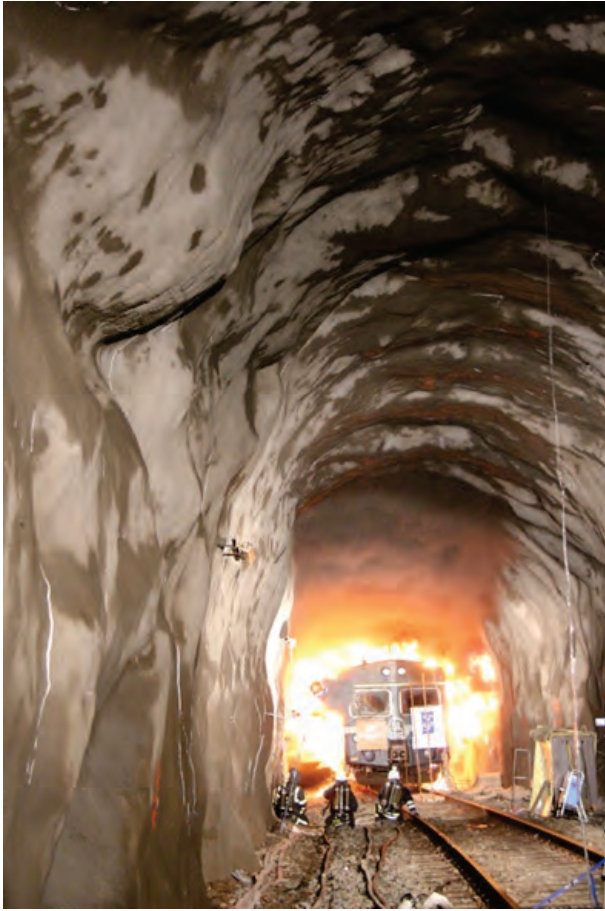
Figure A4.17 Flames from the carriage approx. 1h 57 min after ignition. The fire is now growing rapidly. From the picture it is also possible to see the emerging backlayering. (Photo: Per Rohlén)
