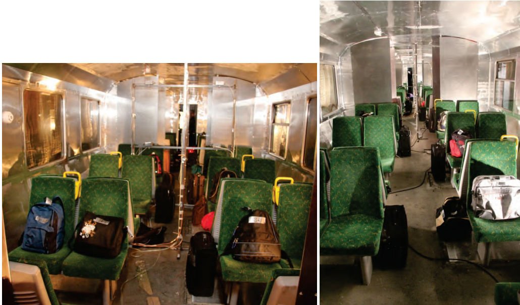
Figure 4.9 Pieces of luggage in, at or under different seats in the refurbished X1 carriage before the start of test 3. (Photo: Per Rohlén)
