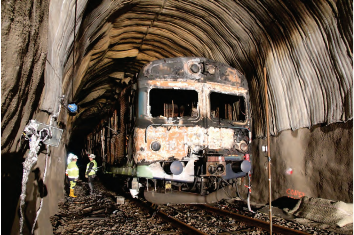
Figure A4.11 The remains of the carriage after test 2. (Photo: Per Rohlén)
