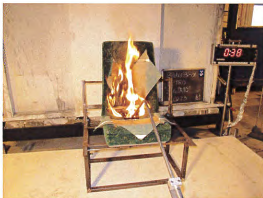
Photo 3 – Time 00:38. The foam on the backrest and parts of the seat is burning and small areas of the fabric have ignited. The flames are high and reaches over the top of the backrest.
