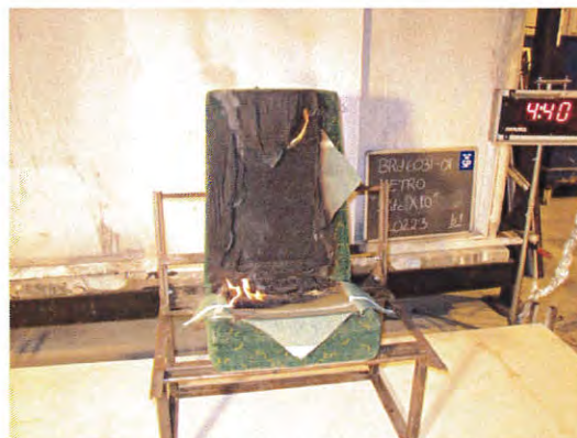
Photo 6 – Time 04:40. The fire has lost in intensity and only parts of the Velcro is burning as well as the foam around it.
