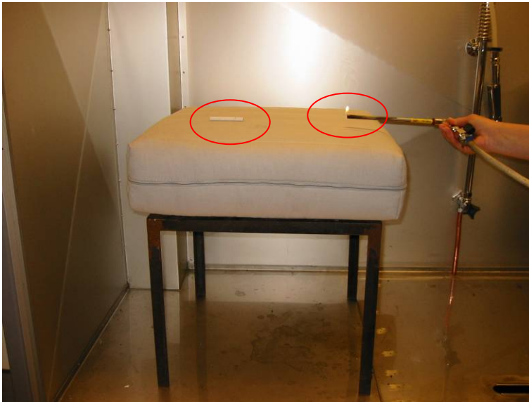
Figure I- 3 Test set-up for EN 597-1 (cigarette) and EN 597-2 (match flame). The test specimen is located on top of a steel rig. Depending on the finish of the mattress, ignition sources are placed on the flat surface, at tape edges, at quilted locations, tufts etc.
