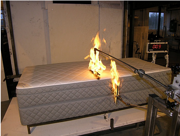
Figure I- 5 During testing according to 16 CFR Part 1633 a mattress is exposed to two T-shaped burners with a total burner heat output of 27 kW. During the test the heat release rate and the total energy developed are measured.
