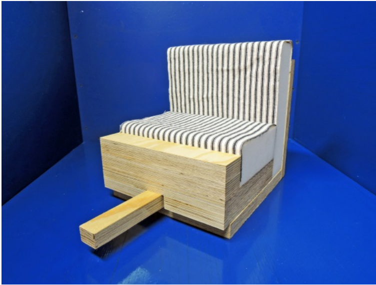
Figure I-6 Example of TB 117 test set-up of a filling in combination with a standard fabric. A glowing cigarette is placed in the junction between the seat and the back in the mock-up assembly.
