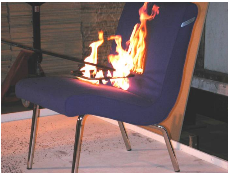
Figure I-7 During testing according to TB 133 a square gas burner with a heat output of 20 kW is positioned centrally on top of the seat for 80 s. During the test the heat release rate and the total energy developed are measured.
