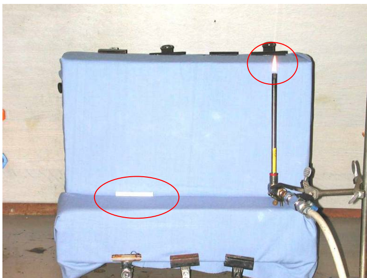
Figure I-2 Test set-up for testing according to EN 1021-1 (cigarette) and EN 1021-2 (match flame). The cover fabric and the filling are put in a test rig to create a small sofa with a 90° angle between seat and back. The ignition sources are located in the junction between seat and back. Note that the small gas flame is note located in the test position in the photo.
