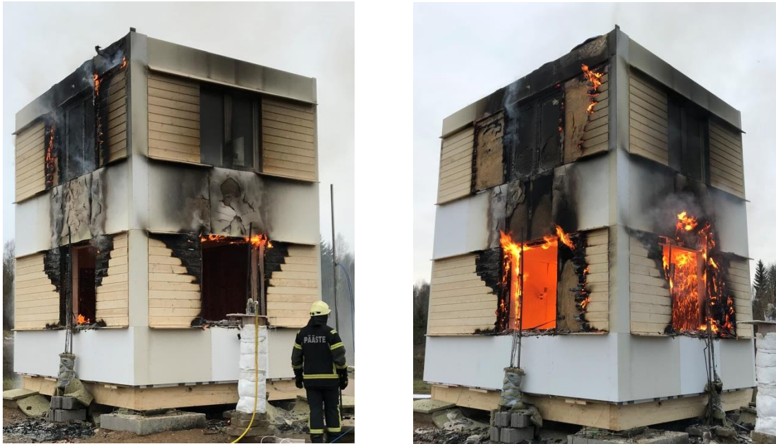
Figure 37: 35 minutes into the first decay phase at 1:17h (left) start of the second decay phase at 1:40h (right)
