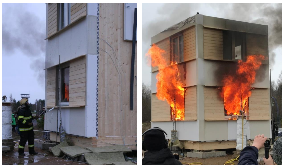
Figure 36: Breaking of the window at 0:20h (left) flashover at 0:47h (right)
