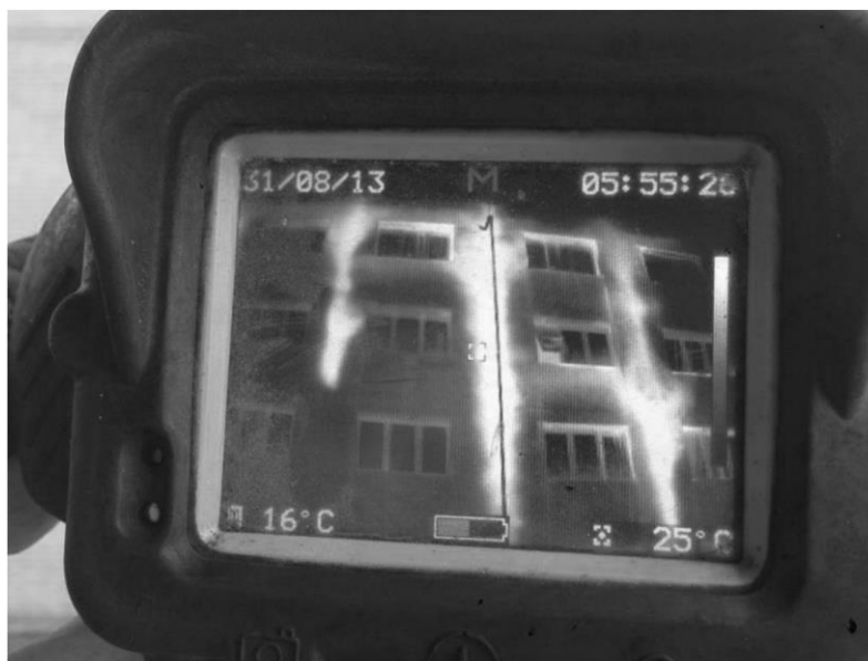
Figure 18: Infrared camera picture indicating a downwards fire spread through cavities 2
