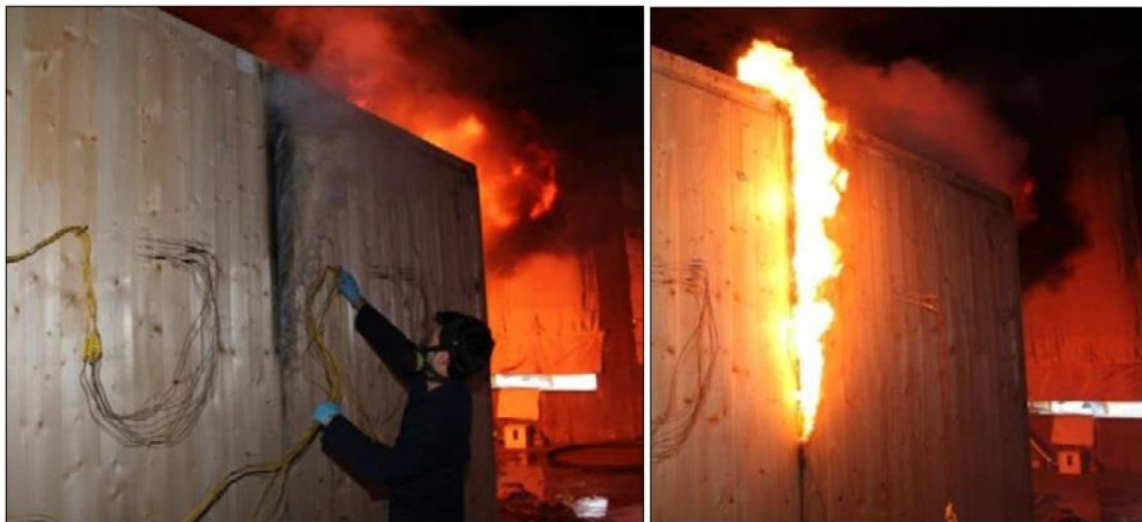
Figure 16: Fire spread through a CLT splice connection, taken from McGregor (2014).
