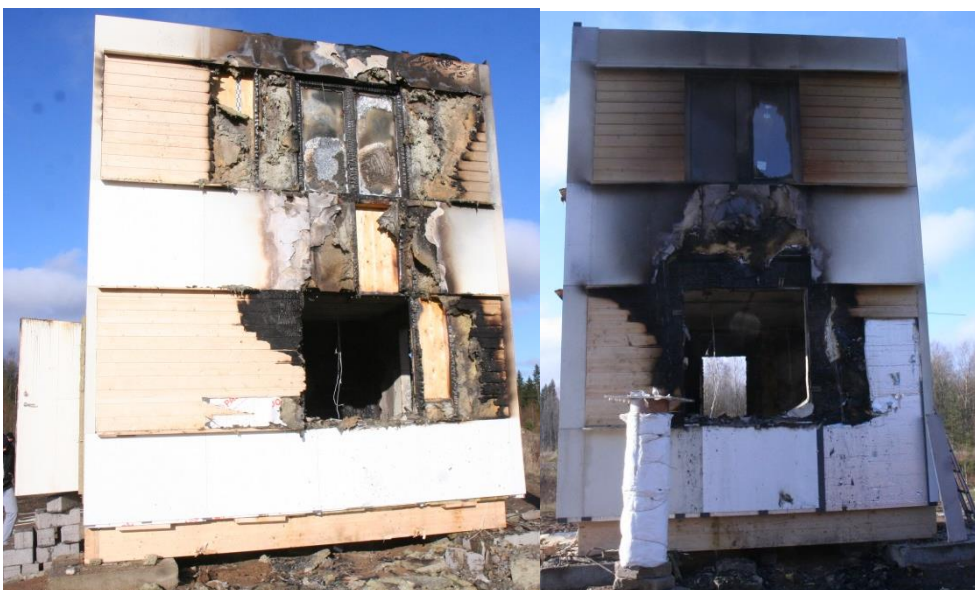
Figure 38: Façade with stone wool insulation (left) and PIR insulation (right, some panels removed)
