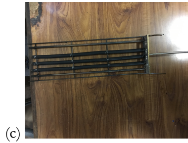
Figure 13 FPA test setup (a) sample inside quartz tubes (b) sample without quartz tube (c) sample holder.
