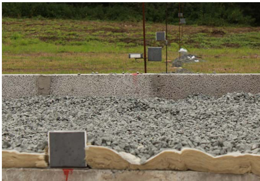
Figure 13 A view of the measurement setup in the west direction with the closest PT mounted on the rim of the test pool.
