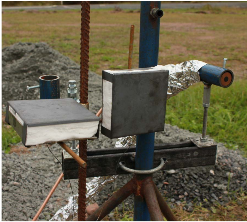
Figure 12 A picture of the measuring station (5 m east of the fire) where PT were mounted both in horizontal and vertical orientation, This station also included a heat flux meter.
