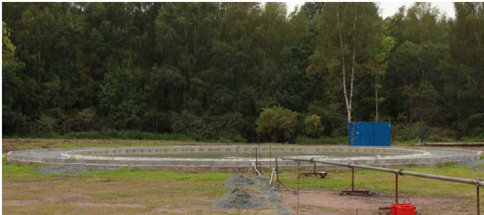
Figure 9 The fire tests were performed on an existing fire test pool ( \varnothing = 24 m) made of concrete and with a varying depth. An inner pool with a diameter of 18 m was constructed to provide a defined test area and a constant fuel depth. The rim of the inner pool was 150 mm high. The pipe to the lower right was used to fill the pool with fuel.
