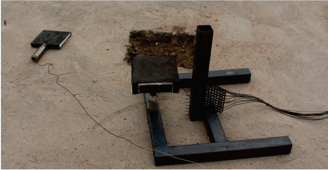
Figure A 8 The instrumentation for burning rate and flame exposure in the center of the pool.
