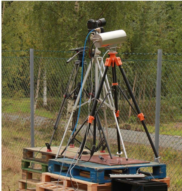
Figure 14 The location of two video cameras, one digital camera and one IR-camera at 57 m (IR 57.5 m) from the pool center in east direction.
