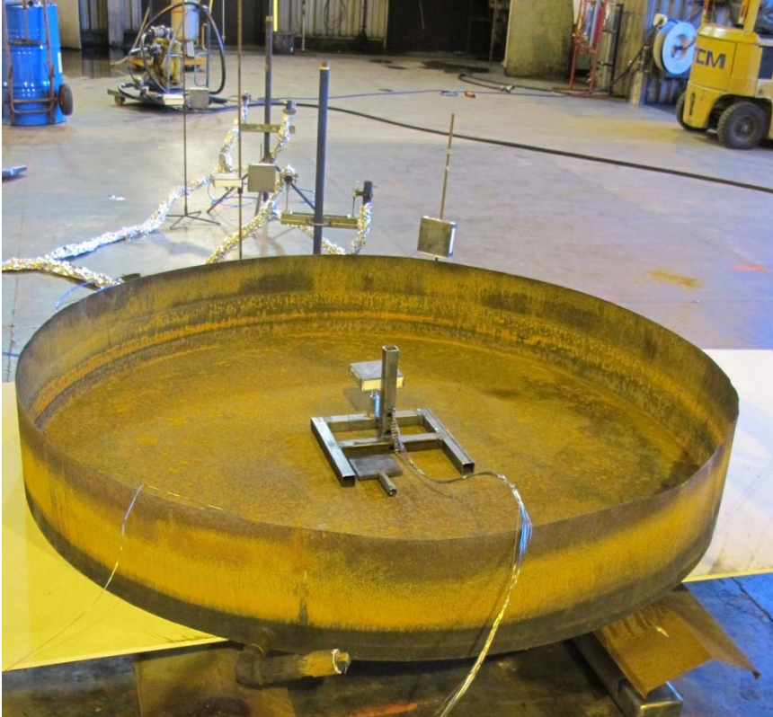
Figure 8 The 2.0 m 2 fire tray with the thermocouple arrangement in the tray and the PT and heat flux meter in “south” direction.
