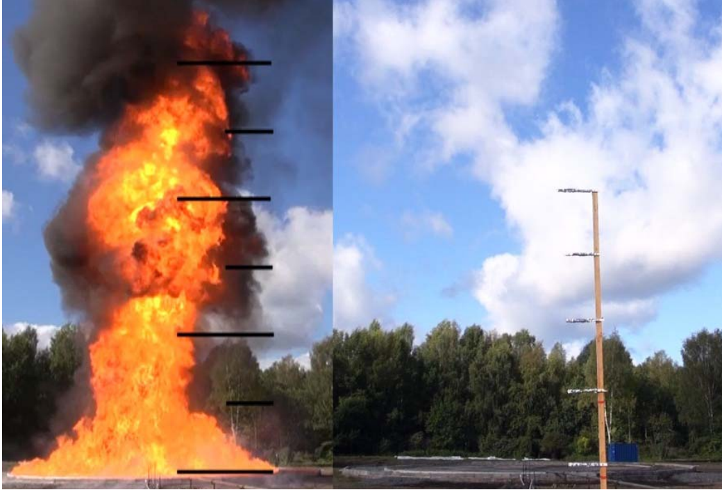
Figure 6 A measuring stick with markings every 0.5 m located at 1/10 of the distance to the pool center was used as a reference for the flame height measurements. The superimposed markings on the flame in the left image are 5 m apart.
