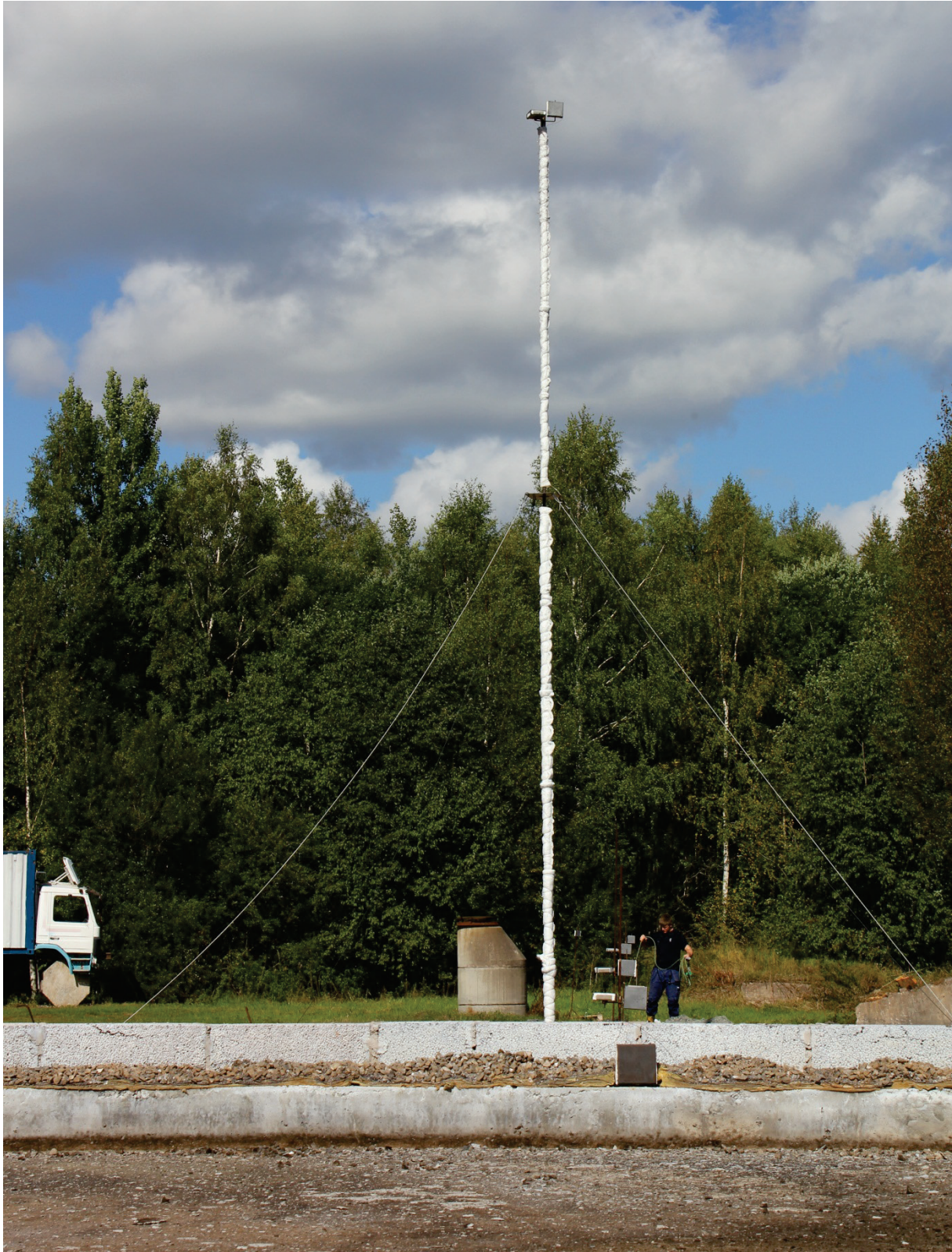
Figure A 10 A view of the instrumentation in north (downwind) direction, including the elevated PT at 10 m distance from the rim of the pool.
