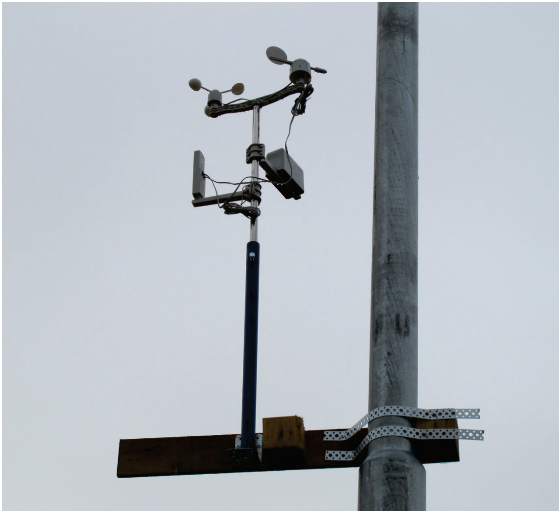
Figure A 9 The weather station located NW of the pool at about 4.5 m height above ground level.
