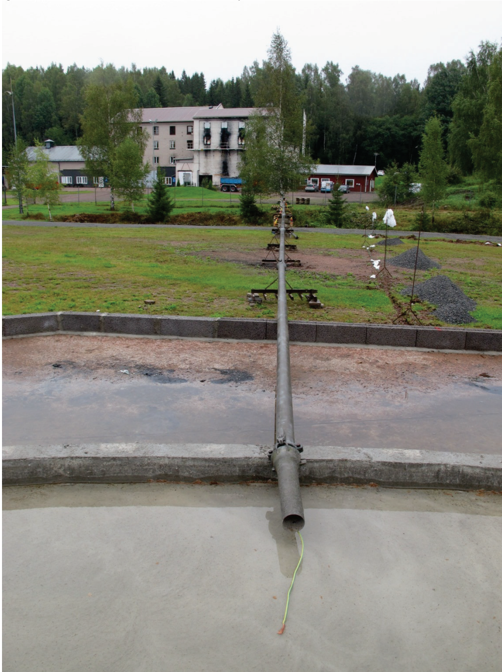
Figure A 7 The fuel filling pipe used during the tests and the support poles for the instrumentation in east direction.
