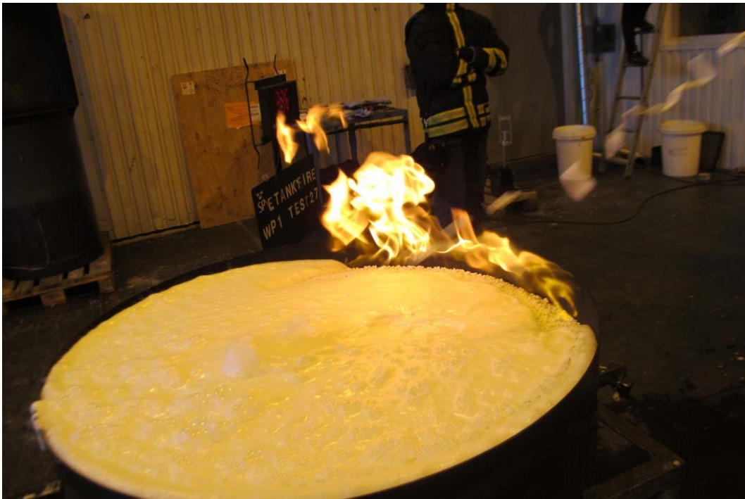
Figure 37 Test#27 (025) Test in the 2580-tray applying cellular glass (average 30 mm) followed by Type III foam application. Due to the thicker layer of cellular glass, no open fuel surface was created.
