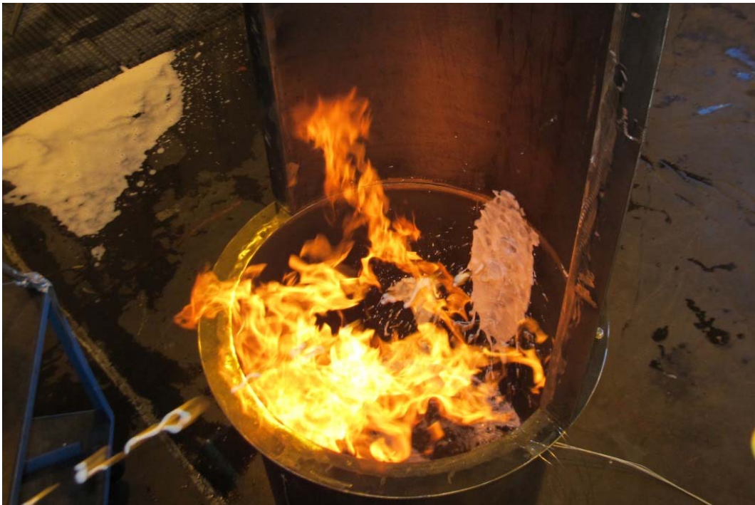
Figure 4 Test #4 (087) 225 mm fuel, foam impact position 0,575 m above fuel surface.
