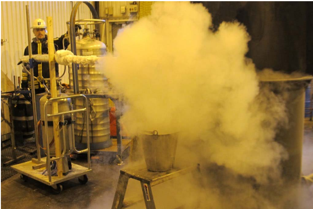
Figure 27 Test#22 (003) Sampling of liquid nitrogen to determine the flowrate before the fire test.
