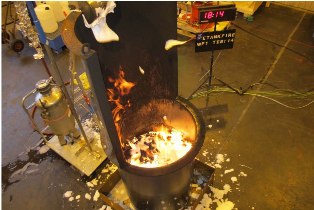
Figure 17 Test#14 (015) CAF application via the foam chamber. Still free fall of foam (3:14 min:s after start of application).
