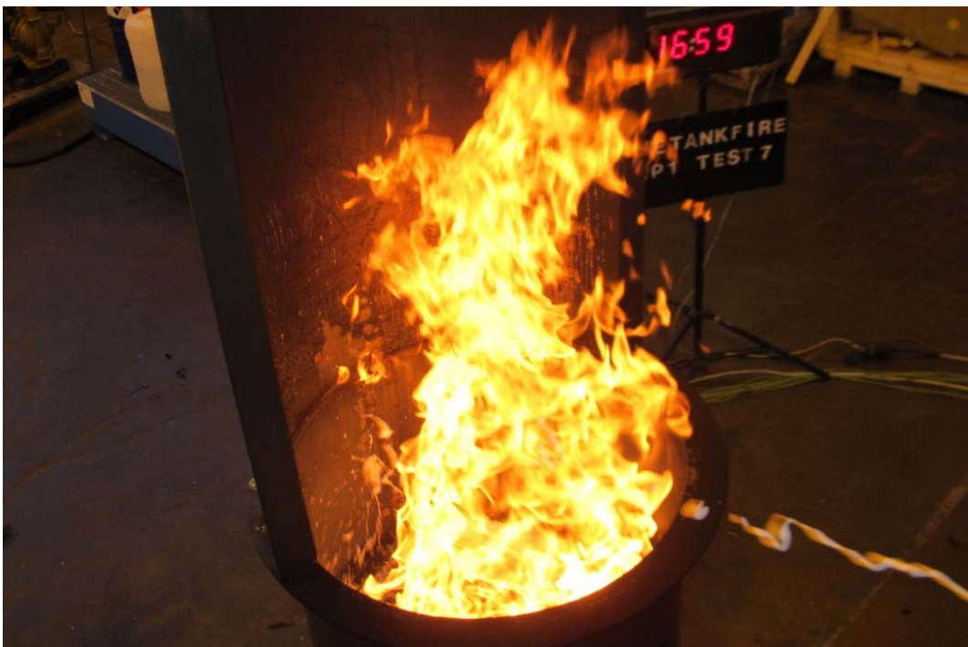
Figure 7 Test#7 (022) 450 mm fuel, preburn 15 minutes, foam impact position 0,35 m above fuel surface.
