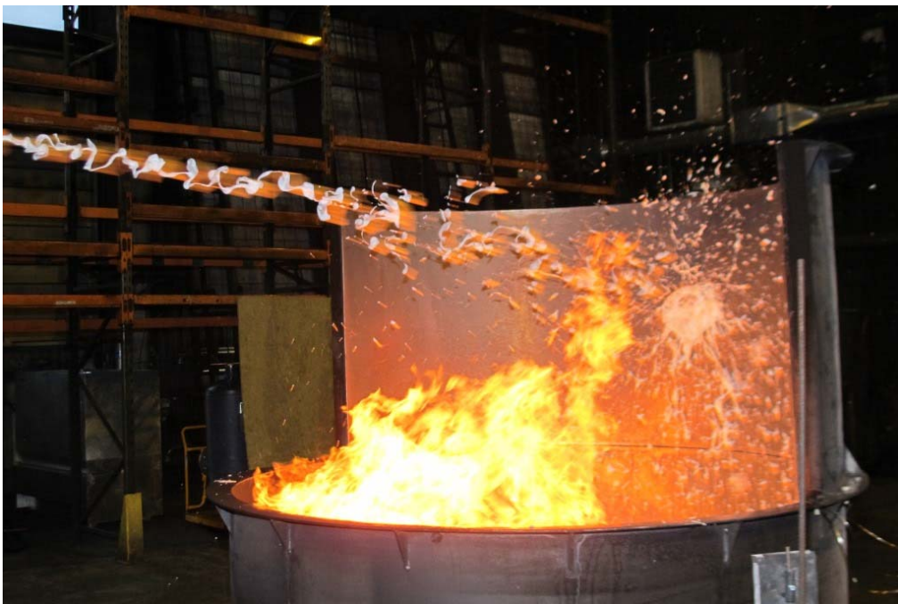
Figure 41 WP2-Test#2 (014) Identical to WP2-Test#1 but using AFFF-AR at 6% concentration (instead of 3%).
