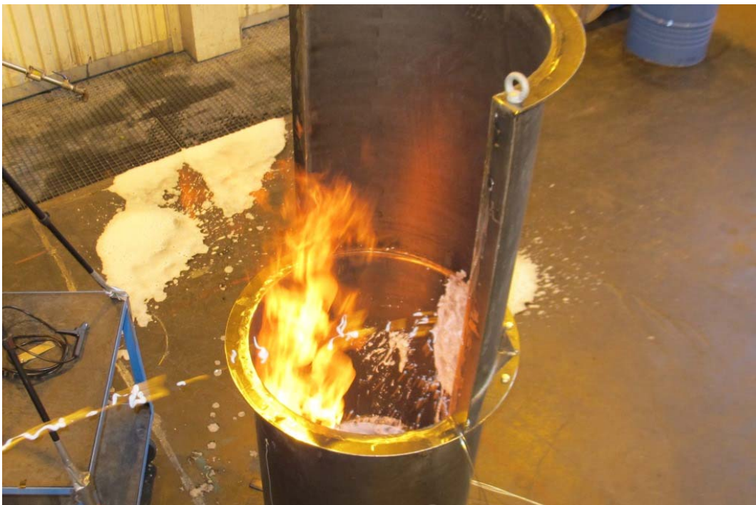
Figure 3 Test #3 (073) First test in the WP1 fire tray, 73 mm fuel, foam impact position 0,725 m above fuel surface.
