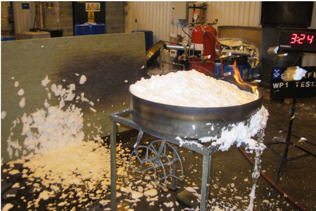
Figure 39 Test#28 (034) Test in the 2580-tray using CAF and Type III foam application showing the fire almost extinguished.
