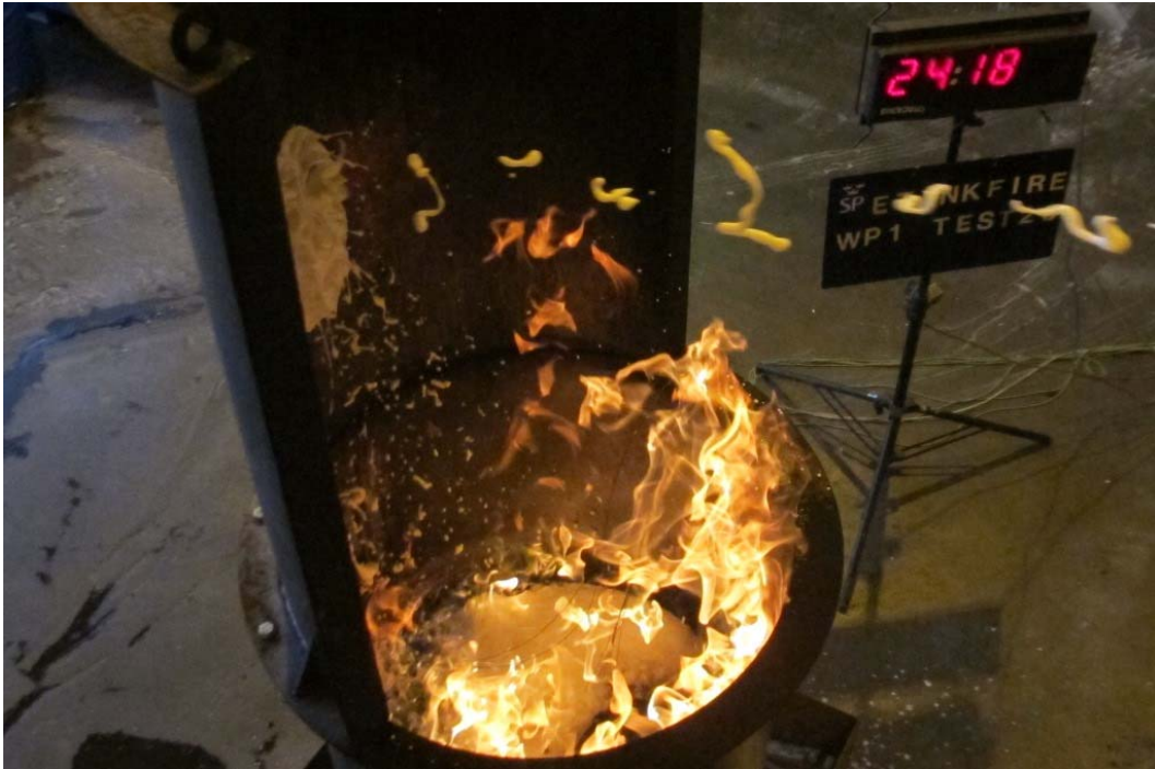
Figure 35 Test#25 (104) Similar to Test #8 and #21 but using 350 mm of fuel.
