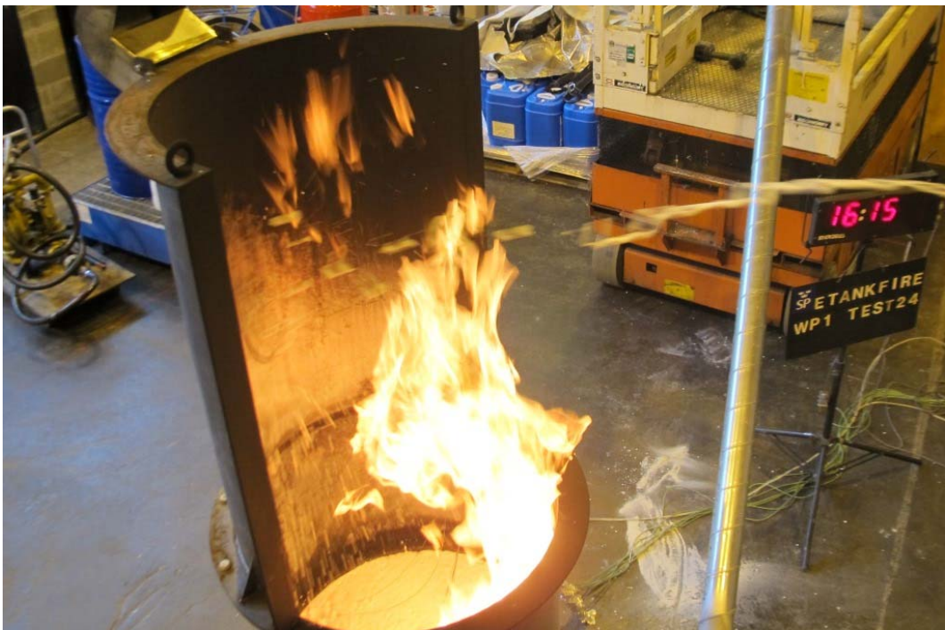
Figure 34 Test#24 (070) Application of cellular glass (average thickness 20 mm) followed by foam application at 1,05 m above the fuel/cellular glass surface.
