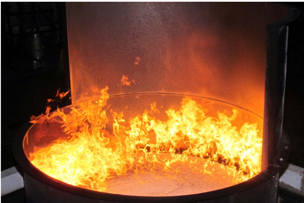
Figure 55 WP2-Test #13 (038) Within about 2 minutes, the fire intensity is reduced to about 25 % of its original intensity due to the applied layer of cellular glass.
