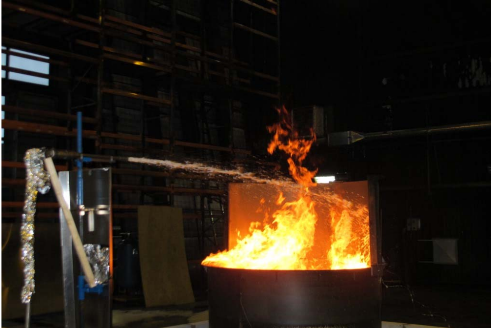
Figure 40 WP2-Test#1 (032) Test with AFFF-AR, 3%, under similar conditions as WP1-Test #8, foam impact position 1,05m above fuel surface. Picture shows the fire after about 15 minutes of foam application and as in the WP1 test, no control of the fire was obtained.
