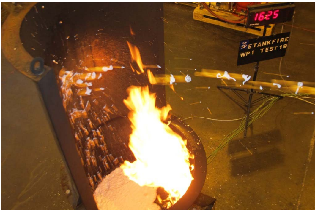
Figure 24 Test#19 (004) Similar to Test #8 but using F3 foam, foam impact position 1,05m above fuel surface.
