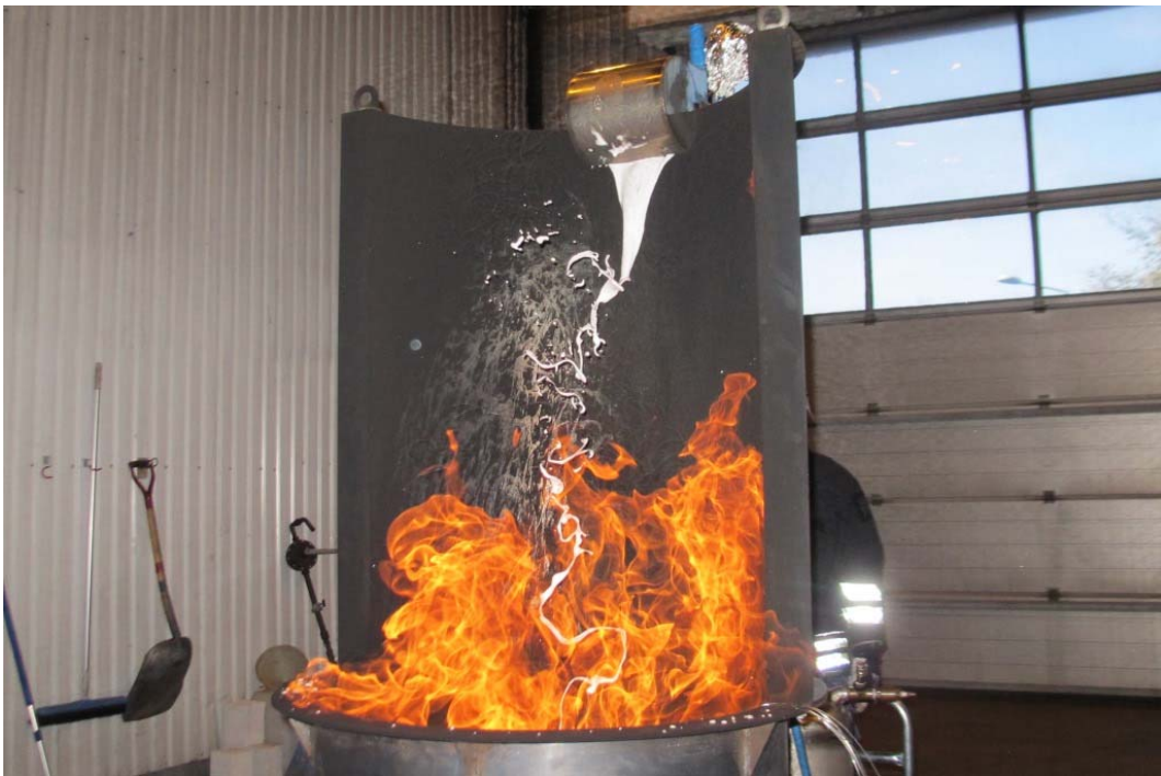
Figure 9 Test#9 (031) Foam chamber application, 1,55m above fuel surface. Free fall of foam due to the hot steel wall.
