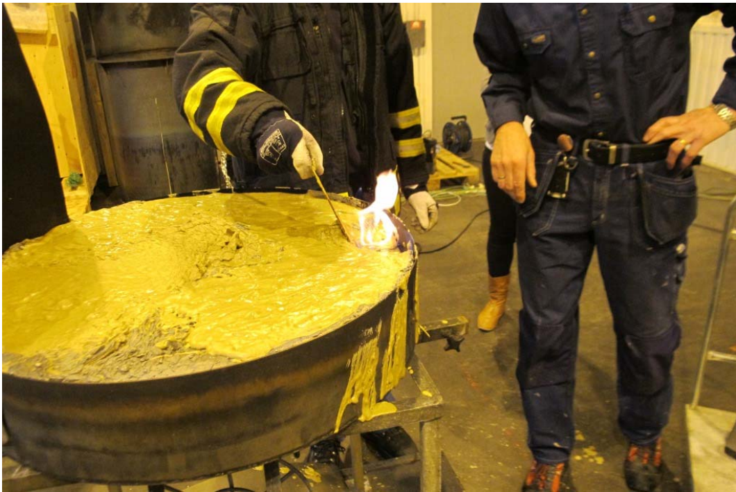
Figure 21 Test#17 (011) Check of the burnback resistance of the AVD foam layer.
