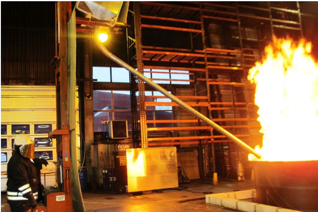
Figure 54 WP2-Test #13 (033) Test combined with application of cellular glass (average depth 50 mm), 10 min waiting followed by Type III foam application (AFFF-AR 3%, 3,63 l/m 2 min).
