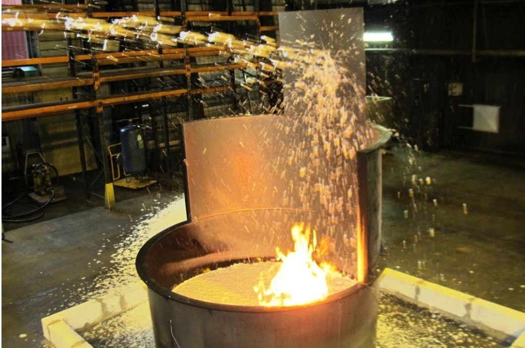
Figure 46 WP2-Test #6 (014) Similar to WP2-Test #3 ( 4,77 \text{ l/m}^2 \text{ min} ) but with foam impact position 2,05 m above the fuel surface.
