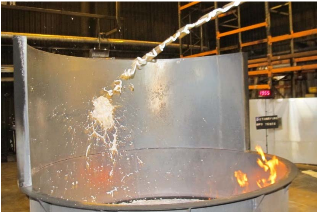
Figure 45 WP2-Test #5 (048) Similar to WP2-Test #2 and #3 but using even lower application rate ( 3,63 \text{ l/m}^2 \text{ min} )
