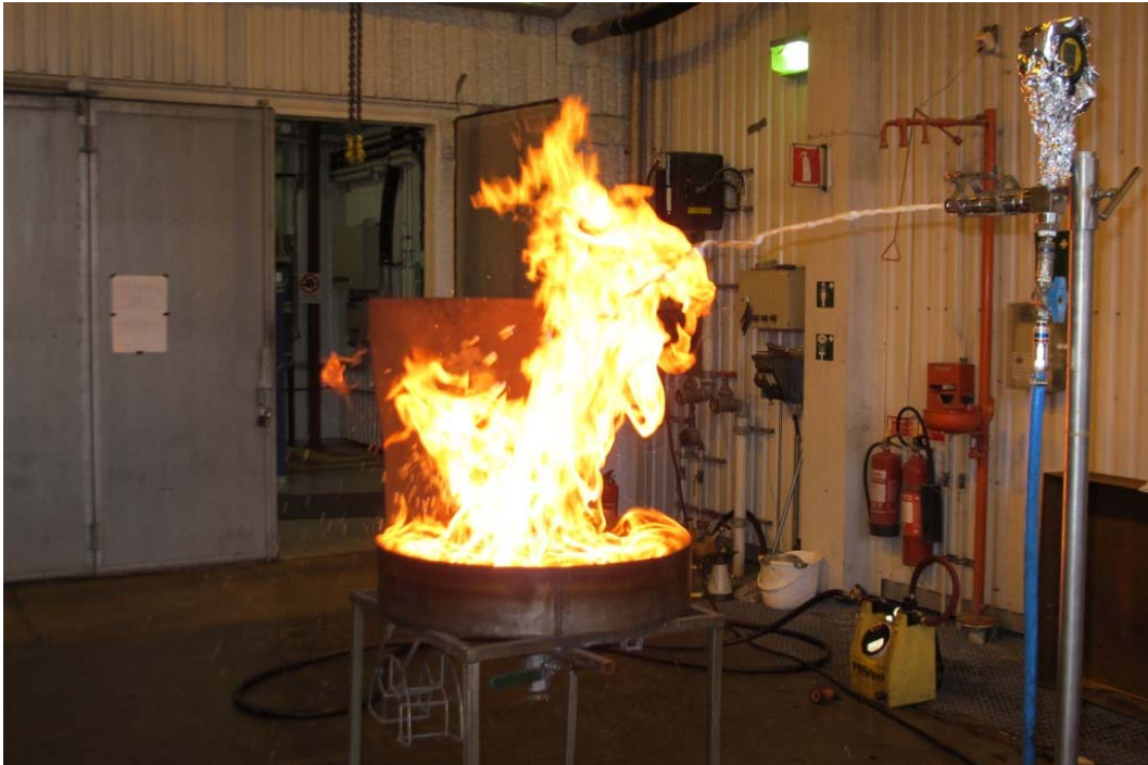
Figure 1 Test#1 (029) Test according to SP method 2580 using ethanol as fuel.
