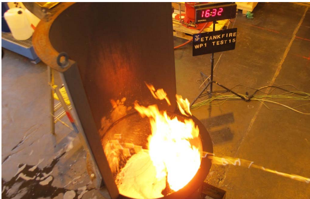
Figure 18 Test#15 (033) Repeat of Test #7, foam impact position 0,35 m above fuel surface.
