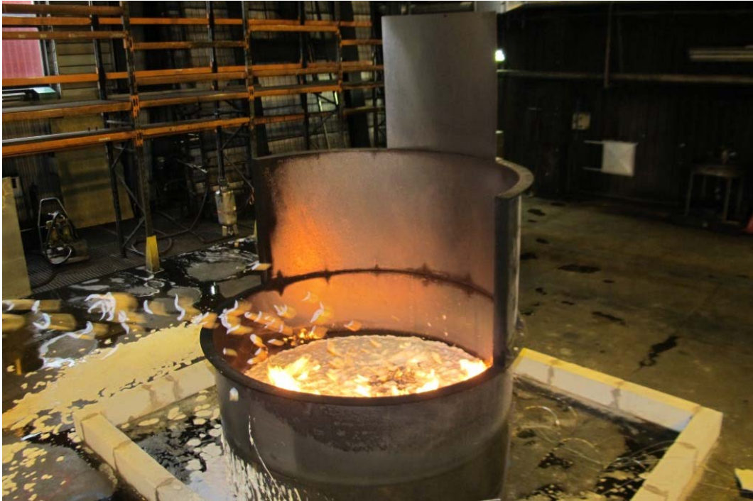
Figure 50 WP2-Test #9B (029) Retest using the same fuel as in Test #9, but using Type III application. (Preburn time reduced to 5 min).
