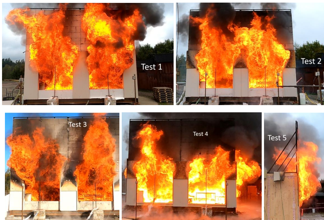
Figure 12. Snapshots from each test at 2 minutes after flashover.
