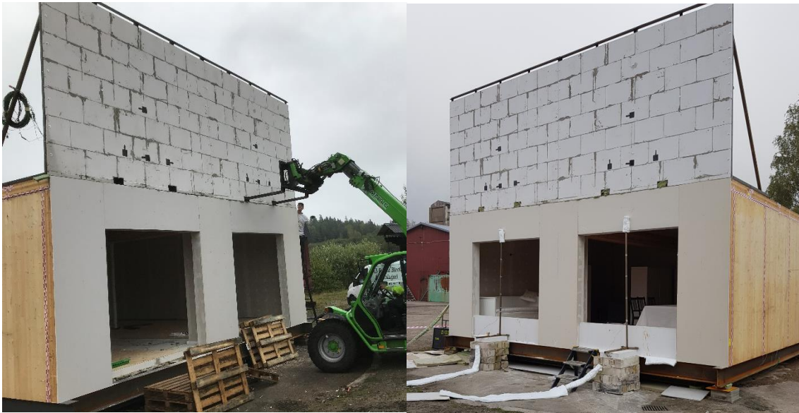
Figure 5. Placement of a façade mock-ups on the construction (left). Facades in place prior to test 1. The façade structure was instrumented with a number of thermocouples (TC) corresponding to some of the assessment points in test standards (NFPA, CAN/ULC, BS 8414, ISO 13785-2, SP Fire 105 as well as the recently proposed European method) or location where additional measurements have been taken in available standard tests, as shown in Figure 6. In addition, four plate thermometers (PT), as used in standard fire resistance furnaces (Wickström, 1994) were embedded flush to the surface of each façade mock-up (Figure 7). A full list of instrumentation including their location and number can be found in Annex B.
