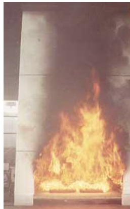
Figure 36 Front view of the SP-FIRE 105 test (picture courtesy RISE)
