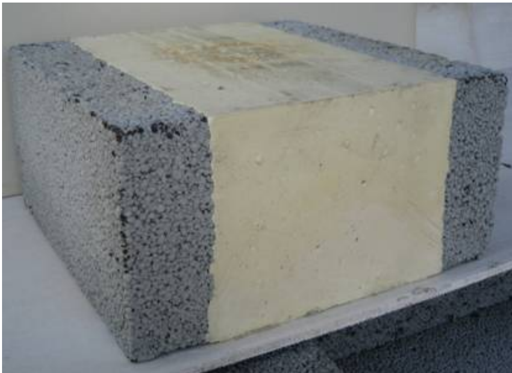
Figure 12 Example of a light weight composite concrete wall system (without rendering) Picture Miklos Molnar.
