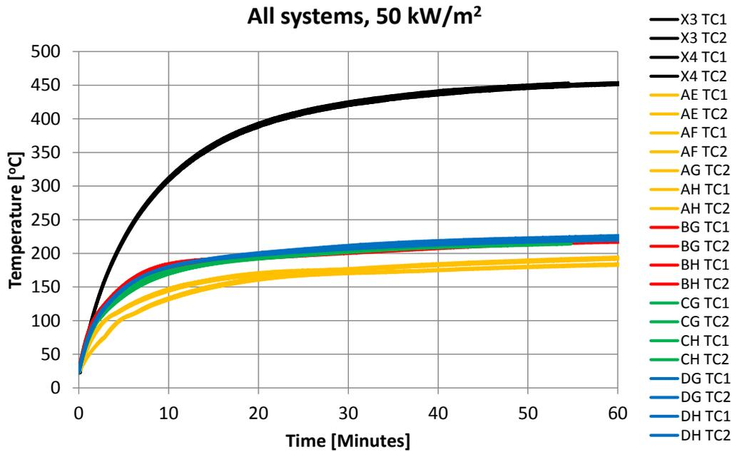
**Figure 10** Cone calorimeter tests during incident heat flux 50 kW/m<sup>2</sup>. Shown in the graph are steel temperatures on the heat exposed surface. All measurements can be seen in Appendix A.
