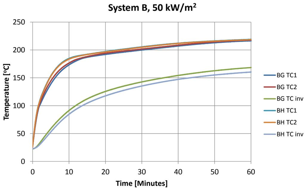
**Figure 49** Cone calorimeter tests on steel with intumescent paint system B, 50 kW/m<sup>2</sup> exposure.
