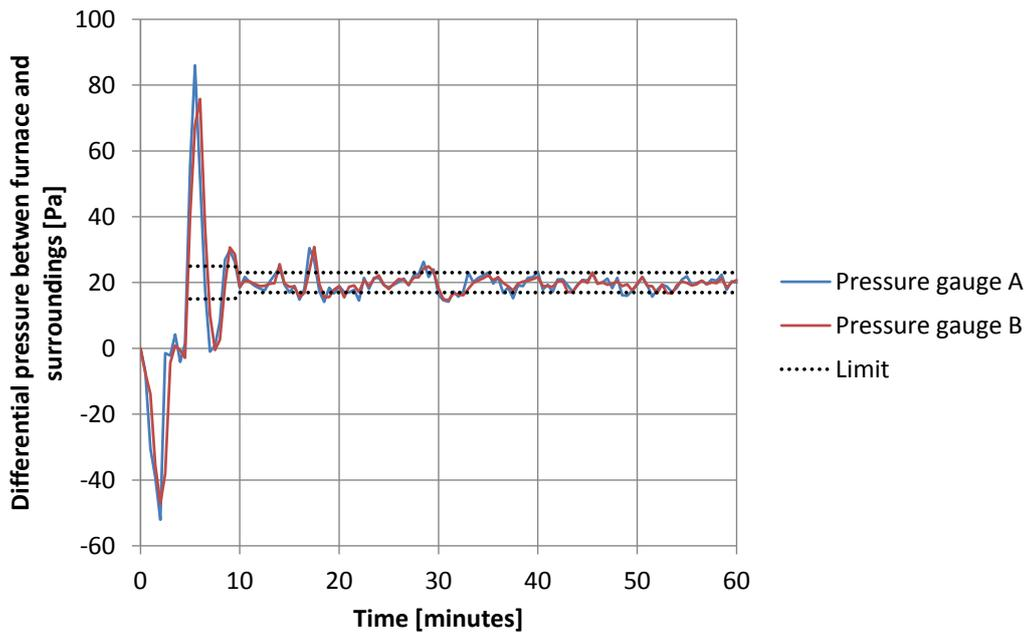
**Figure 14 Pressure difference between furnace and surroundings on the height 100 mm beneath the furnace roof as measured with two different gauges. The pressure was outside the limits stated in the standard during the time 5-10 minutes.**
