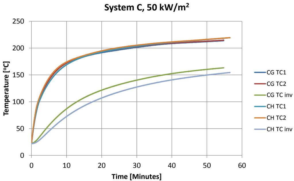
**Figure 51** Cone calorimeter tests on steel with intumescent paint system C, 50 kW/m<sup>2</sup> exposure.
