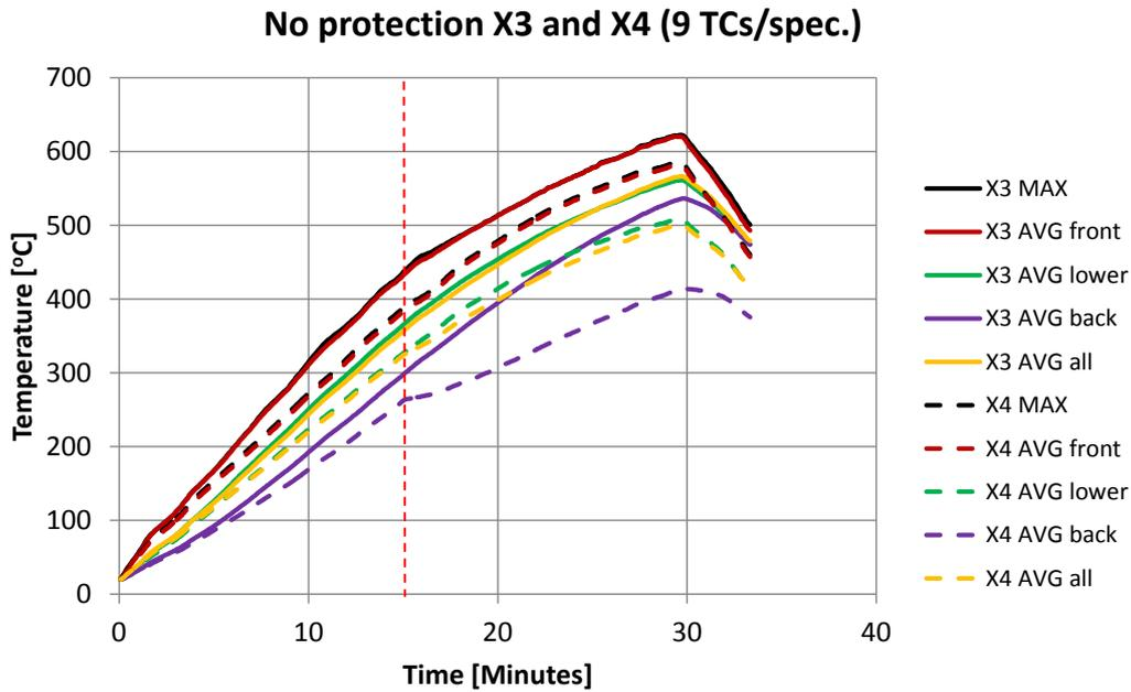
**Figure 30** Measured temperatures in the steel section during test 6, test specimen X2 and X4 exposed to the ceiling jet scenario. The red horizontal line marks the time 15 minutes when the right side of the test rig was opened. Exposure temperatures during test 6 can be found in Appendix.
