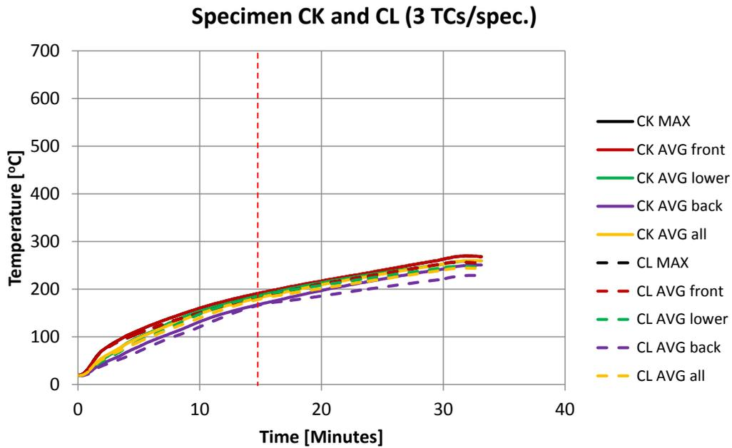
**Figure 34** Measured temperatures in the steel section during test 4, test specimen AM and AN exposed to ceiling jet scenario. The red horizontal line marks the time 15 minutes when the right side of the test rig was opened. Exposure temperatures during test 4 can be found in Appendix A.
