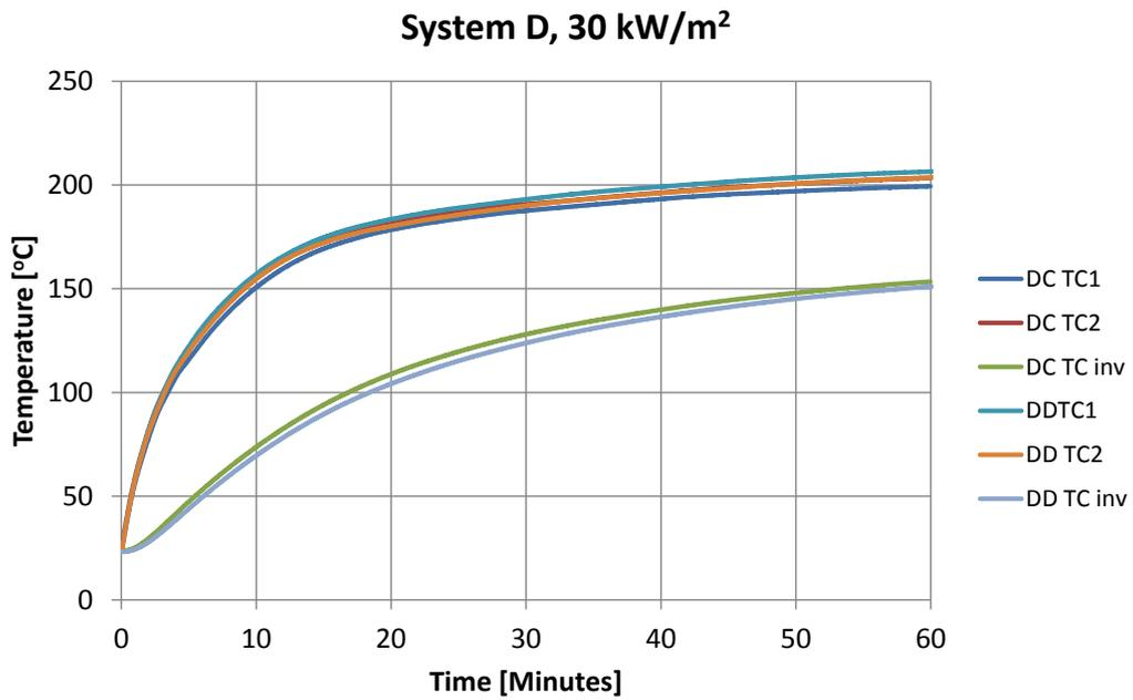
**Figure 52** Cone calorimeter tests on steel with intumescent paint system D, 30 kW/m<sup>2</sup> exposure.
