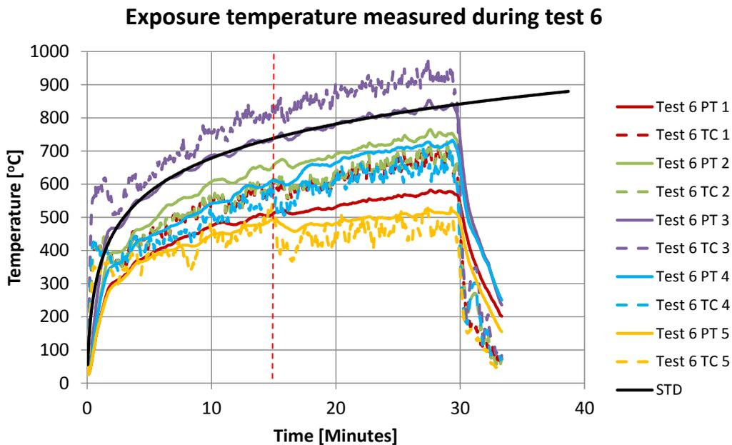
**Figure 28 Example of temperature development during exposure according to the ceiling jet scenario with reference specimens without protection, measurements from all tests are shown in the appendix. The red horizontal line marks the time 15 minutes when the right side of the test rig was opened.**
