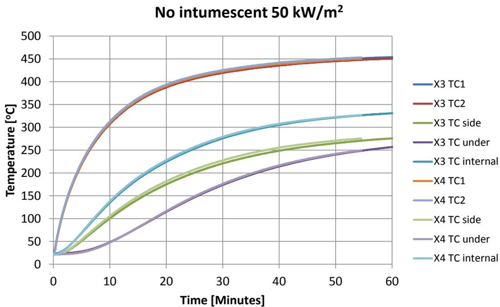
Figure 45 Cone calorimeter tests on steel without intumescent paint, 50 kW/m<sup>2</sup> exposure.
