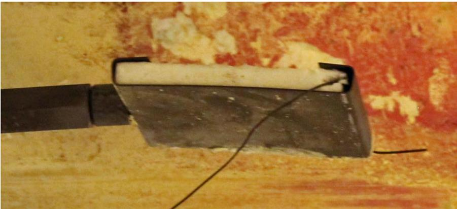
**Figure 25** Plate thermometer pointing downwards, paired with a 1 mm shielded thermocouple sticking out 3 cm from the plate.
