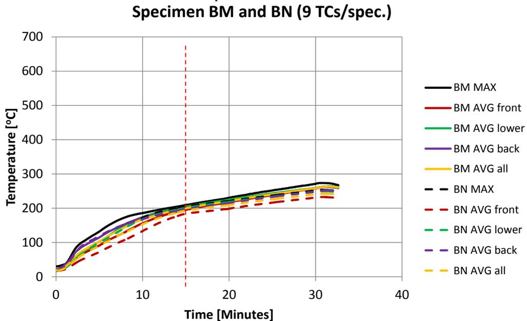
**Figure 33** Measured temperatures in the steel section during test 3, test specimen BM and BN exposed to ceiling jet scenario. The red horizontal line marks the time 15 minutes when the right side of the test rig was opened. Exposure temperatures during test 3 can be found in Appendix A.
