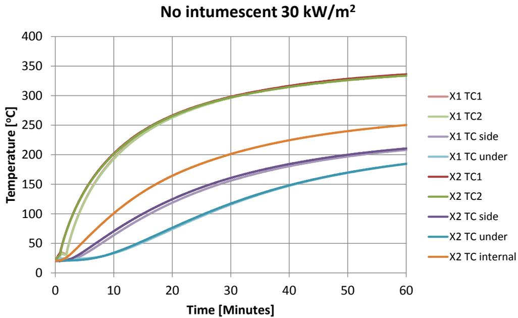
Figure 44 Cone calorimeter tests on steel without intumescent paint, 30 kW/m<sup>2</sup> exposure.
