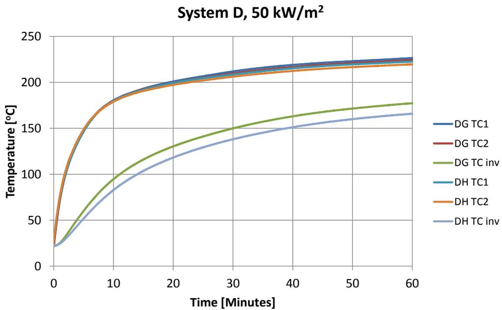
**Figure 53** Cone calorimeter tests on steel with intumescent paint system D, 50 kW/m<sup>2</sup> exposure.
