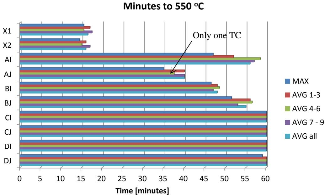
**Figure 21** Time to reach the design temperature 550 °C during standard fire exposure. Thermocouples 4-6 are on the bottom, horizontal part of the specimens. Specimen C1, C2, D1 and average temperatures in specimens D2 did not reach 550 °C during 60 minutes.
