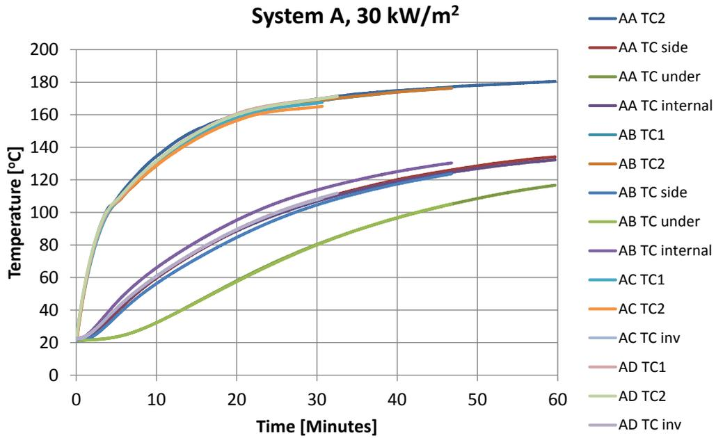
**Figure 46** Cone calorimeter tests on steel with intumescent paint system A, 30 kW/m<sup>2</sup> exposure.
