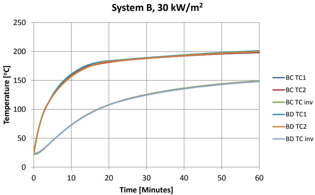
**Figure 48** Cone calorimeter tests on steel with intumescent paint system B, 30 kW/m<sup>2</sup> exposure.
