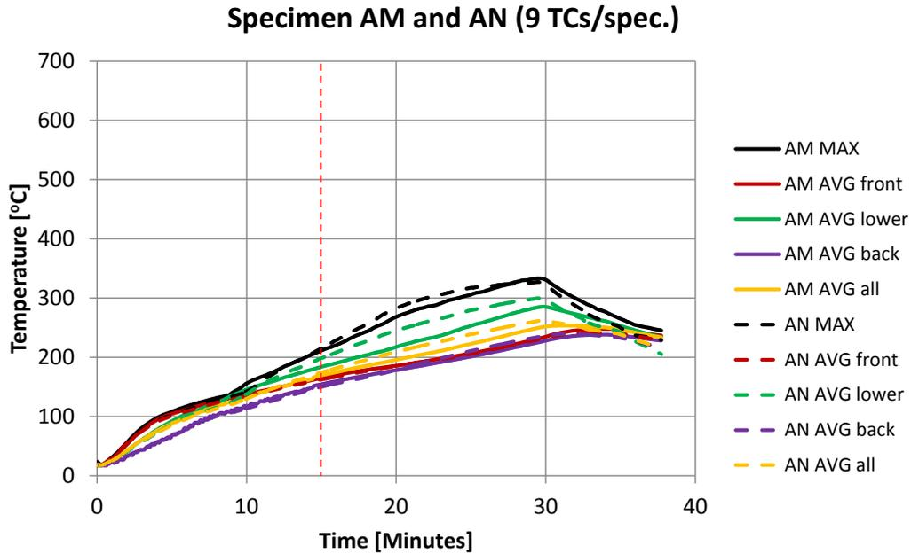
**Figure 32** Measured temperatures in the steel section during test 2, test specimen AM and AN exposed to ceiling jet scenario. These temperatures show an overestimation of the function since paint falling down on the instrumentation was shielding it from radiation from the fire. The red horizontal line marks the time 15 minutes when the right side of the test rig was opened. Exposure temperatures during test 2 can be found in Appendix A.
