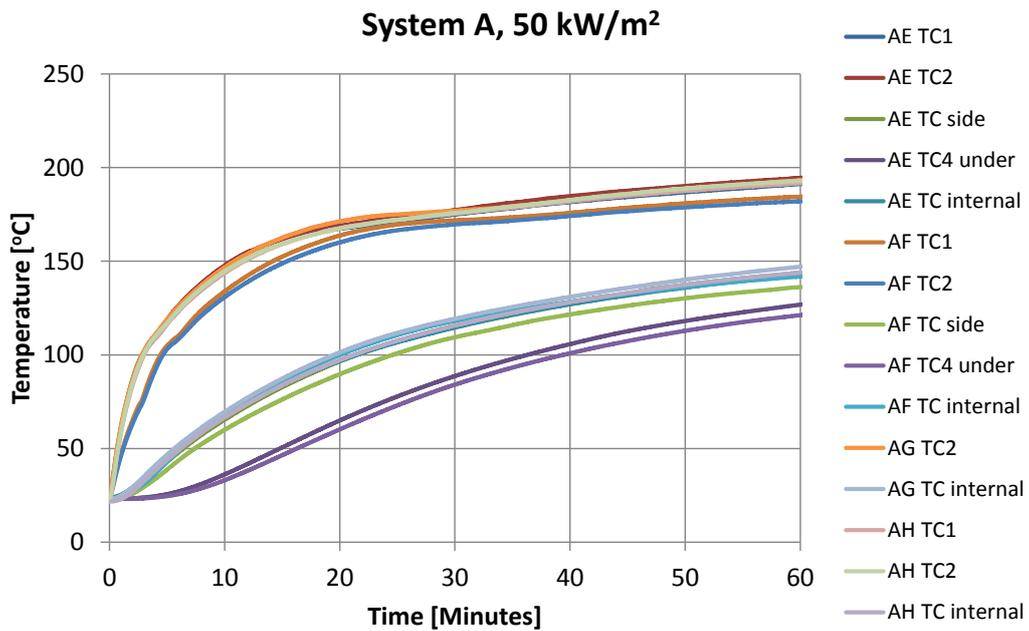
**Figure 47** Cone calorimeter tests on steel with intumescent paint system A, 50 kW/m<sup>2</sup> exposure.
