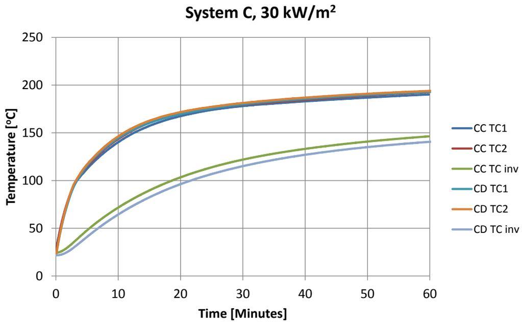
**Figure 50** Cone calorimeter tests on steel with intumescent paint system C, 30 kW/m<sup>2</sup> exposure.
