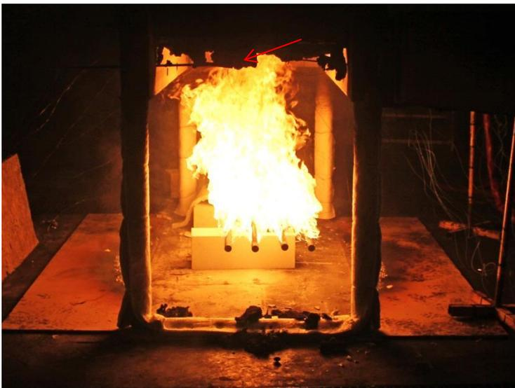
**Figure 31** Release of parts of system A during ceiling jet scenario. Photo taken after the opening of the side, chunks of paint on the instrumentation 100 mm below the surface (red arrow) and on the floor.
