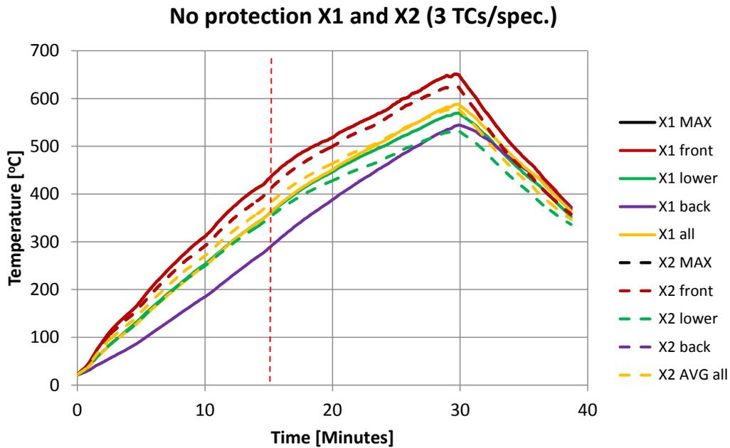
**Figure 29 Measured temperatures in the steel section during test 1, test specimen X1 and X2 exposed to the ceiling jet scenario. The thermocouple on the back side of specimen X2 was defect. This makes the average temperature “X2 AVG all” less representative for comparison with other tests. The red horizontal line marks the time 15 minutes when the right side of the test rig was opened. Exposure temperatures during test 1 can be found in Appendix A.**
