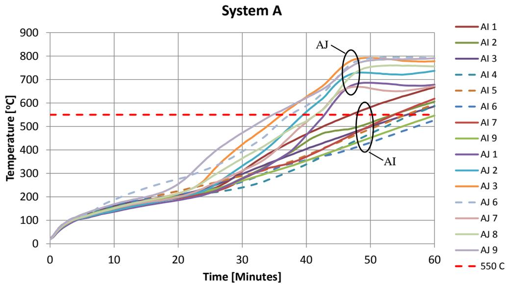
**Figure 16** Temperatures in system A specimens during furnace testing. The design temperature 550 °C is included as a reference. Measurements on the underside of the specimen is marked with dashed lines.
