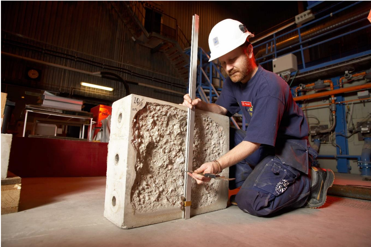
Figure 3. Spalled test specimen after fire exposure. The three holes in the specimen were used for the post stressing bars in the loading system, (Boström & Jansson, 2008).
