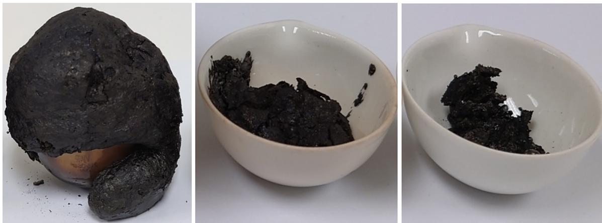
*Figure 7. Flame retardants heated to 400°C. From left to right: Na<sub>3</sub>ArgPA, Ca-Na<sub>3</sub>ArgPA, Al-Na<sub>3</sub>ArgPA.*
