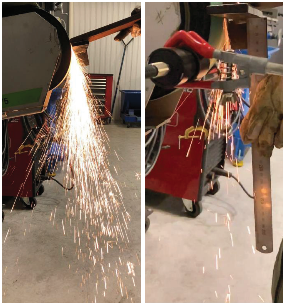
Figure 37. More snapshots from the spark generation of the grinding belt used for temperature evolution of the fragments.
