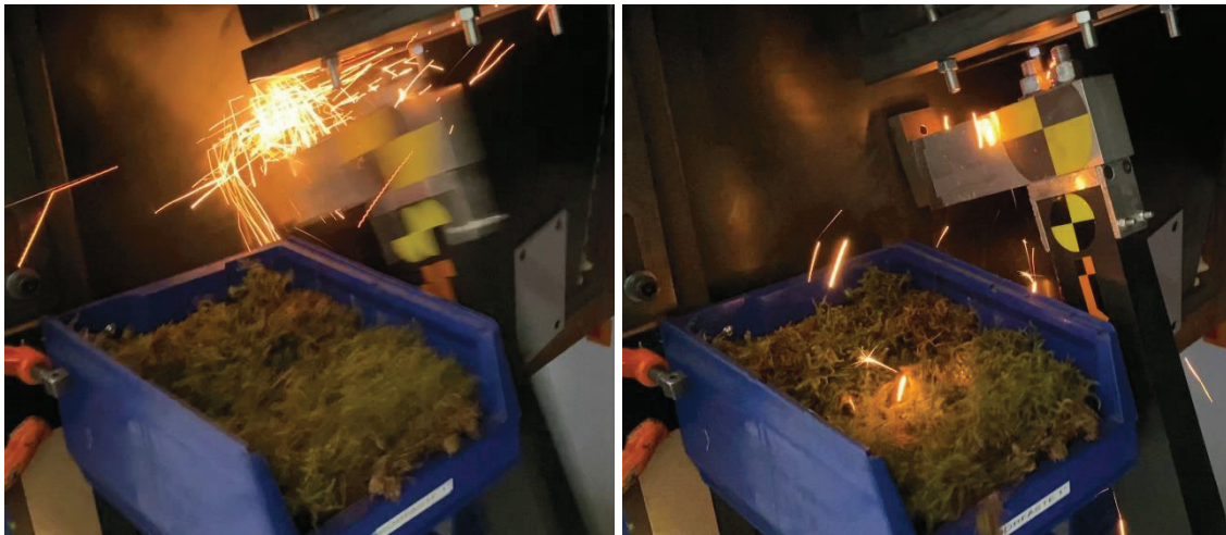
Figure 15. Upper: Axe testing equipment turned into a single strike apparatus producing glowing fragments of Hardox. Lower: Photo during (left) and just after (right) the strike.
