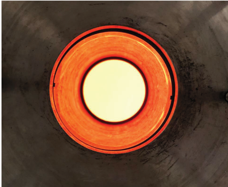
Figure 29. Visual photo of the spherical black body furnace used to validate the temperature measurements using spectroscopy. Photo shows the furnace exterior (metal grey) and the duct (orange) leading into the furnace interior (yellow) at 1173 K.
