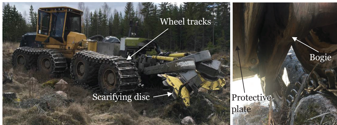
Figure 1. Left : overview of a scarifier use for site preparation. Right : photo from below the machine showing the protection plate, the bogie and the wheel tracks on an extruding rock.
