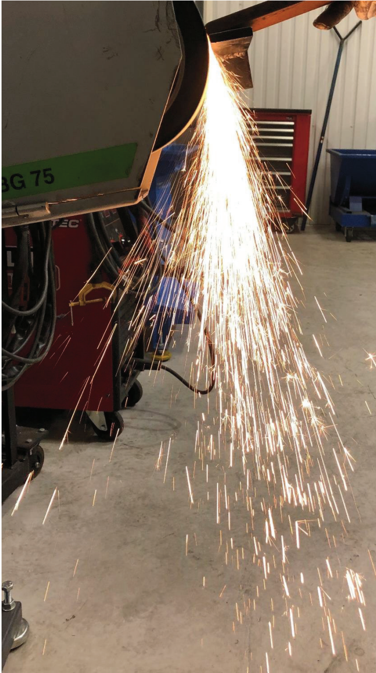
Figure 14. The shower of sparks from Hardox forced against a grinding belt.
