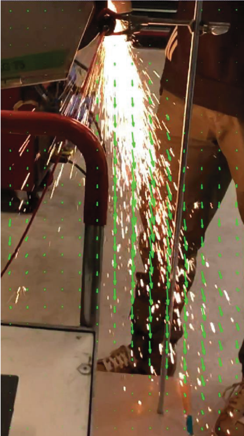
Figure 38. PIV analysis assessing showing the video snapshot and the velocity of sparks (arrows) assessed from the previous snapshot.
