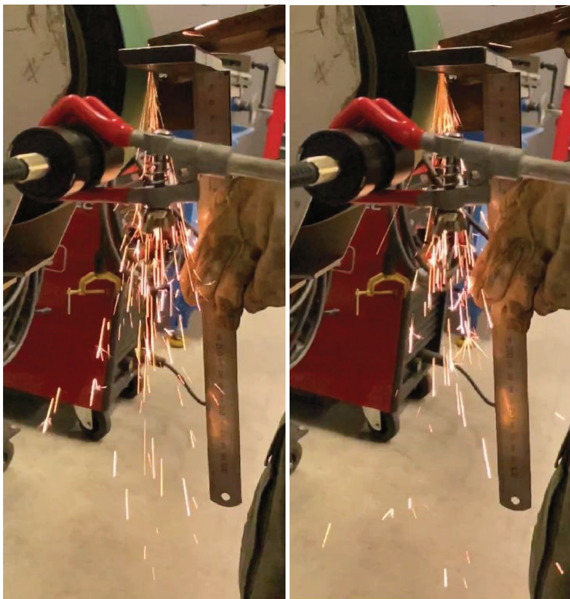
Figure 36. Snapshots from the spark generation of the grinding belt used for temperature evolution of the fragments.
