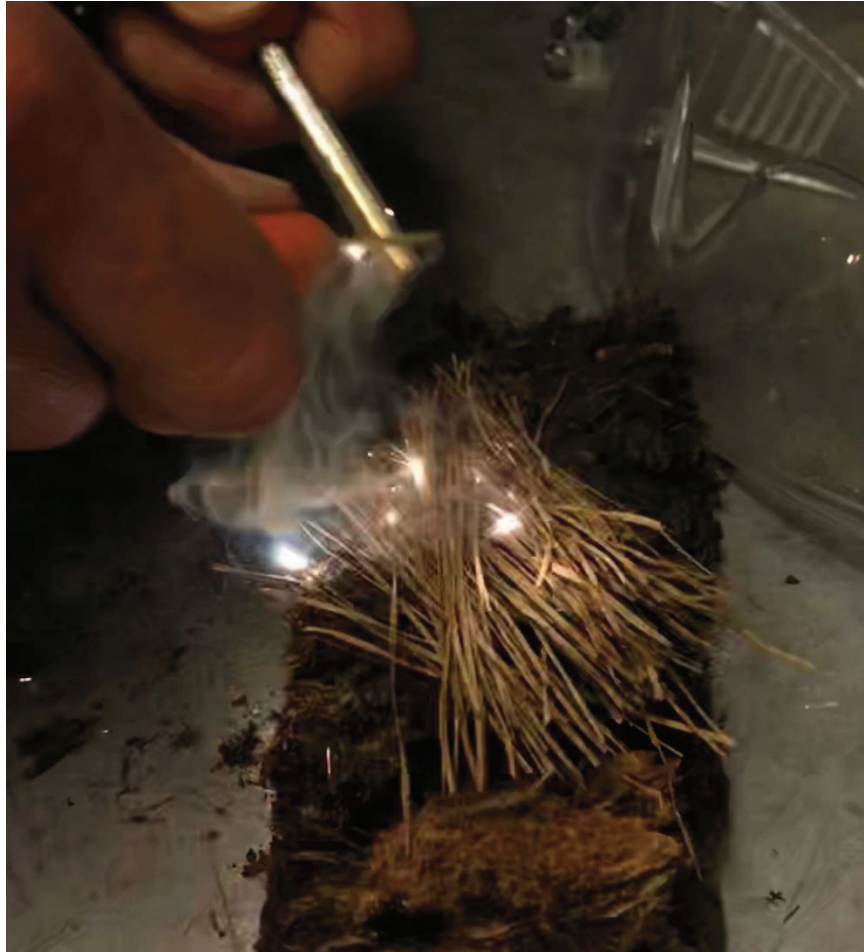
Figure 11. Swedish Fire Steel (LMF) from LightMyFire® used to produce sparks towards grass and humus.
