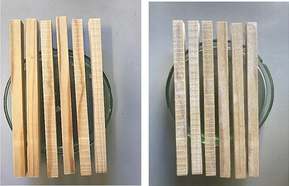
Fig. 20. Wood specimens before the mineralisation and after the impregnation.
