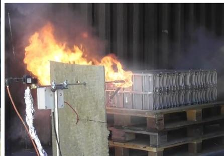
(b) thermal runaway event during a free burn test.
