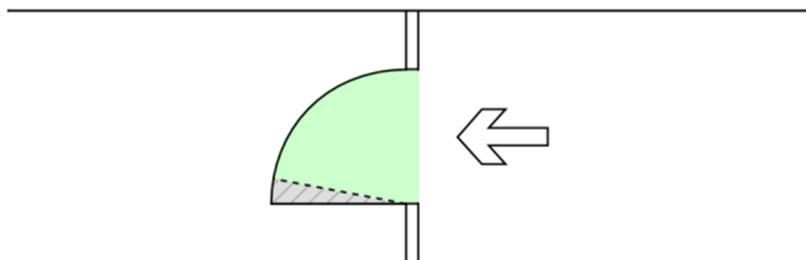
Figure 27. Visualization of the "shading effect" noted in scenarios with outward opening door. Figure reproduced from [7].
