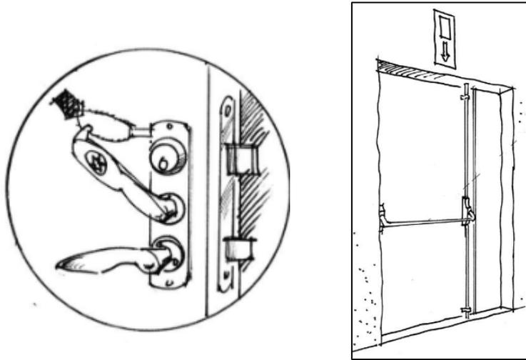
Figure 26. Door fittings according to SS-EN 179 (left) and SS-EN 1125 (right), illustrations from Brandskyddshandboken [30].
