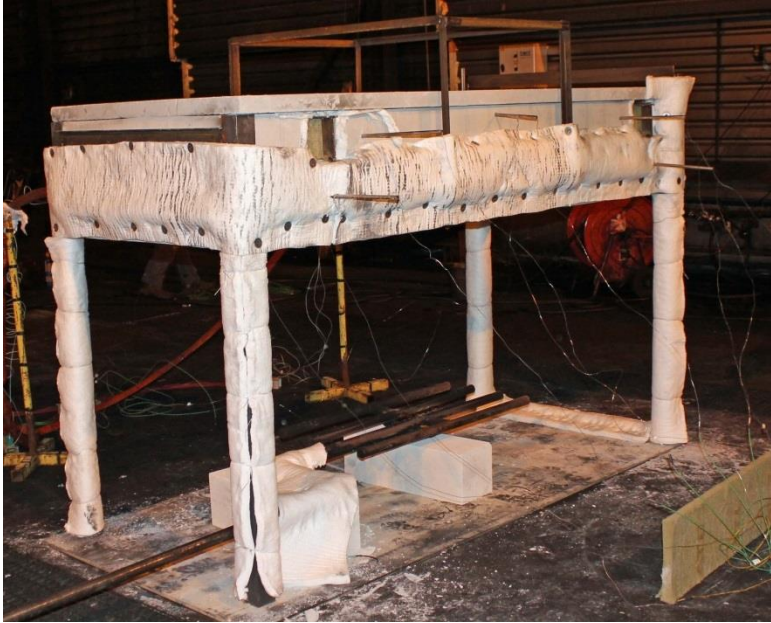
Figure 22 Test setup for testing two specimens in the ceiling jet scenario.
