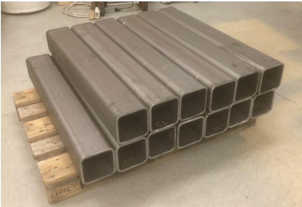
Figure 5 Test specimens for furnace and ad hoc tests before application of the protection systems. Photo; Robert Jansson McNamee.
