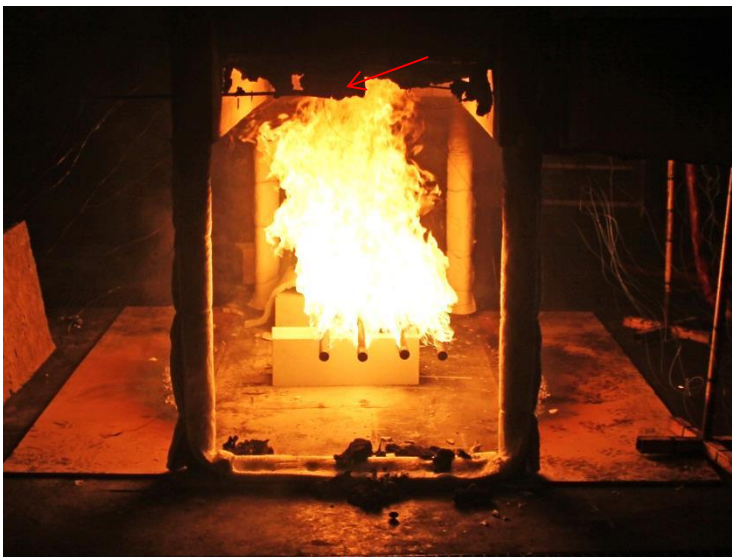
Figure 31 Release of parts of system A during ceiling jet scenario. Photo taken after the opening of the side, chunks of paint on the instrumentation 100 mm below the surface (red arrow) and on the floor.
