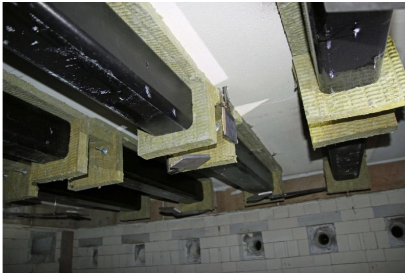
Figure 13 Test specimens during mounting in the horizontal furnace at SP Fire Research AS in Trondheim. Photo: Per Gunnar Nordløyken
