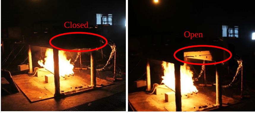
Figure 26 Opening up of the test rig after 15 minutes of exposure during the ceiling jet scenario.
