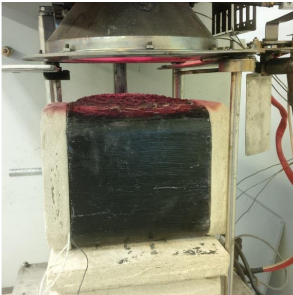
Figure 8 Test of intumescent system in cone calorimeter. The ends were insulated with stiff insulation board of 25 mm thickness. Photo: Ulla Eidissen Jensen
