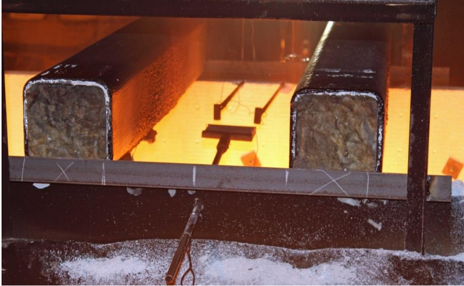
Figure 27 Fire plume scenario. Plate thermometer positioned in the centre and two differential pressure probes to estimate flow speed. An additional 1 mm shielded thermocouple was also protruding from each device. The distance between the two test specimens was 300 mm.
