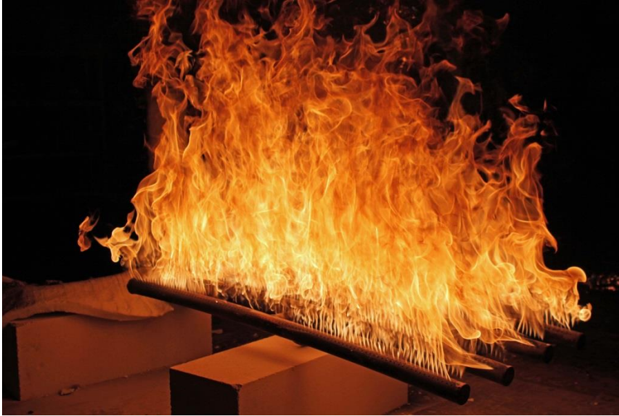
Figure 24 The fire source during ceiling jet and fire plume scenarios. Pipes slightly bent by thermal expansion.
