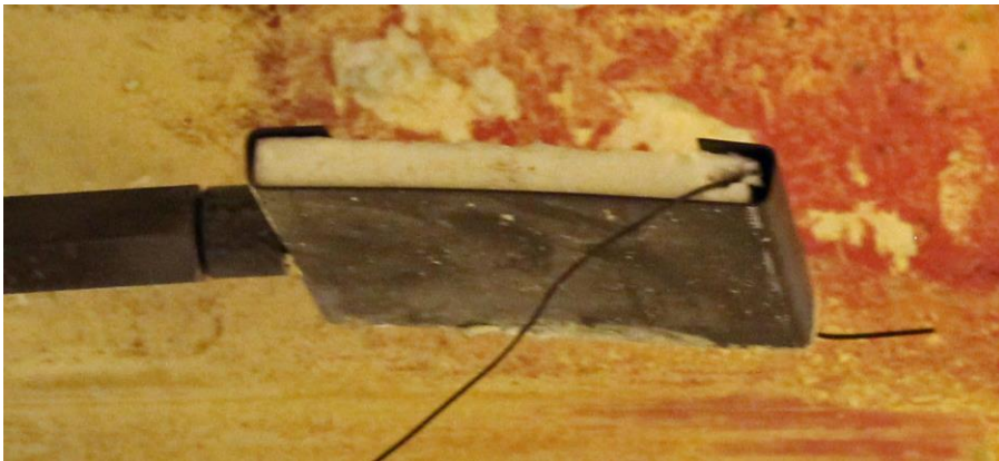
Figure 25 Plate thermometer pointing downwards, paired with a 1 mm shielded thermocouple sticking out 3 cm from the plate.
