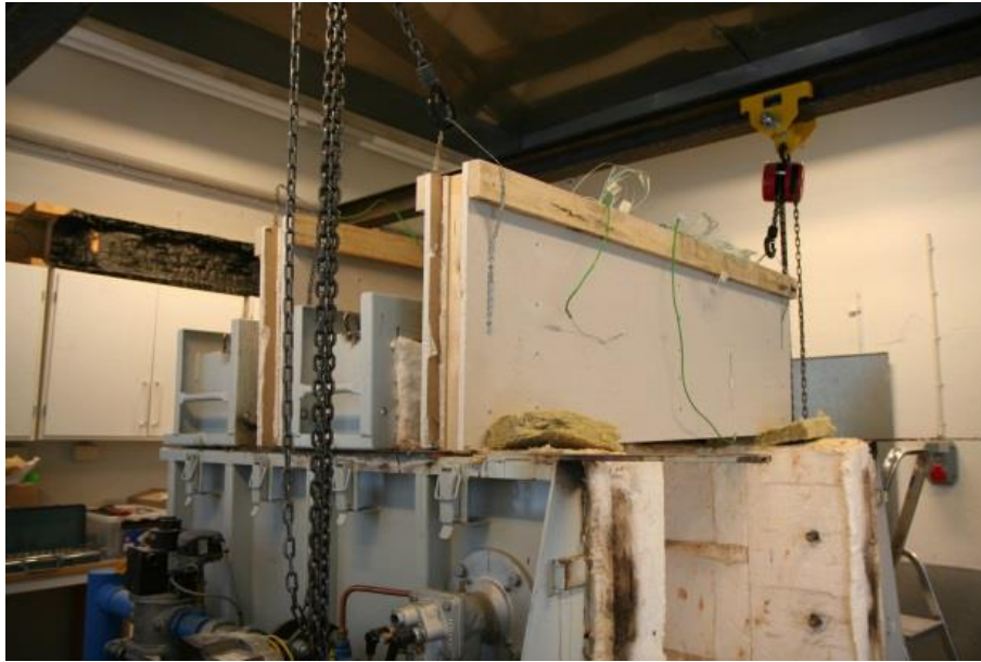
Figure 2 - Positioning of 2 specimens on top of a furnace.
