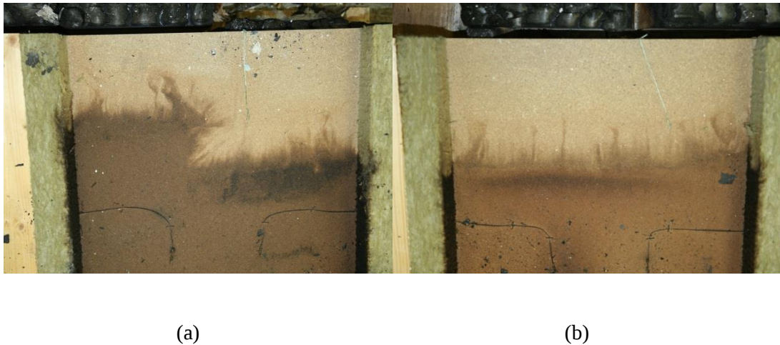
Figure 14 - Cavity walls of FSJ2.1 (a) and FSJ2.2 (b) after the test
