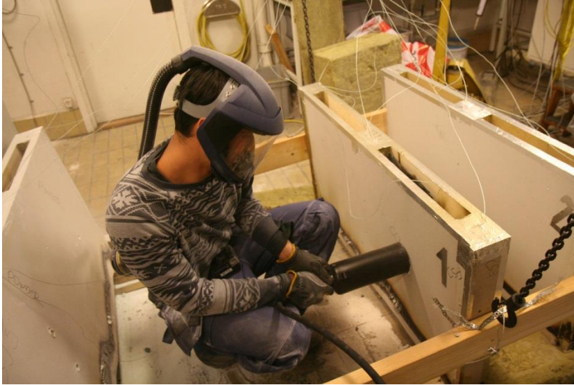
Figure 17 - Extinguishing of specimen FSJ1.
